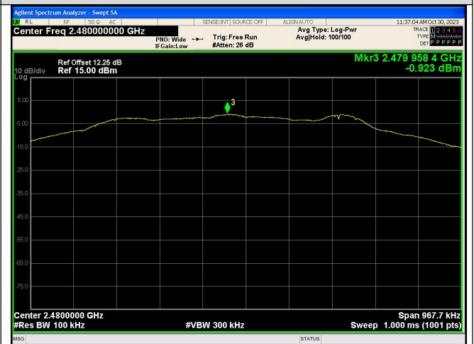
In-Band Reference Level LE_Channel 39
