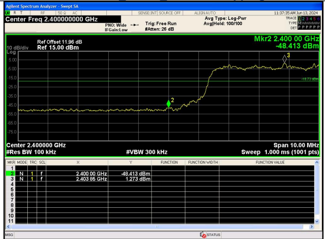
Out Of Band Emission(Left) \pi/4 DQPSK_2-DH5_Channel Hopping
