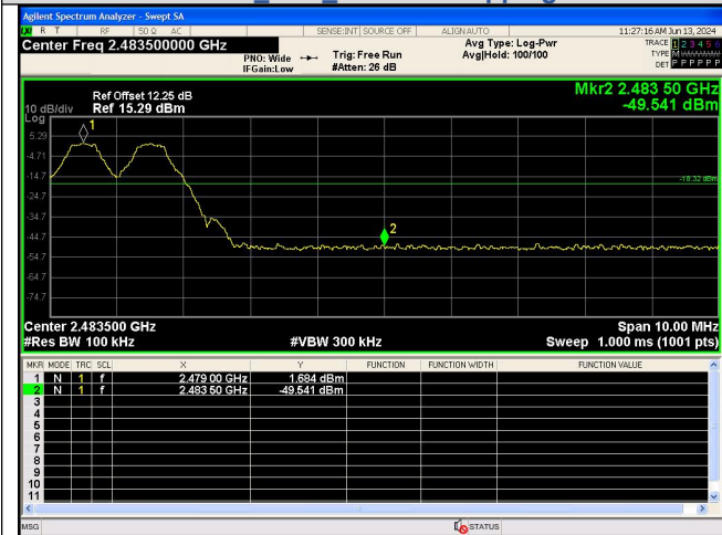
Out Of Band Emission(Right) GFSK_DH5_Channel Hopping
