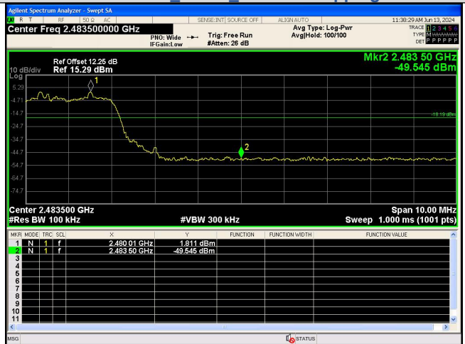
Out Of Band Emission(Right) \pi/4 DQPSK_2-DH5_Channel Hopping
