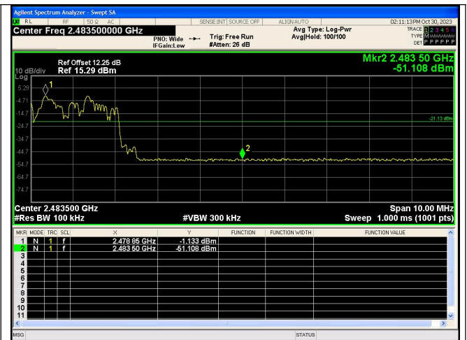
Out Of Band Emission(Right) \pi/4 DQPSK_2-DH5_Channel Hopping
