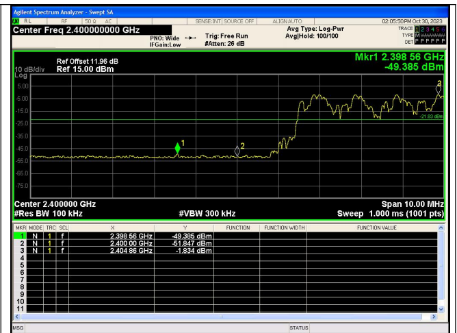
Out Of Band Emission(Left) \pi/4 DQPSK_2-DH5_Channel Hopping
