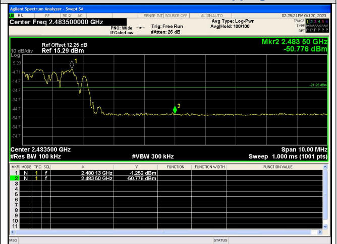
Out Of Band Emission(Right) 8DPSK_3-DH5_Channel Hopping
