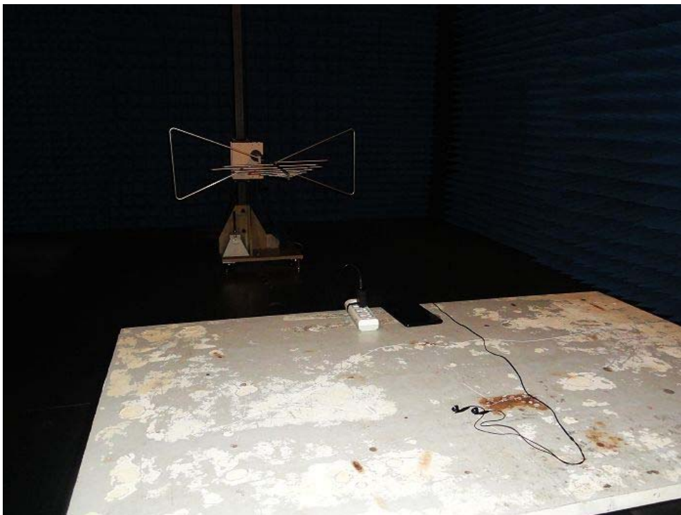
Radiated Emission Test Setup:
