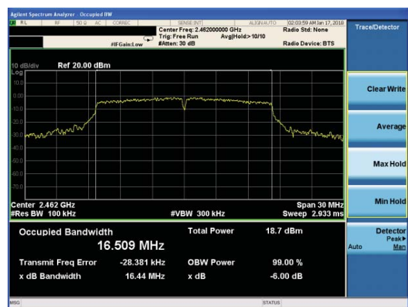
(802.11g) 6dB Bandwidth plot on channel 11
