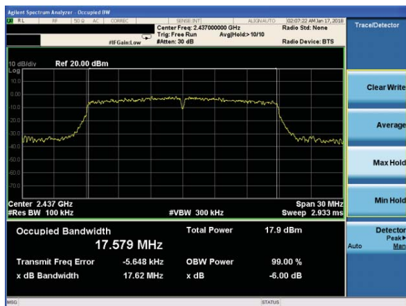
(802.11N20) 6dB Bandwidth plot on channel 11
