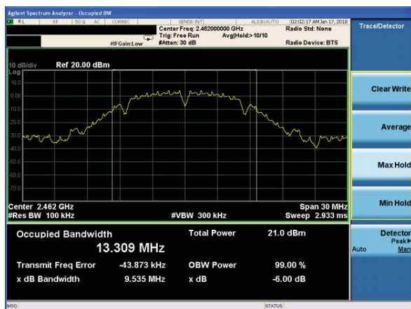
(802.11b) 6dB Bandwidth plot on channel 11
