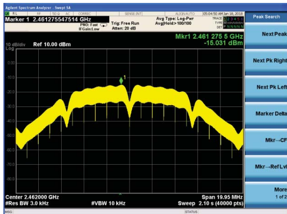
(802.11b) PSD plot on channel 11
