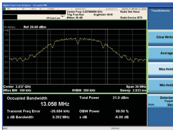
(802.11b) 6dB Bandwidth plot on channel 11
