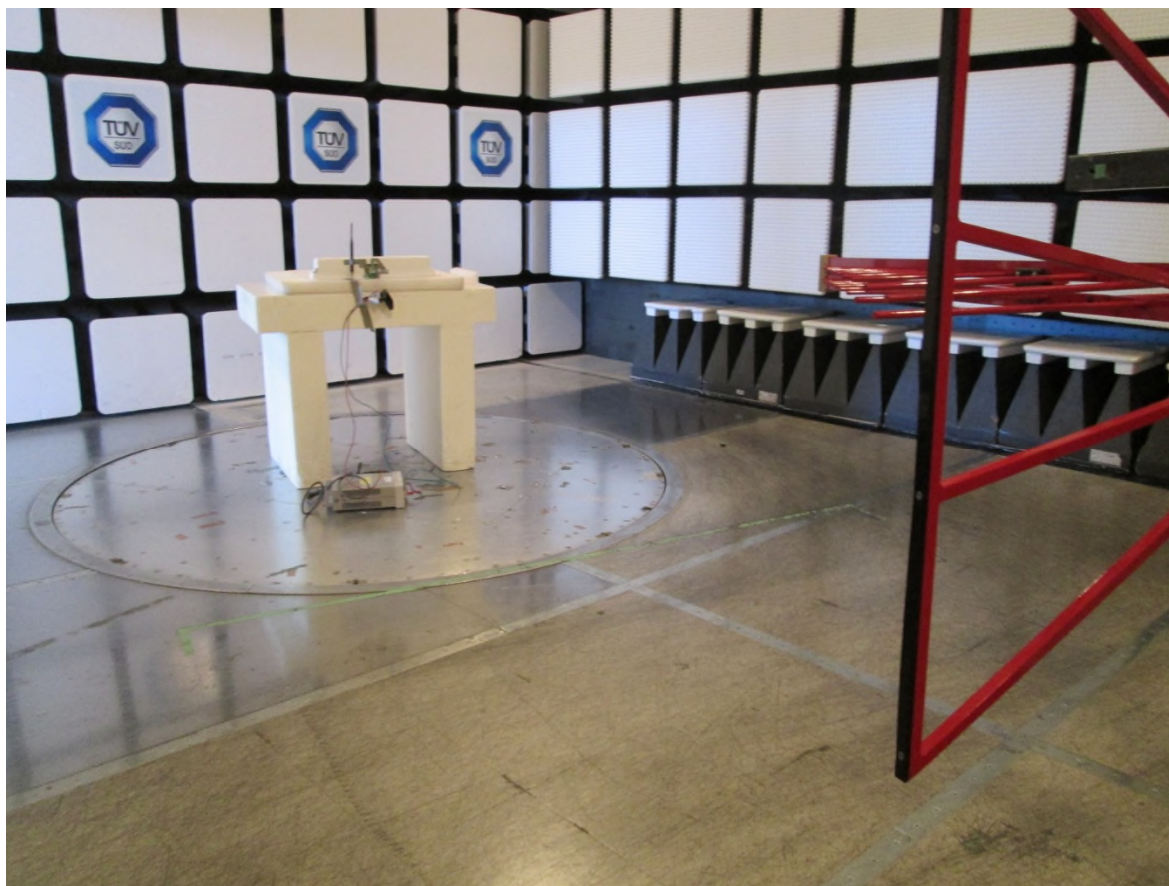
Test setup photo 2 Radiated measurements, 30 MHz – 1 GHz
