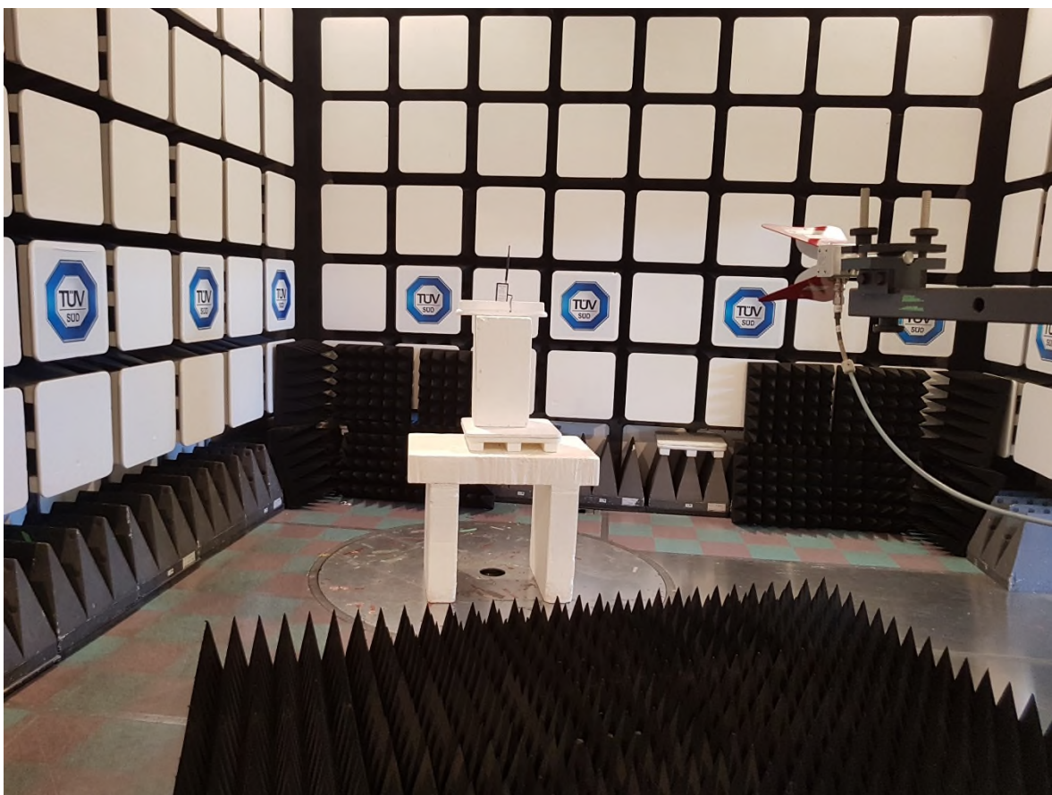
Figure 5 – Radiated Emissions Setup 1GHz to 6GHz
