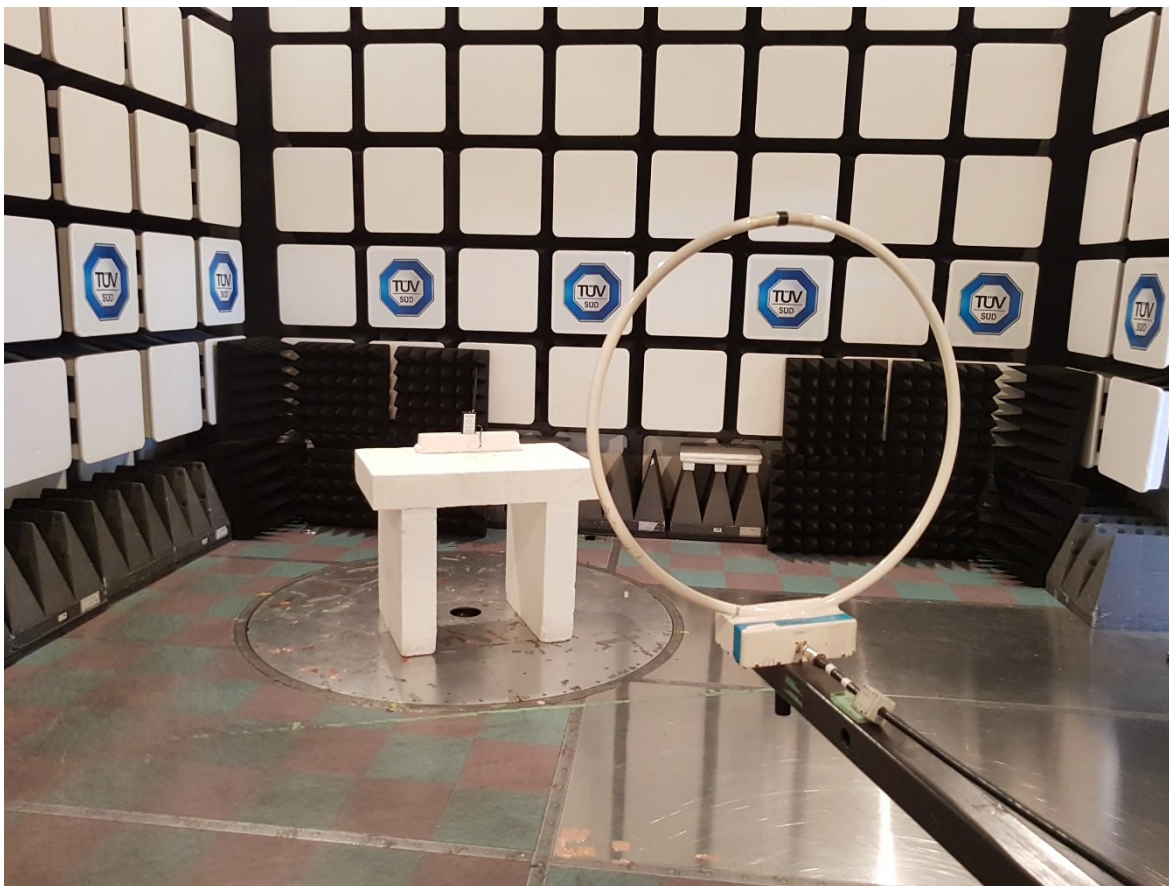
Figure 3 – Radiated Emissions Setup 9kHz to 30MHz
