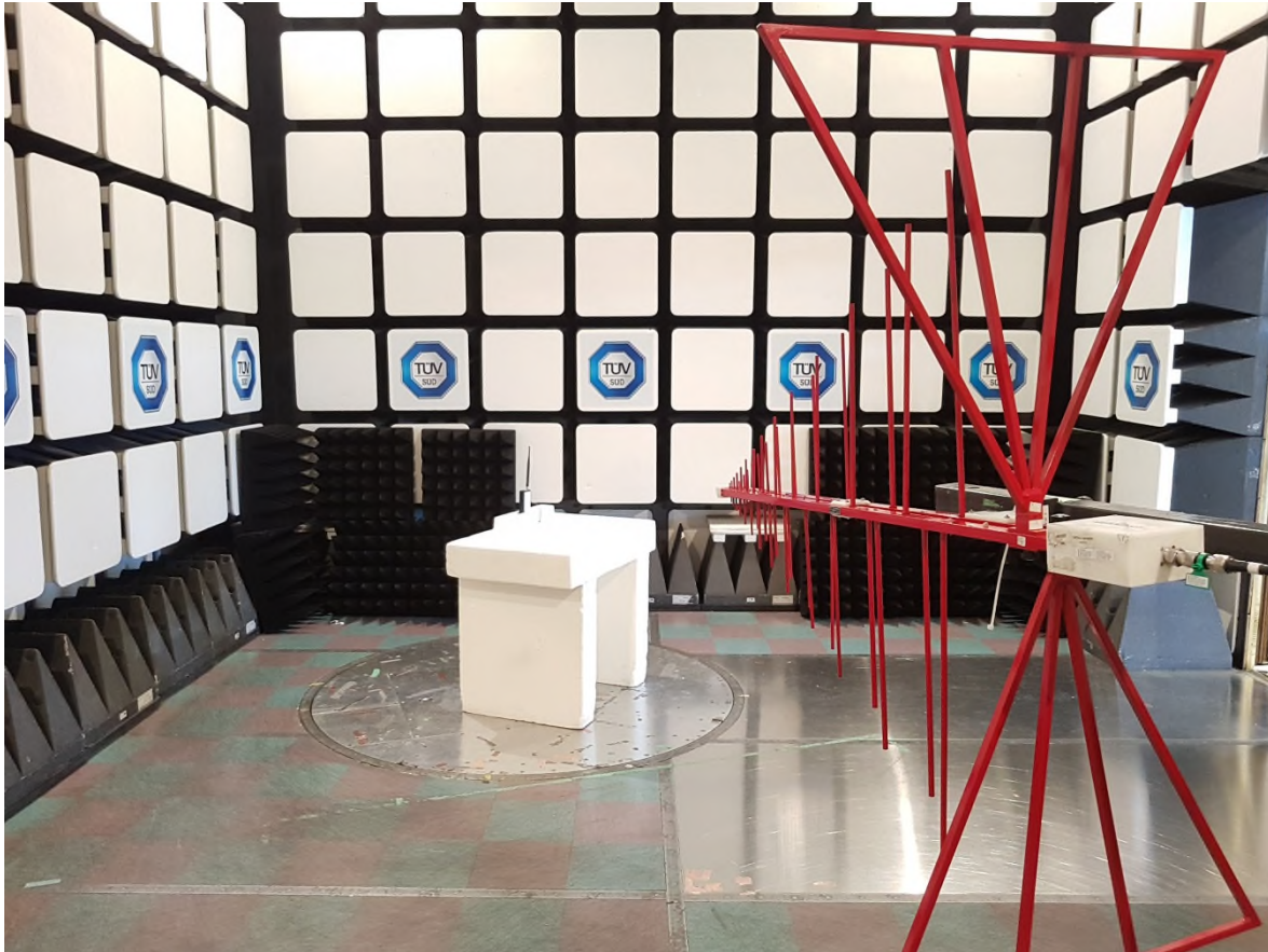
Figure 4 – Radiated Emissions Setup 30MHz to 1GHz
