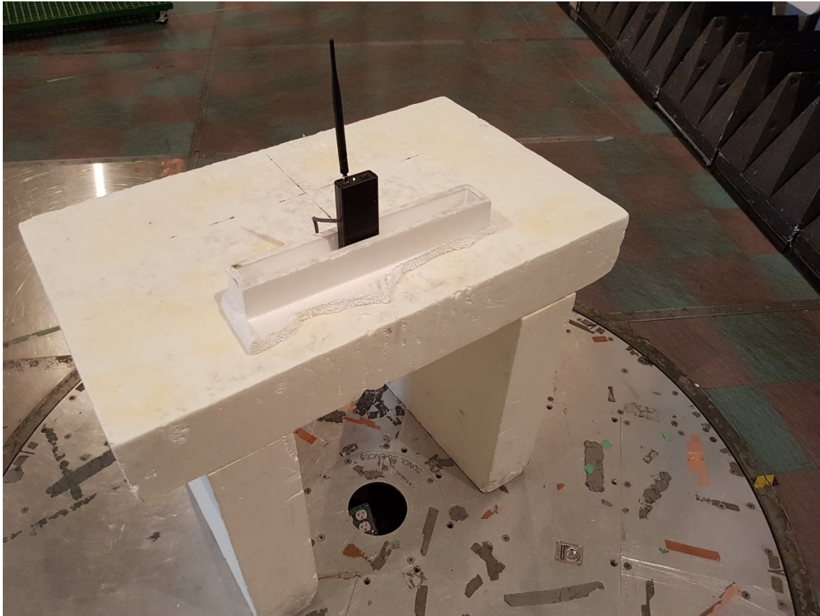
Figure 2 – Radiated Emissions Setup X-Axis
