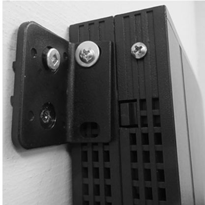
Figure 8 NC-2100K (1U model) mounted to a wall
