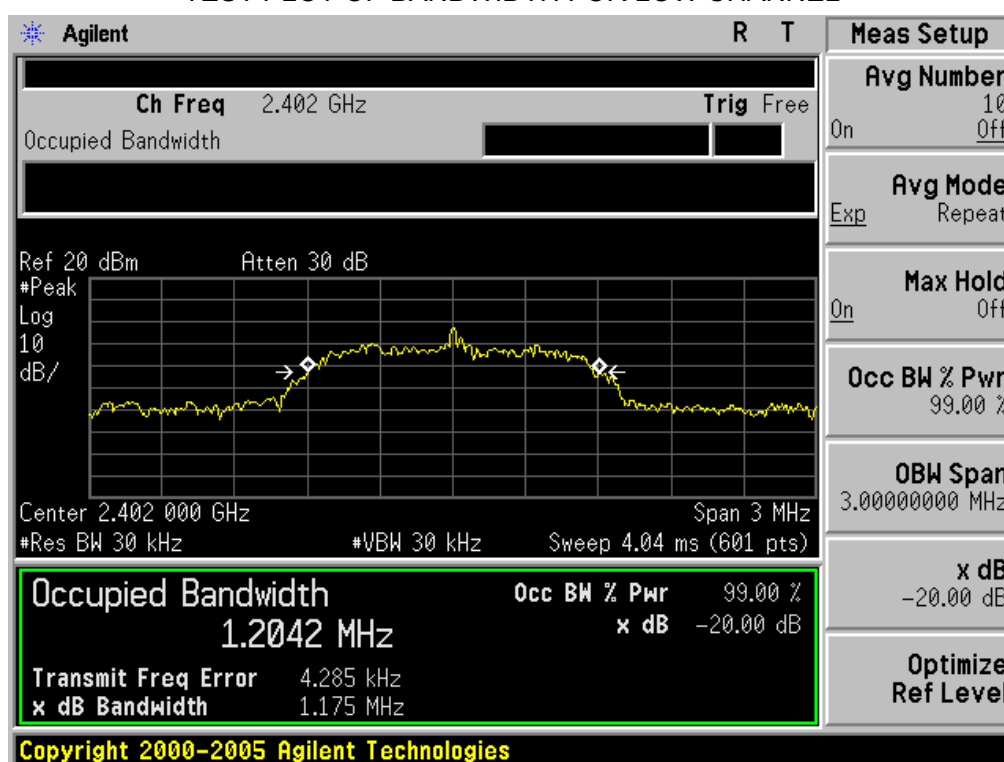
TEST PLOT OF BANDWIDTH FOR LOW CHANNEL
