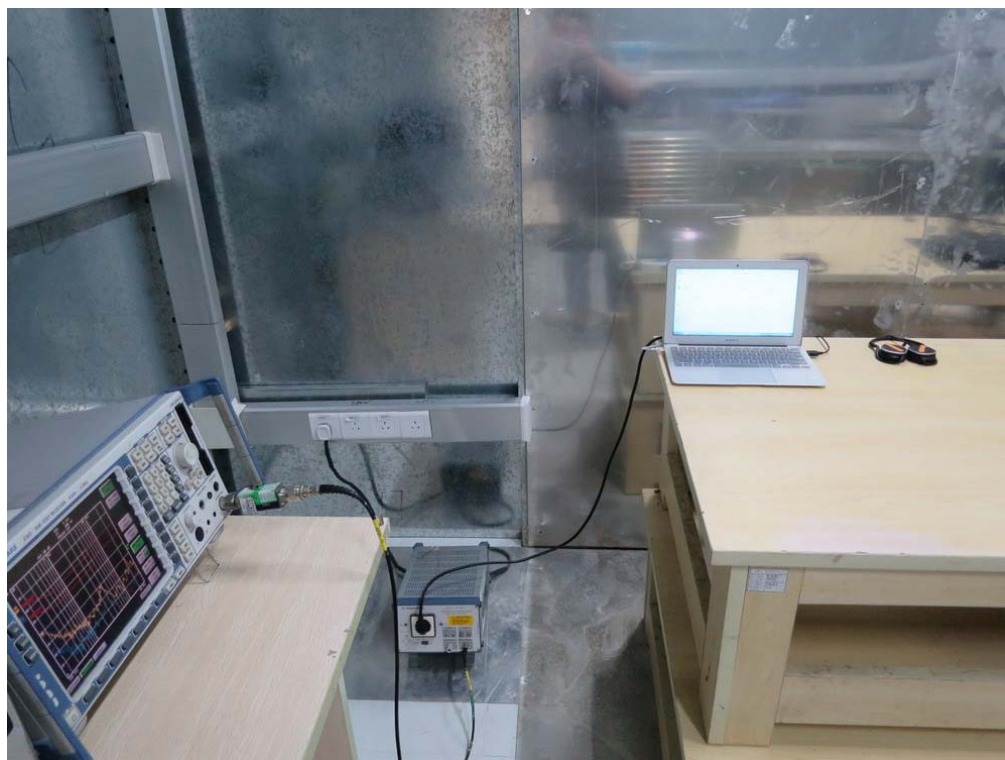
FCC RADIATED EMISSION TEST SETUP
