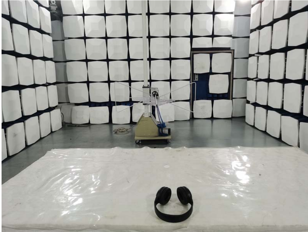
Radiated Emission Test Setup:
