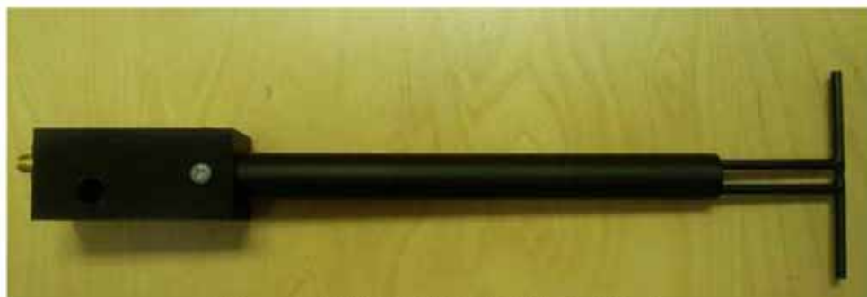
Figure 1 – MVG COMOSAR Validation Dipole
