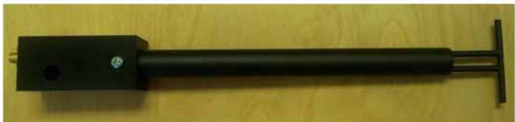
Figure 1 – MVG COMOSAR Validation Dipole
