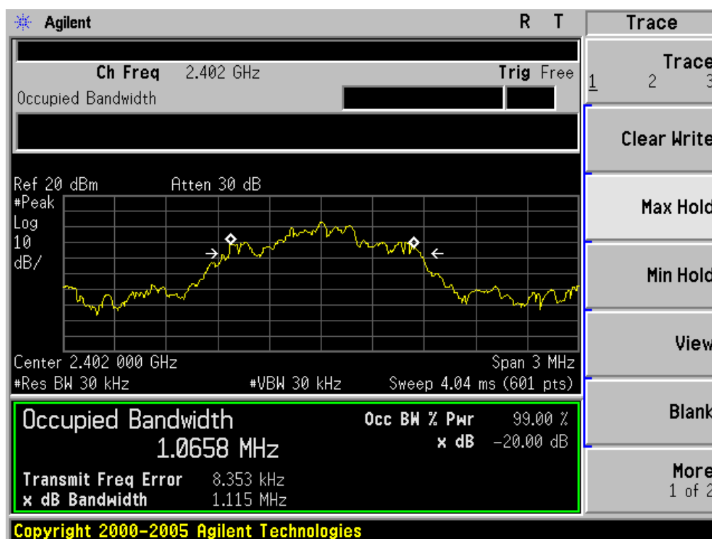
TEST PLOT OF BANDWIDTH FOR LOW CHANNEL
