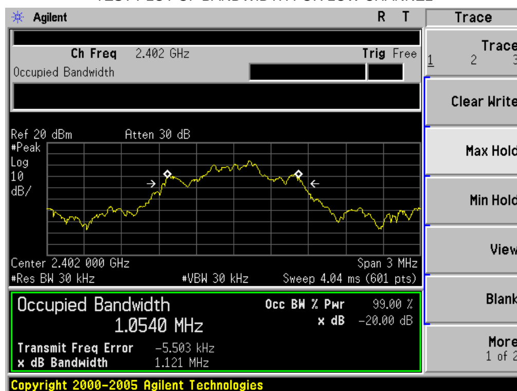
TEST PLOT OF BANDWIDTH FOR LOW CHANNEL
