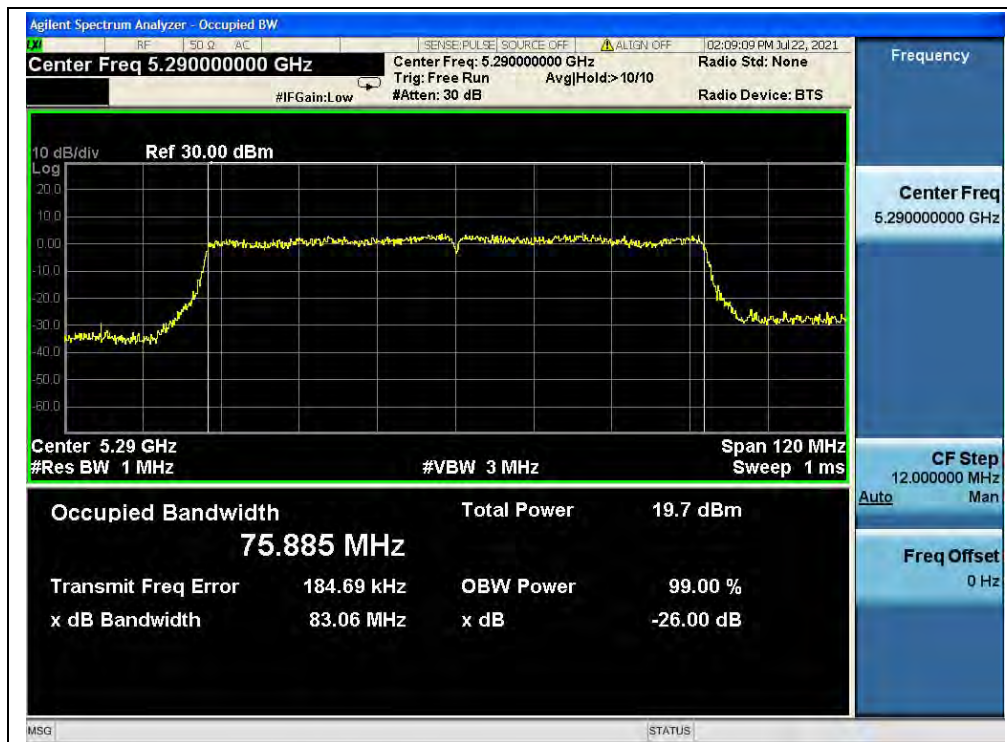
(Channel 58, 5290MHz, 802.11ac (VHT80))
