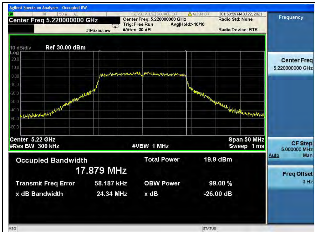
(Channel 44, 5220MHz, 802.11ac (VHT20))
