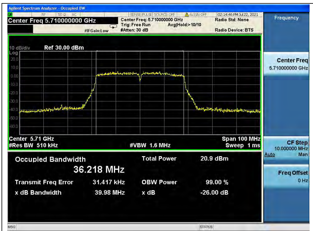
(Channel 142, 5710MHz, 802.11ac (VHT40))
