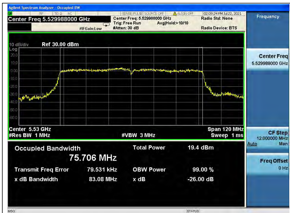
(Channel 106, 5530MHz, 802.11ac (VHT80))
