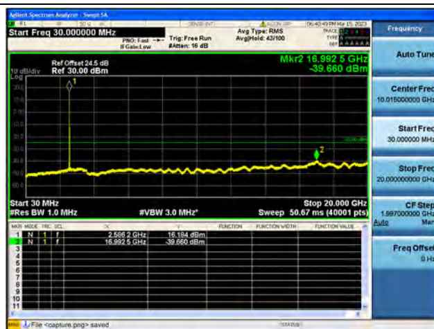
Band41-30M-20G / 15MHz / Mid CH / 64QAM
