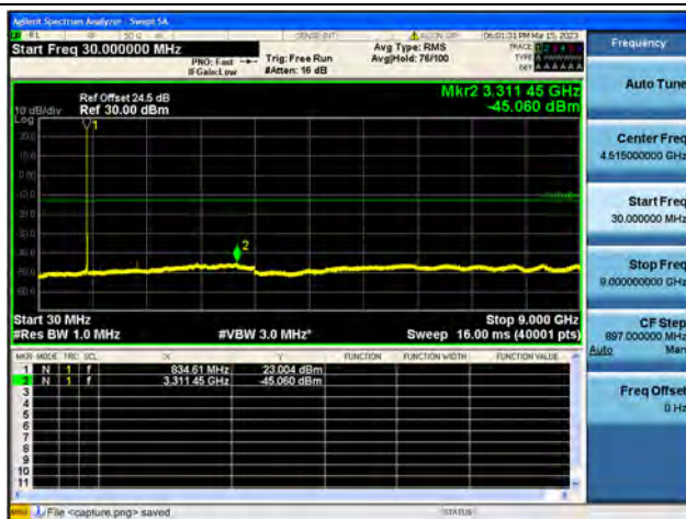
Band26 Part22 / 5MHz / Mid CH / 16QAM
