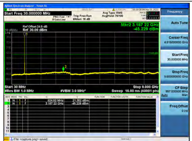
Band26 Part22 / 3MHz / Low CH / 64QAM
