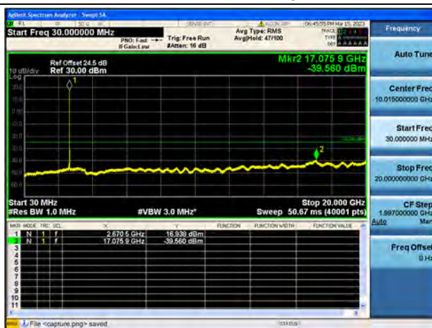
Band41-30M-20G / 20MHz / High CH / 64QAM
