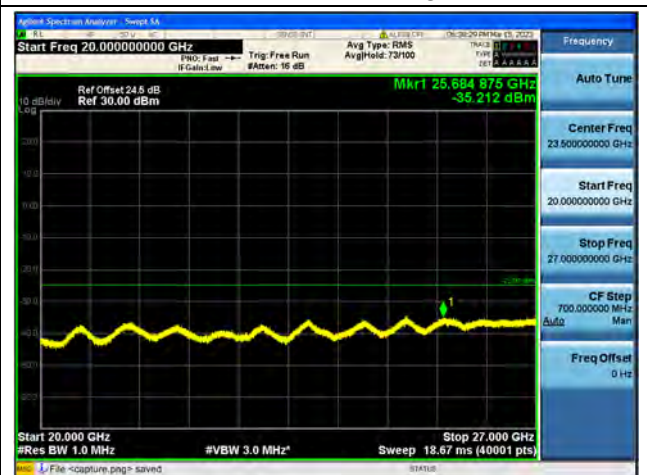
Band41-20G-27G / 10MHz / High CH / 64QAM
