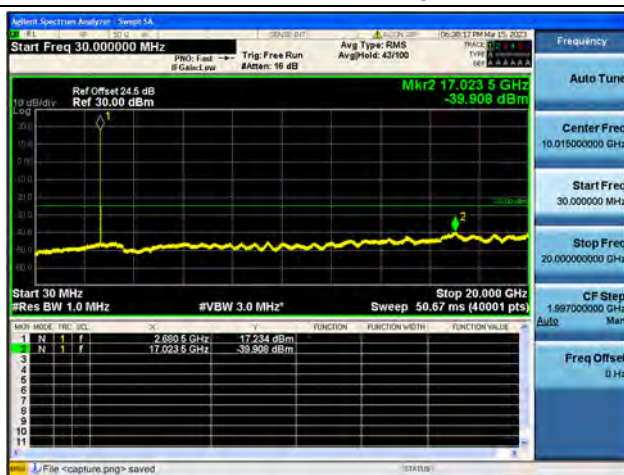
Band41-30M-20G / 10MHz / High CH / 64QAM
