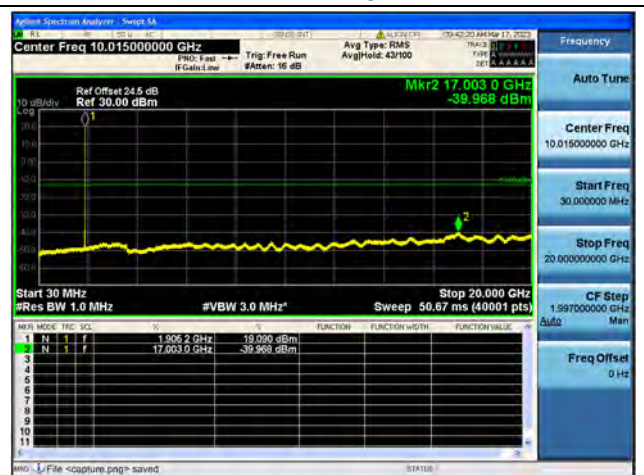
Band25 / 10MHz / High CH / 64QAM
