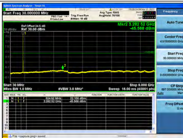
Band26 Part22 / 3MHz / Low CH / 16QAM
