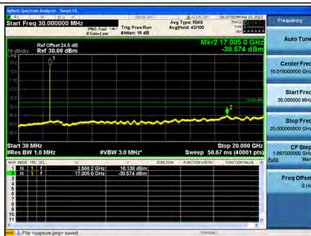
Band41-30M-20G / 10MHz / Mid CH / 64QAM
