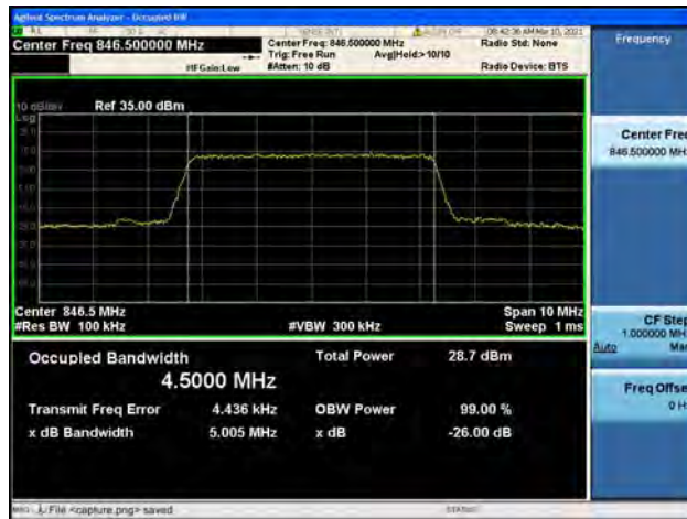
Band5 / 5MHz / High CH / 64QAM
