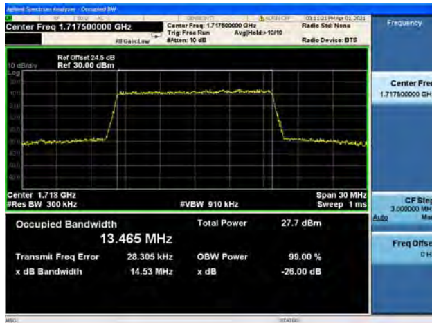
Band66 / 15MHz / Mid CH / 16QAM
