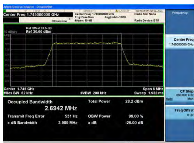
Band66 / 3MHz / High CH / 16QAM
