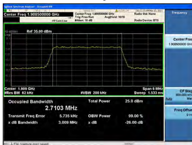
Band2 / 3MHz / High CH / 64QAM
