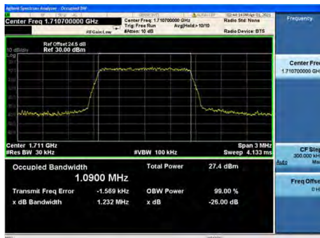
Band66 / 1.4MHz / Mid CH / 16QAM
