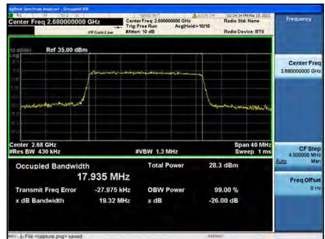
Band41 / 20MHz / High CH / 16QAM
