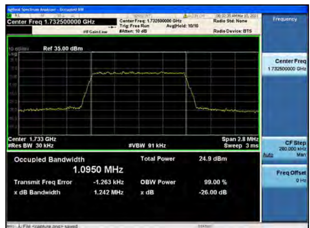
Band4 / 1.4MHz / Mid CH / 64QAM
