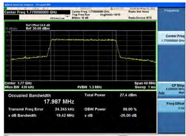
Band66 / 20MHz / High CH / 64QAM
