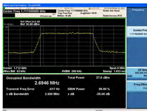
Band66 / 3MHz / Low CH / 64QAM
