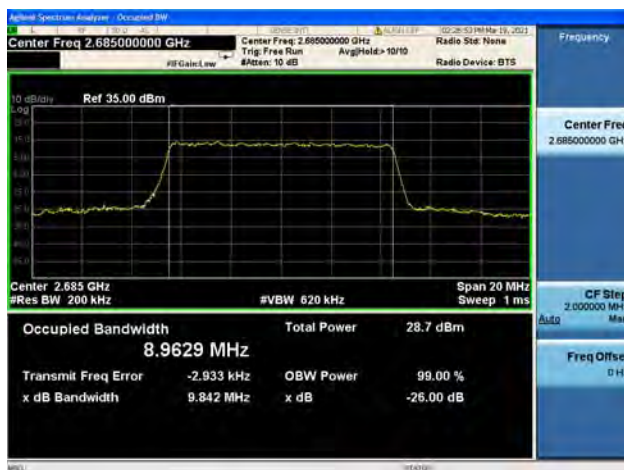
Band41 / 10MHz / High CH / 64QAM
