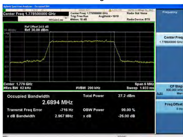
Band66 / 3MHz / High CH / 16QAM
