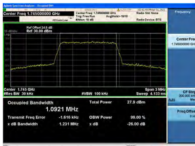
Band66 / 1.4MHz / Mid CH / 16QAM
