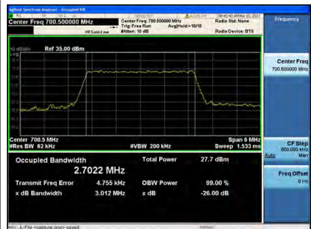
Band12 / 3MHz / Low CH / 64QAM
