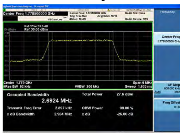
Band66 / 3MHz / High CH / 64QAM
