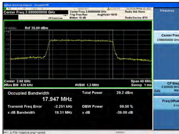
Band41 / 20MHz / High CH / 64QAM
