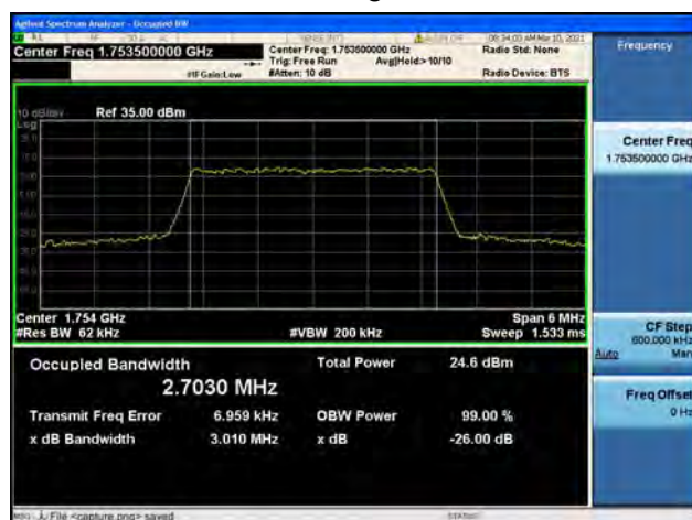
Band4 / 3MHz / High CH / 16QAM
