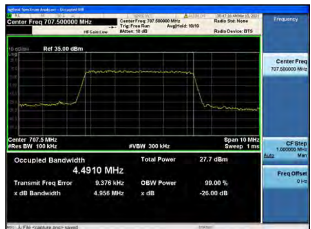
Band12 / 5MHz / Mid CH / 64QAM
