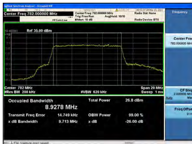
Band13 / 10MHz / High CH / 16QAM
