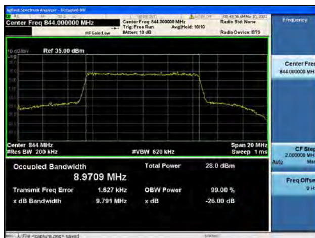
Band5 / 10MHz / High CH / 16QAM
