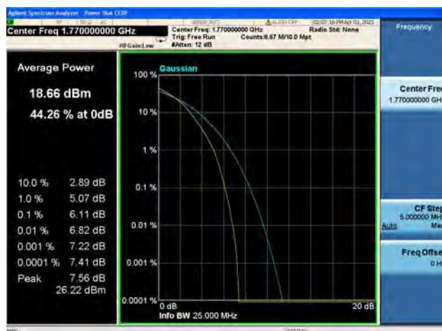
Band66 / 20MHz / High CH / 16QAM
