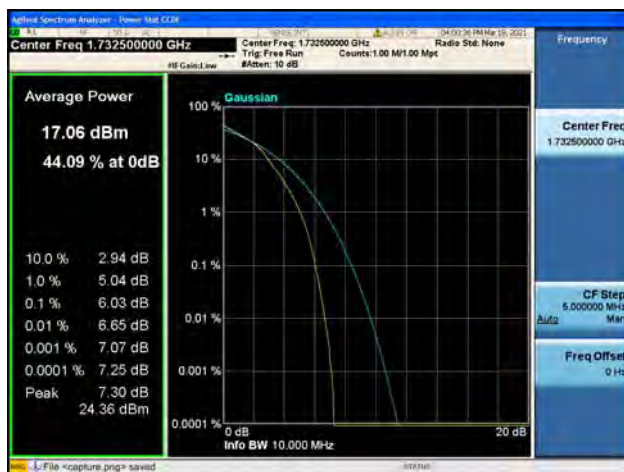
Band4 / 10MHz / High CH / 16QAM
