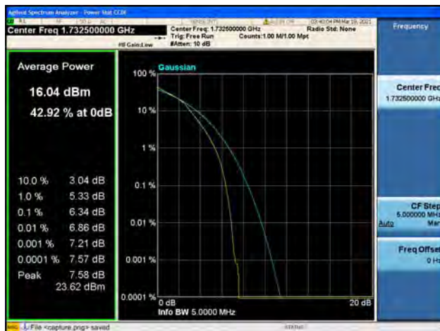
Band4 / 3MHz / High CH / 16QAM
