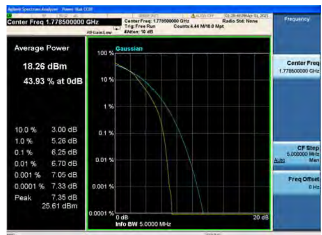
Band66 / 3MHz / High CH / 64QAM
