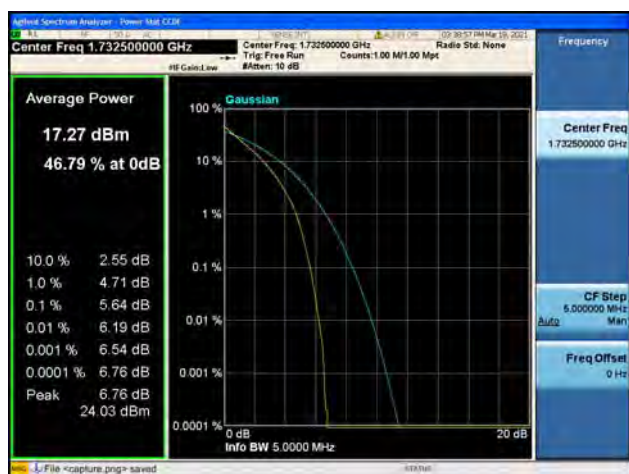
Band4 / 1.4MHz / Mid CH / 64QAM
