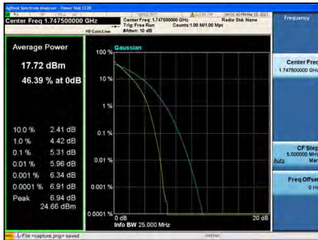
Band4 / 15MHz / High CH / 64QAM
