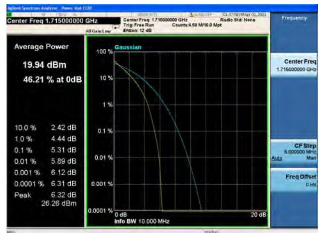
Band66 / 10MHz / Low CH / 64QAM
