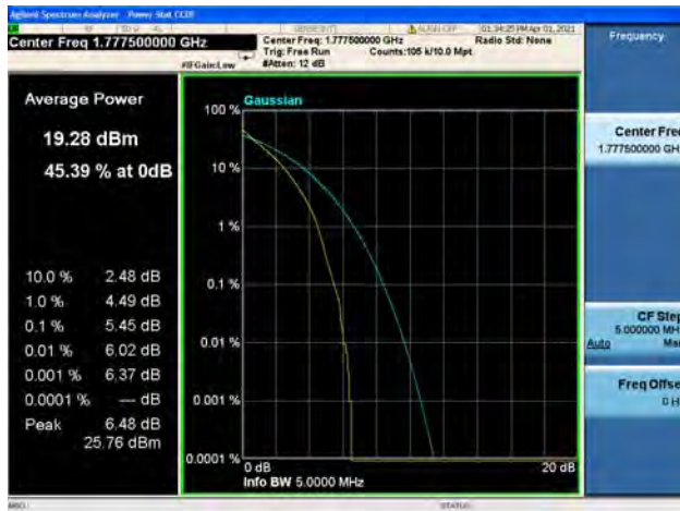
Band66 / 5MHz / High CH / 64QAM
