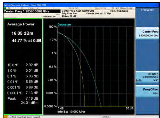
Band2 / 10MHz / High CH / 64QAM
