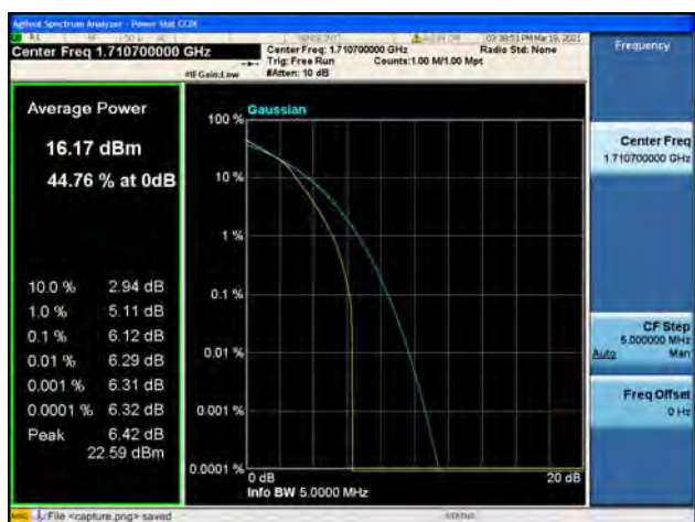
Band4 / 1.4MHz / Mid CH / 16QAM
