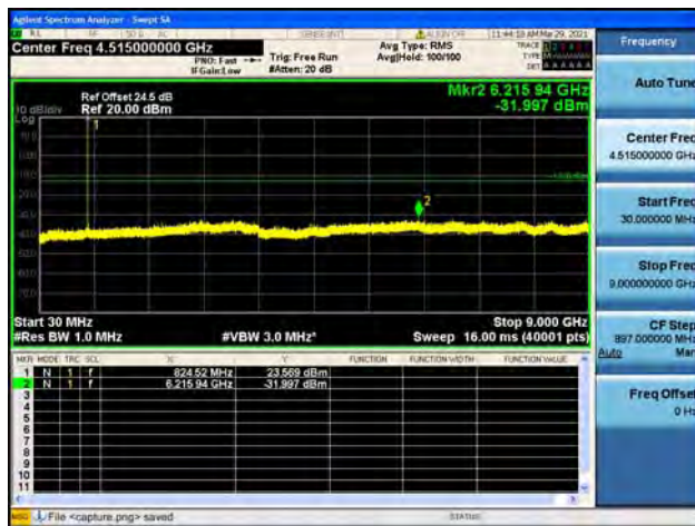
Band5 / 1.4MHz / Mid CH / 16QAM
