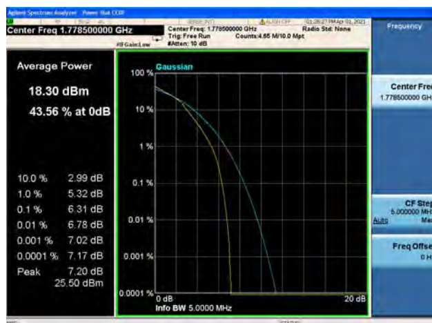
Band66 / 3MHz / High CH / 16QAM
