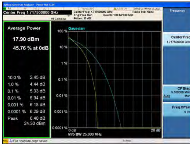
Band4 / 15MHz / Low CH / 64QAM
