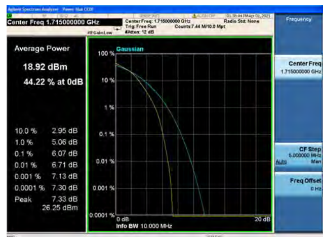
Band66 / 10MHz / Low CH / 64QAM
