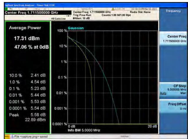
Band4 / 3MHz / Low CH / 64QAM
