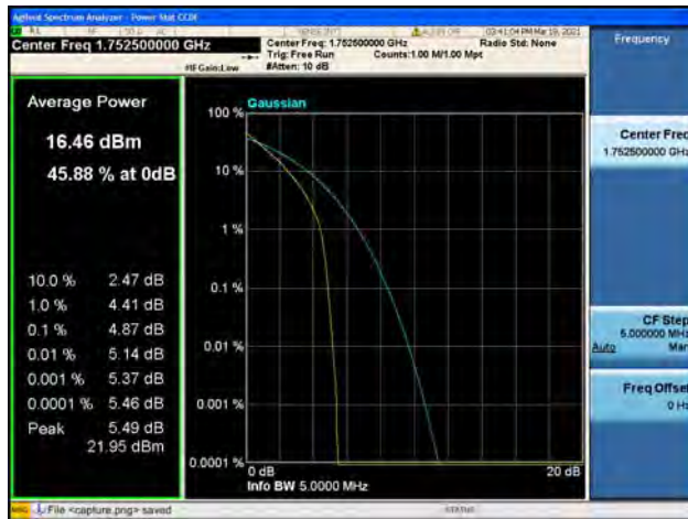
Band4 / 5MHz / High CH / 64QAM
