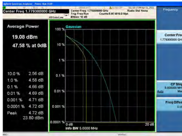
Band66 / 1.4MHz / High CH / 64QAM
