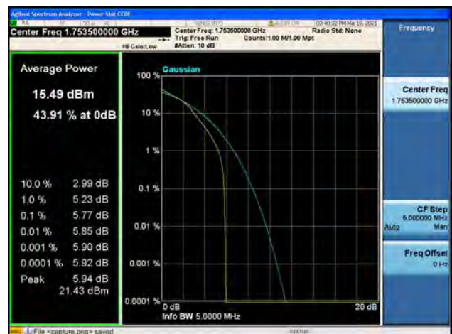
Band4 / 3MHz / High CH / 64QAM
