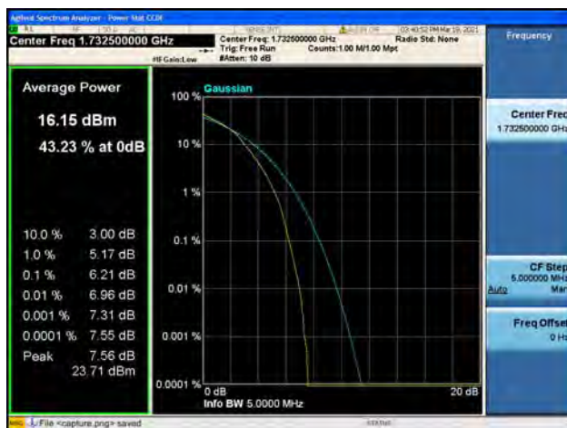
Band4 / 5MHz / Mid CH / 16QAM
