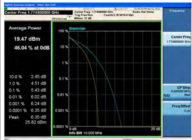
Band66 / 10MHz / High CH / 64QAM
