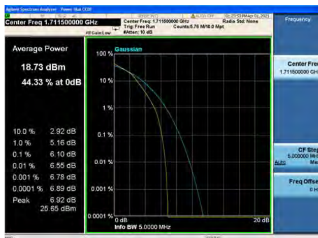
Band66 / 3MHz / Low CH / 16QAM
