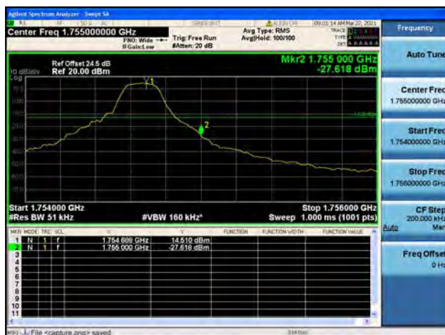
Band4 / 5MHz / High CH / QPSK / 1 RB
