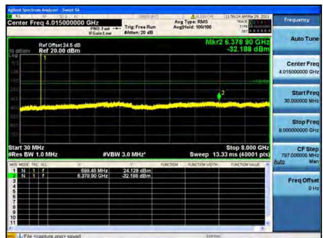
Band12 / 3MHz / Low CH / 64QAM
