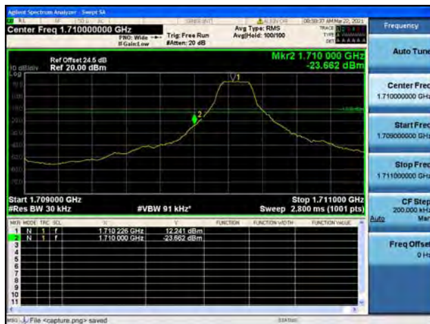
Band4 / 3MHz / Low CH / QPSK / 1 RB
