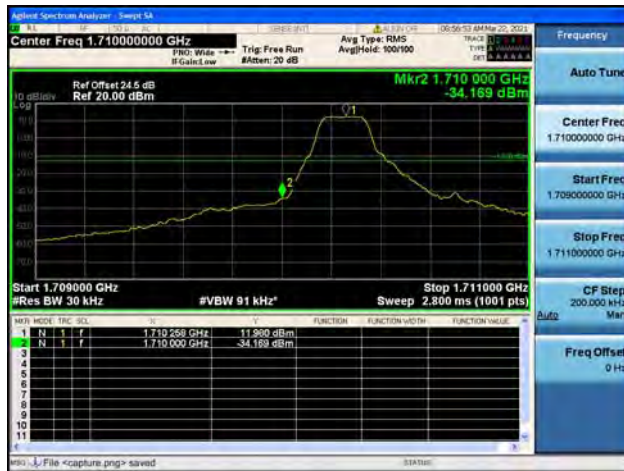
Band4 / 1.4MHz / High CH / QPSK / 1 RB
