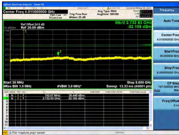
Band13 / 5MHz / High CH / 64QAM
