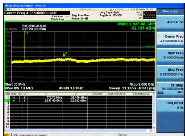
Band13 / 10MHz / High CH / 64QAM
