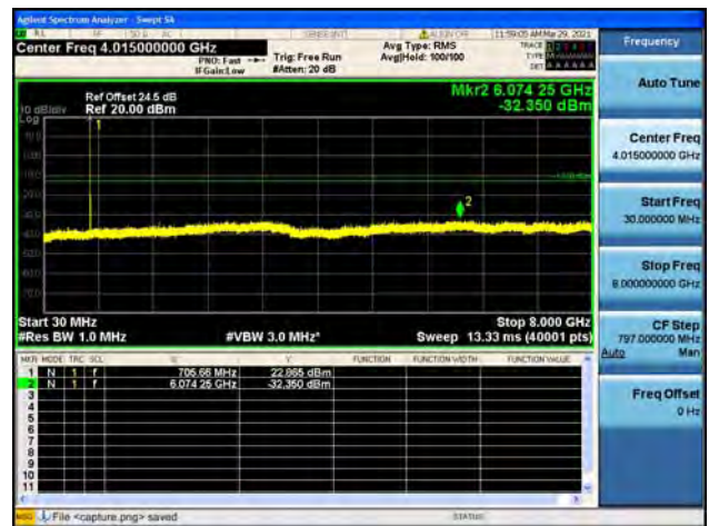
Band12 / 5MHz / Mid CH / 64QAM
