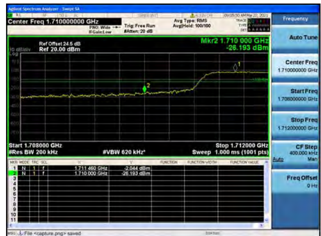
Band4 / 20MHz / High CH / QPSK / FULL RB
