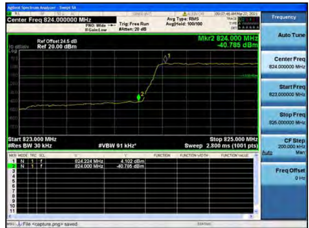
Band5 / 1.4MHz / High CH / QPSK / FULL RB
