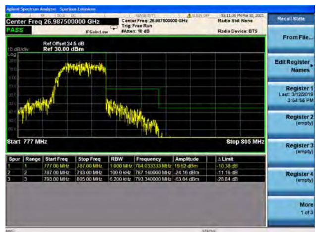
Band13 / 5MHz / High CH / QPSK / FULL RB
