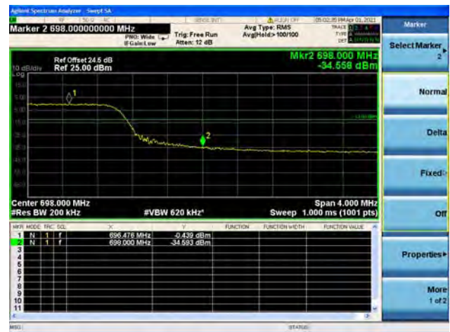
Band71 / 20MHz / High CH / QPSK / FULL RB
