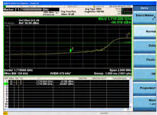
Band66 / 15MHz / High CH / QPSK / FULL RB
