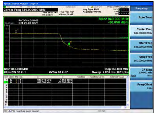
Band5 / 5MHz / Low CH / QPSK / FULL RB
