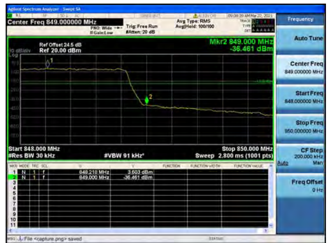
Band5 / 3MHz / Low CH / QPSK / FULL RB
