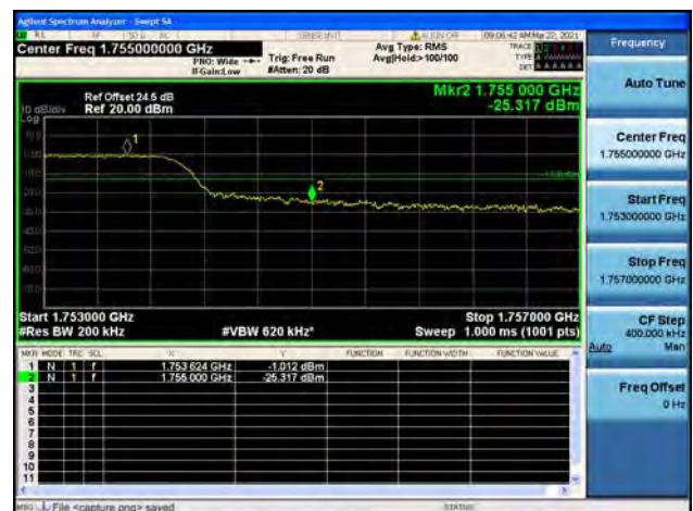
Band4 / 20MHz / High CH / QPSK / FULL RB
