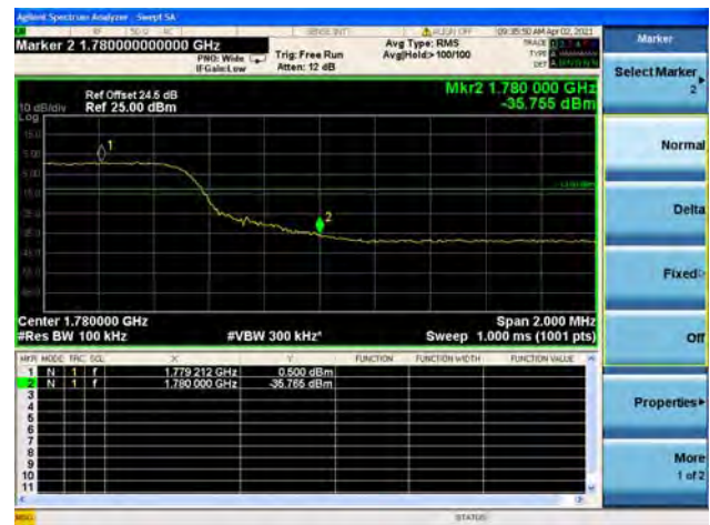
Band66 / 10MHz / High CH / QPSK / FULL RB
