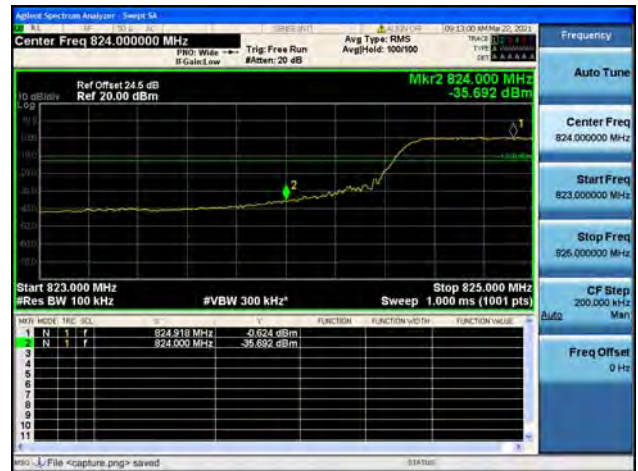
Band5 / 10MHz / High CH / QPSK / FULL RB
