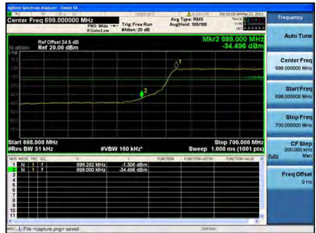
Band12 / 5MHz / High CH / QPSK / FULL RB
