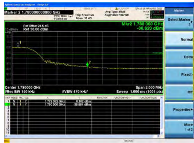
Band66 / 15MHz / High CH / QPSK / FULL RB
