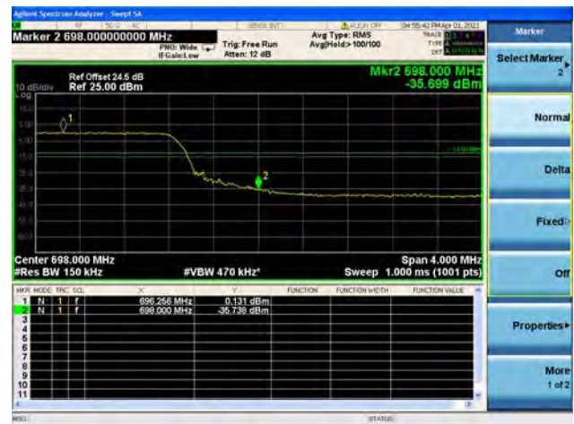
Band71 / 15MHz / High CH / QPSK / FULL RB
