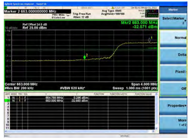
Band71 / 20MHz / High CH / QPSK / FULL RB
