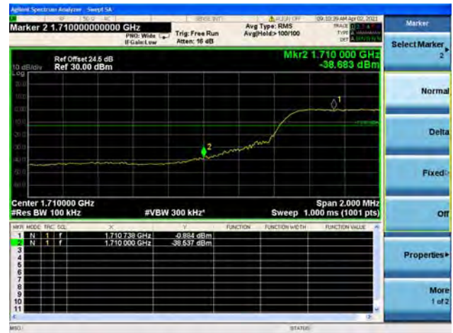
Band66 / 10MHz / High CH / QPSK / FULL RB
