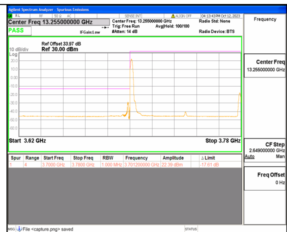
5A_n77(3700-3980MHz) 80M DFT-s-OFDM QPSK Edge_1RB_Left Low
