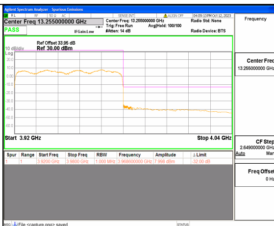
5A_n77(3700-3980MHz) 60M DFT-s-OFDM QPSK Outer_Full High
