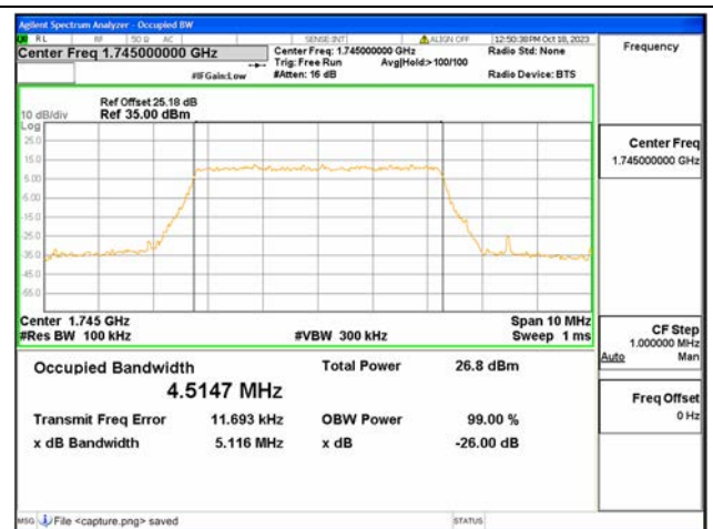
B66 / 5MHz / 256QAM/ Mid CH
