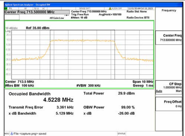
B12 / 5MHz / 16QAM/ High CH
