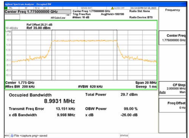
B66 / 10MHz / 16QAM/ High CH
