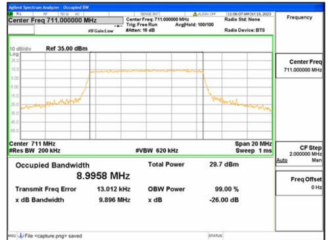
B12 / 10MHz / 16QAM/ High CH
