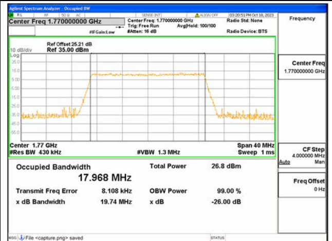
B66 / 20MHz / 256QAM/ High CH
