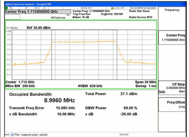
B66 / 10MHz / 256QAM/ Low CH
