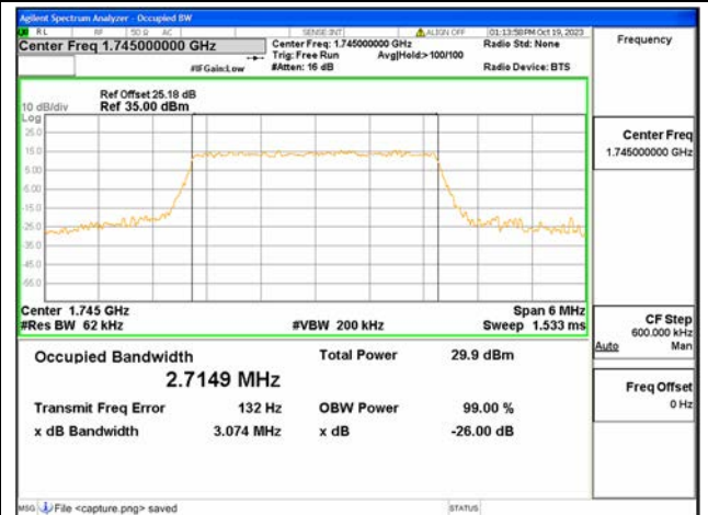
B66 / 3MHz / 16QAM/ Mid CH
