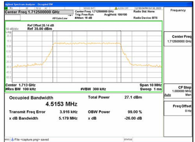
B66 / 5MHz / 256QAM/ Low CH
