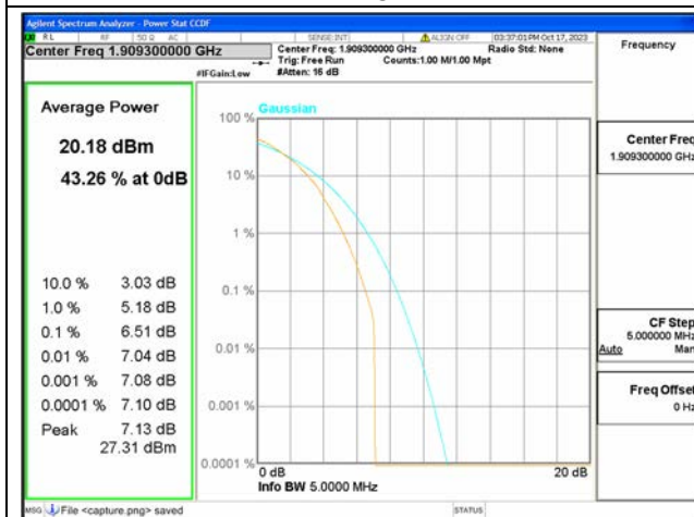
B2 / 1.4MHz / High CH / 64QAM
