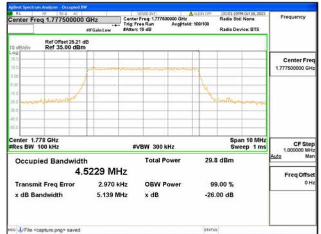
B66 / 5MHz / 16QAM/ High CH
