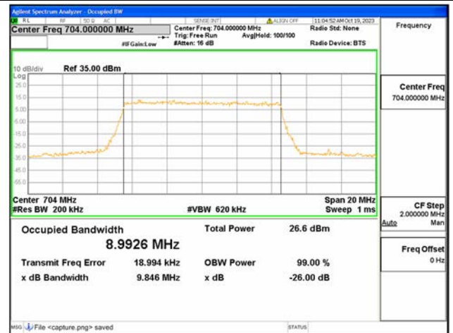
B12 / 10MHz / 256QAM/ Low CH
