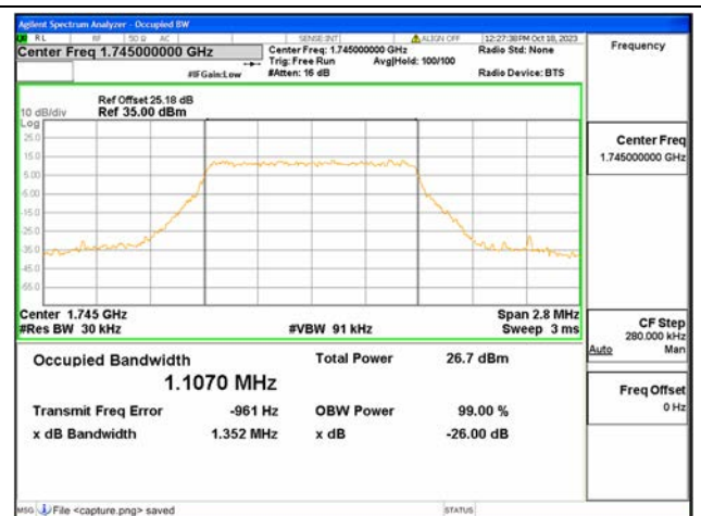
B66 / 1.4MHz / 256QAM/ Mid CH
