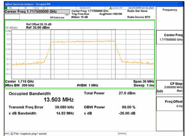
B66 / 15MHz / 256QAM/ Low CH
