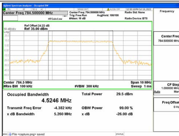
B13 / 5MHz / 64QAM/ High CH
