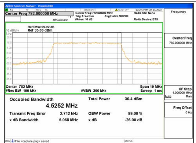
B13 / 5MHz / 16QAM/ Mid CH
