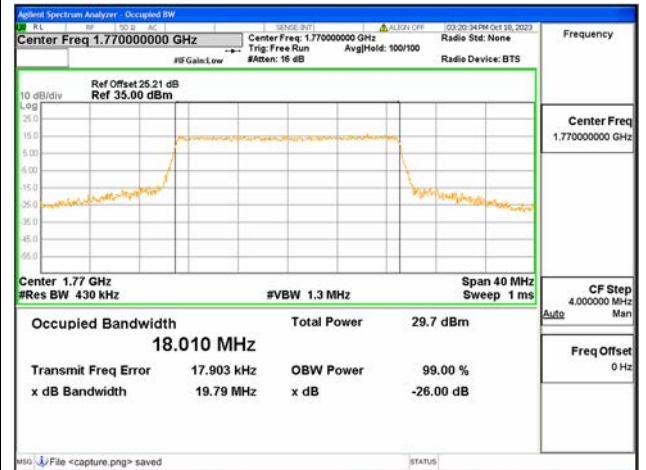
B66 / 20MHz / 16QAM/ High CH
