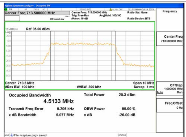
B12 / 5MHz / 256QAM/ High CH
