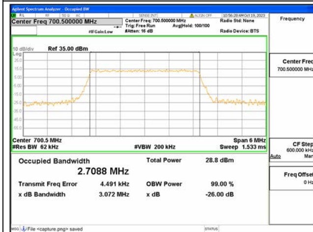
B12 / 3MHz / 64QAM/ Low CH
