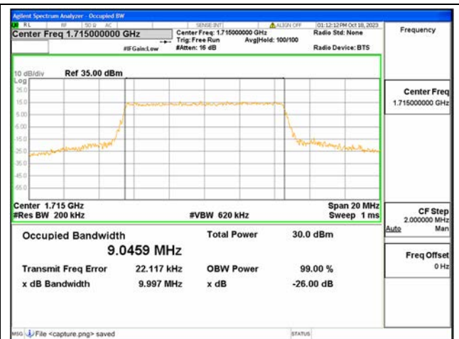
B66 / 10MHz / 16QAM/ Low CH
