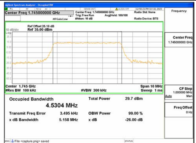
B66 / 5MHz / 16QAM/ Mid CH
