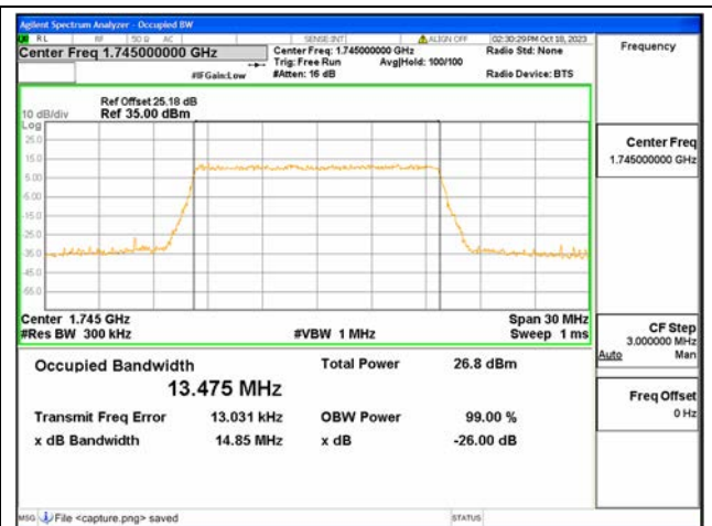
B66 / 15MHz / 256QAM/ Mid CH
