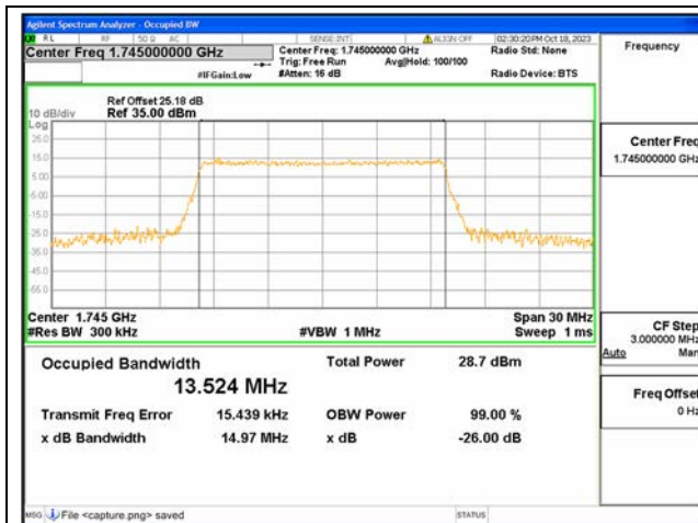
B66 / 15MHz / 64QAM/ Mid CH
