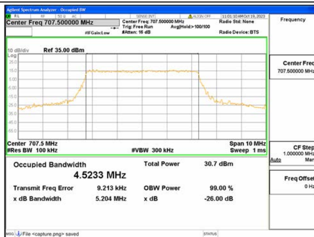
B12 / 5MHz / QPSK/ Mid CH
