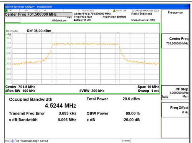
B12 / 5MHz / 16QAM/ Low CH
