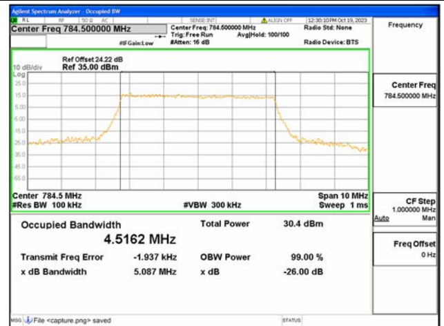
B13 / 5MHz / 16QAM/ High CH
