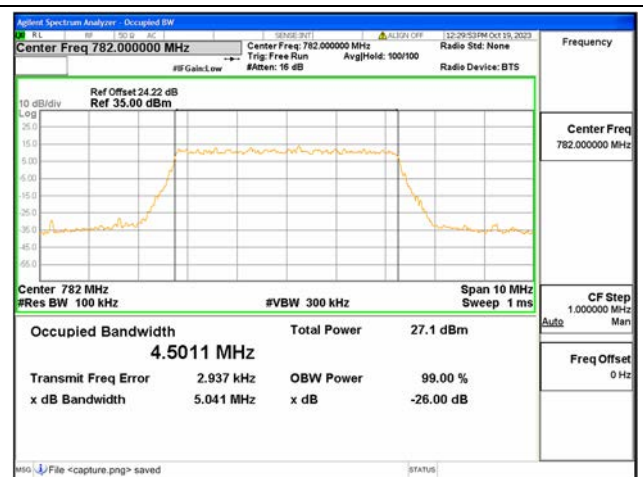
B13 / 5MHz / 256QAM/ Mid CH
