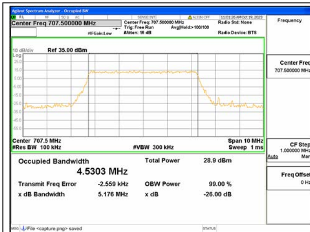
B12 / 5MHz / 64QAM/ Mid CH
