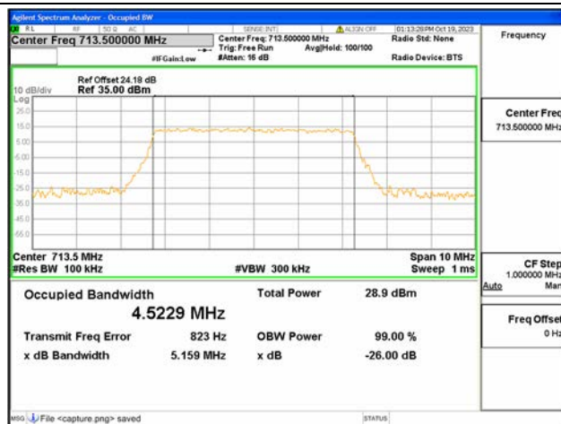
B12 / 5MHz / 64QAM/ High CH
