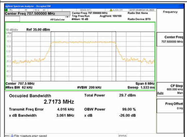
B12 / 3MHz / 16QAM/ Mid CH
