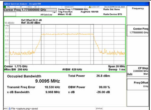
B66 / 10MHz / 256QAM/ High CH
