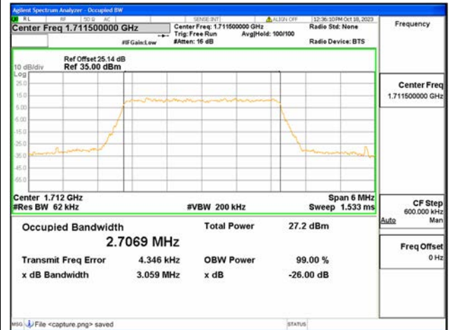
B66 / 3MHz / 256QAM/ Low CH
