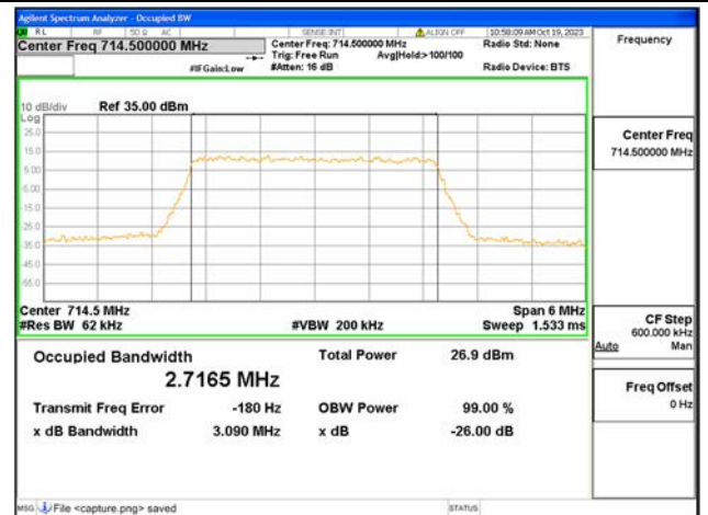
B12 / 3MHz / 256QAM/ High CH
