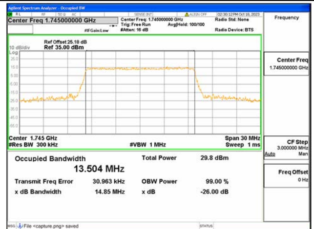
B66 / 15MHz / 16QAM/ Mid CH
