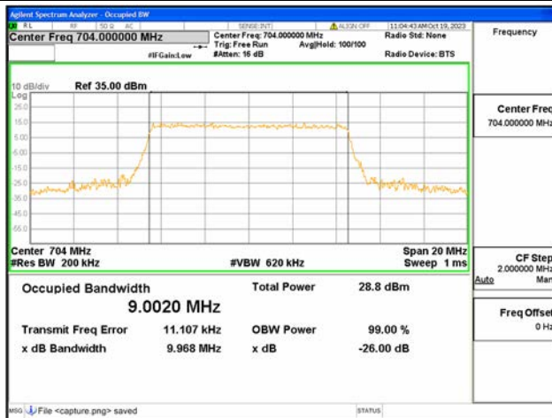
B12 / 10MHz / 64QAM/ Low CH
