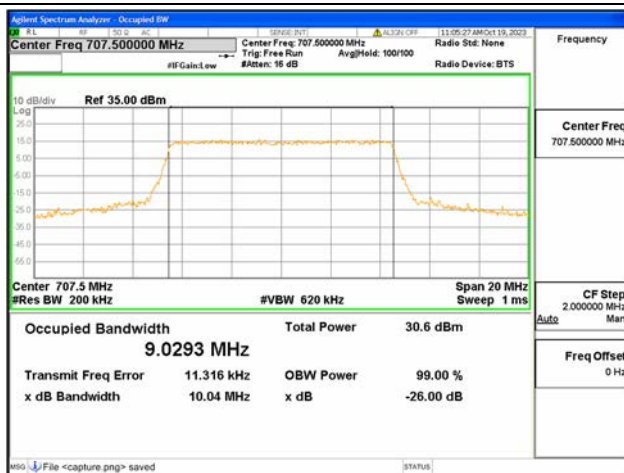
B12 / 10MHz / QPSK/ Mid CH
