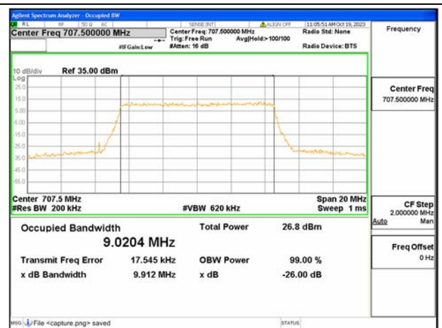
B12 / 10MHz / 256QAM/ Mid CH
