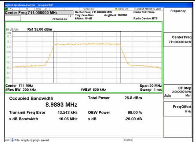
B12 / 10MHz / 256QAM/ High CH
