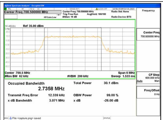
B12 / 3MHz / 16QAM/ Low CH
