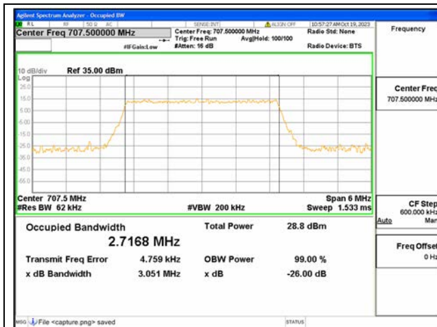
B12 / 3MHz / 64QAM/ Mid CH
