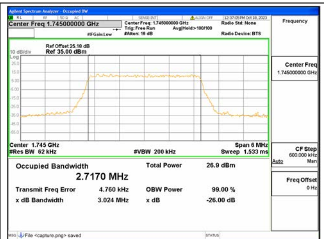
B66 / 3MHz / 256QAM/ Mid CH
