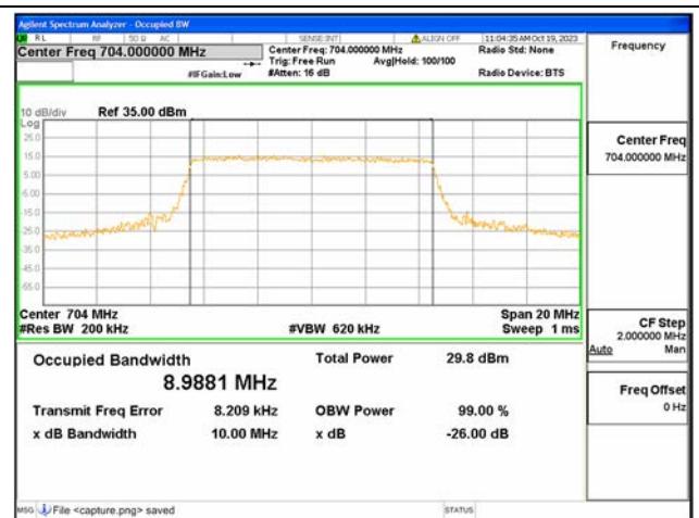
B12 / 10MHz / 16QAM/ Low CH
