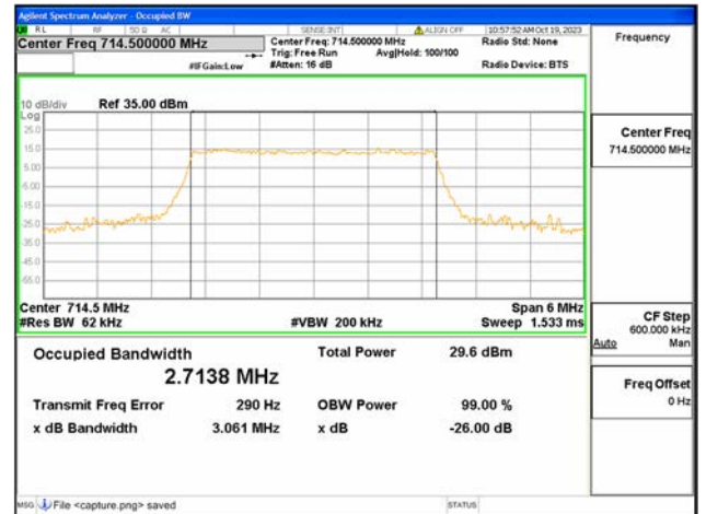
B12 / 3MHz / 16QAM/ High CH
