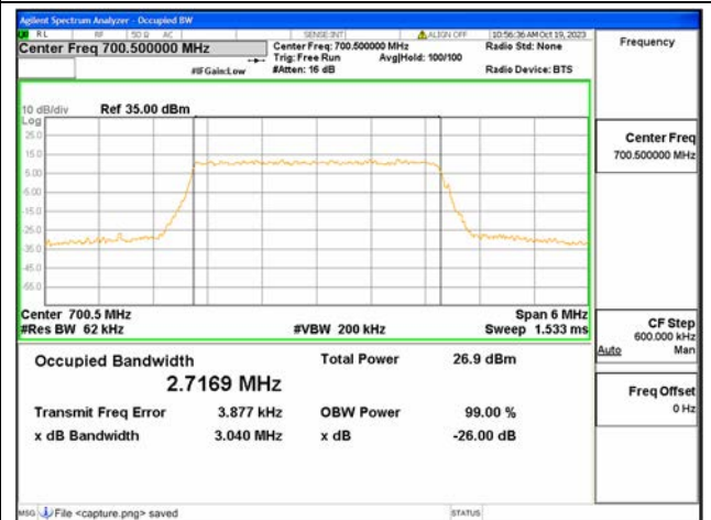
B12 / 3MHz / 256QAM/ Low CH
