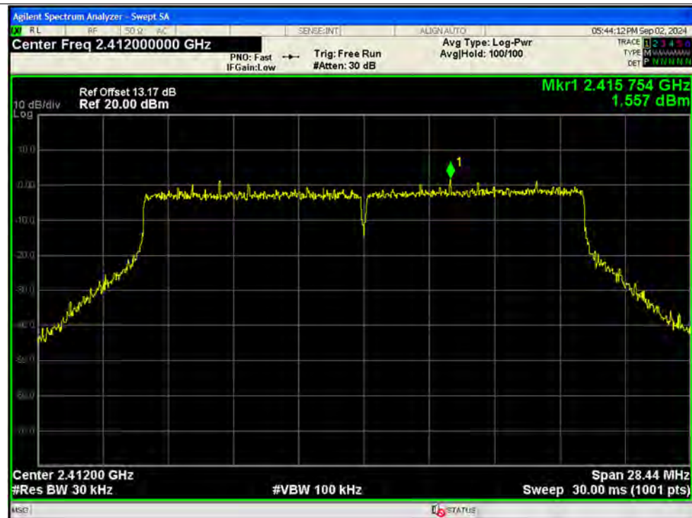
PSD NVNT be20 2412MHz Ant2 SISO
