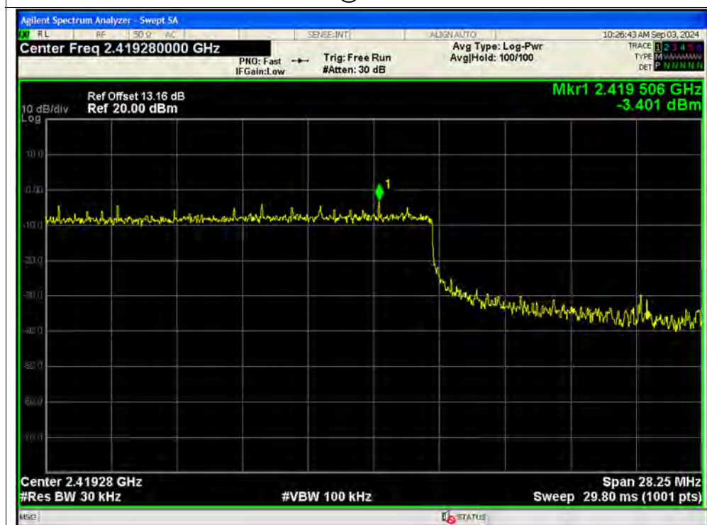
PSD NVNT ax40 242@61 2422MHz Ant2 MIMO
