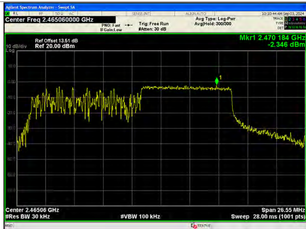
PSD NVNT ax20 106@53 2462MHz Ant2 MIMO
