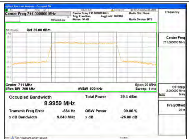
B12 / 10MHz / 64QAM/ High CH
