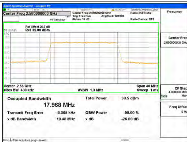
B7 / 20MHz / 16QAM/ High CH
