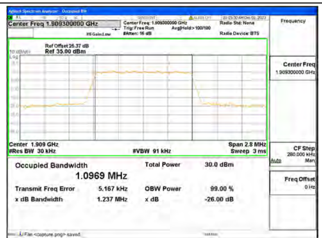
B2 / 1.4MHz / 16QAM/ High CH
