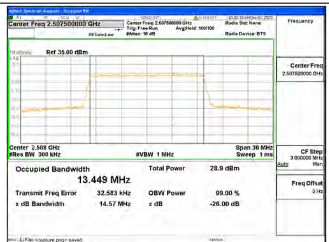
B7 / 15MHz / 64QAM/ Low CH
