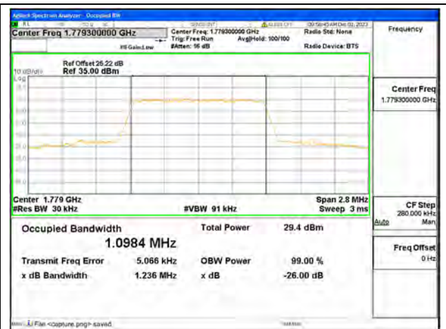
B66 / 1.4MHz / 16QAM/ High CH
