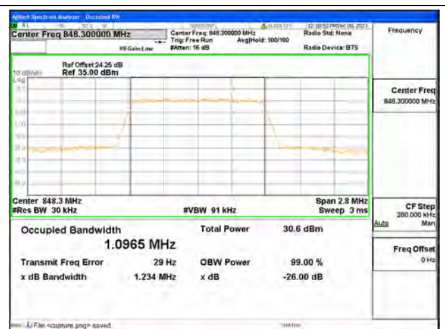
B5 / 1.4MHz / 16QAM/ High CH
