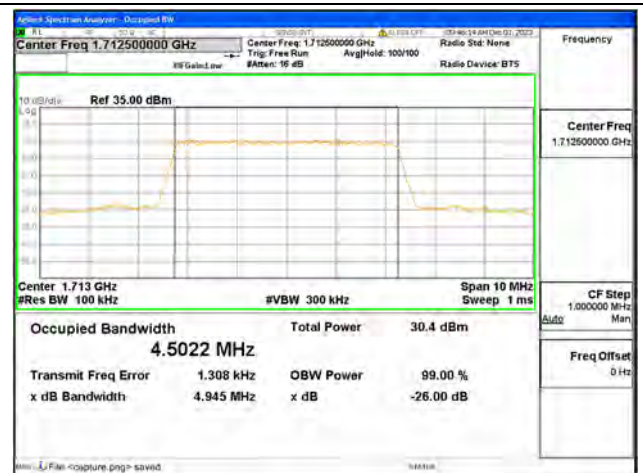
B66 / 5MHz / 64QAM/ Low CH
