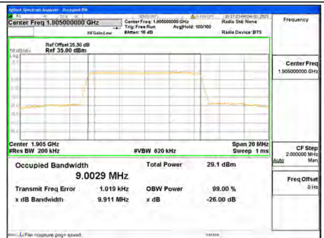
B2 / 10MHz / 64QAM/ High CH
