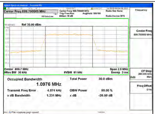
B12 / 1.4MHz / 16QAM/ Low CH
