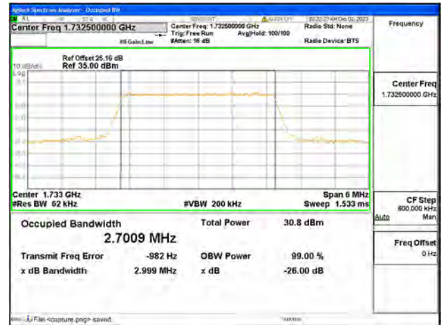
B4 / 3MHz / QPSK/ Mid CH
