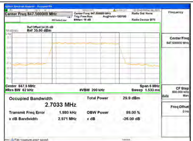
B5 / 3MHz / 64QAM/ High CH
