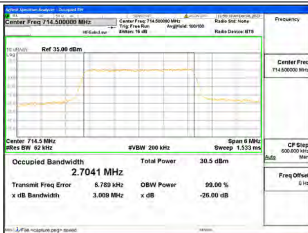
B12 / 3MHz / 16QAM/ High CH
