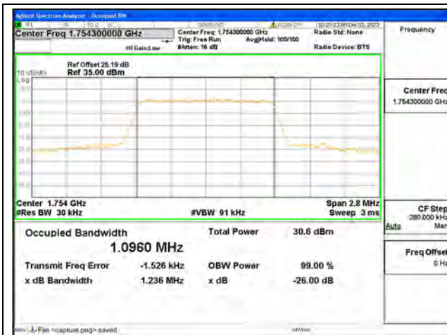
B4 / 1.4MHz / QPSK/ High CH
