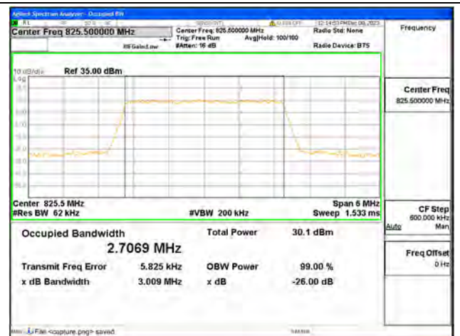
B5 / 3MHz / 64QAM/ Low CH
