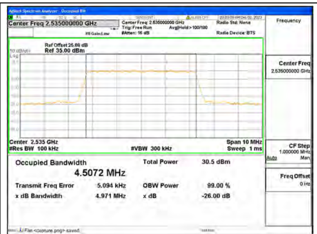
B7 / 5MHz / 16QAM/ Mid CH
