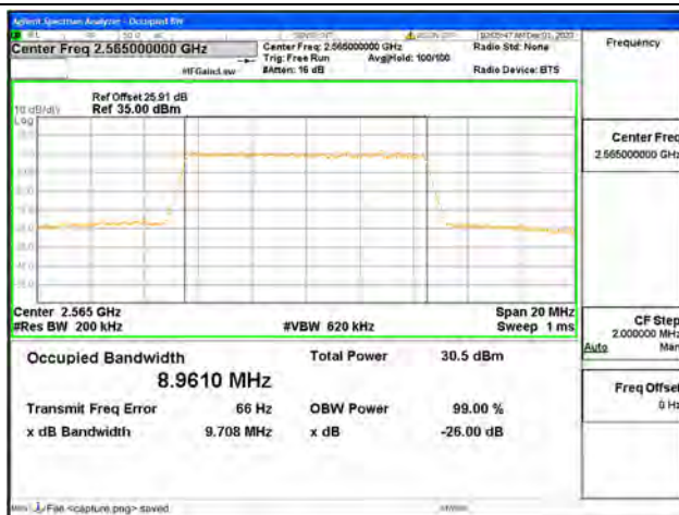
B7 / 10MHz / 16QAM/ High CH
