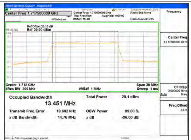
B4 / 15MHz / 64QAM/ Low CH
