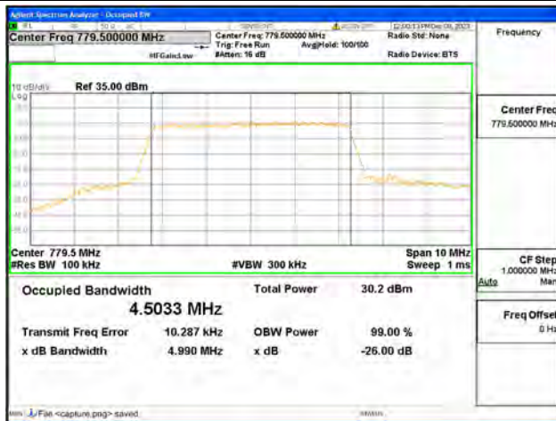
B13 / 5MHz / 64QAM/ Low CH
