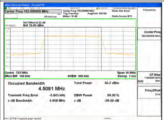
B13 / 5MHz / 64QAM/ Mid CH
