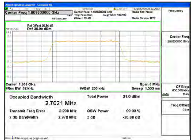
B2 / 3MHz / QPSK/ High CH
