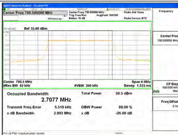
B12 / 3MHz / 16QAM/ Low CH
