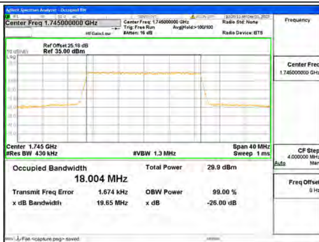
B4 / 20MHz / 16QAM/ High CH
