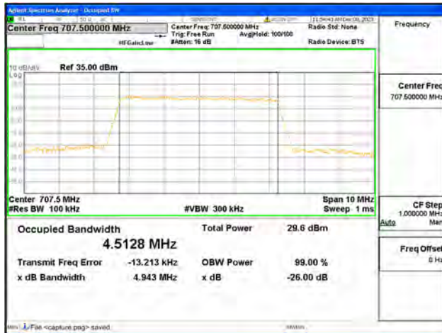
B12 / 5MHz / 64QAM / Mid CH
