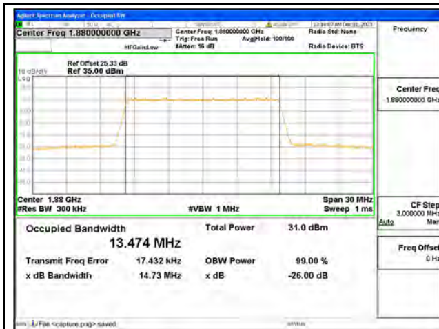
B2 / 15MHz / QPSK/ Mid CH
