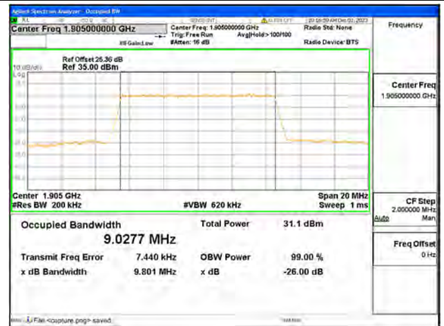
B2 / 10MHz / QPSK/ High CH
