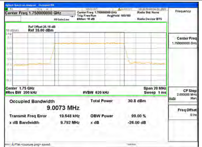
B4 / 10MHz / QPSK/ High CH
