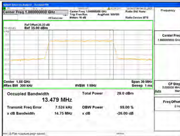
B2 / 15MHz / 64QAM/ Mid CH
