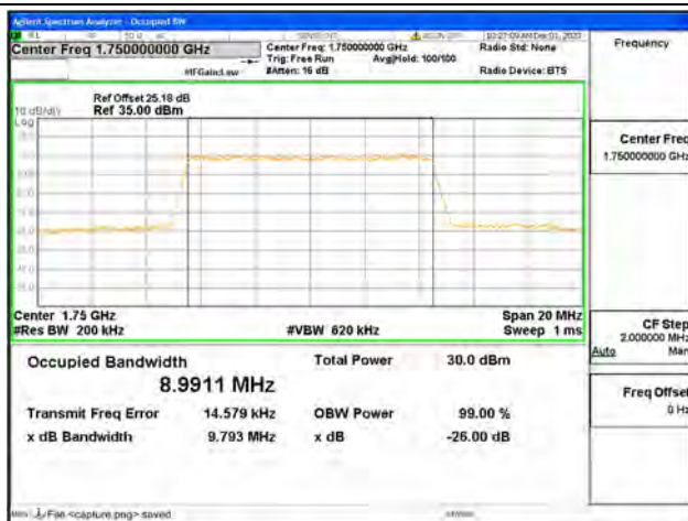
B4 / 10MHz / 16QAM/ High CH
