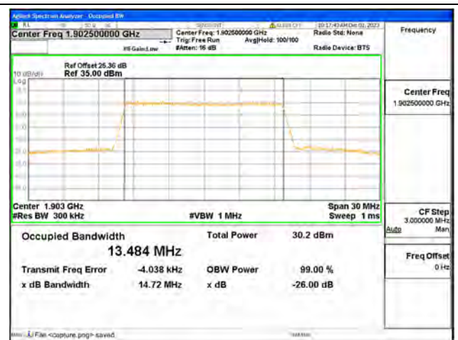
B2 / 15MHz / 16QAM/ High CH
