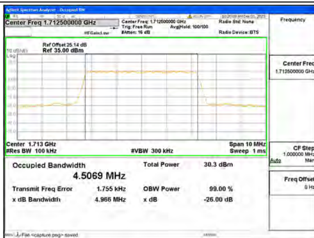
B4 / 5MHz / 16QAM/ Low CH
