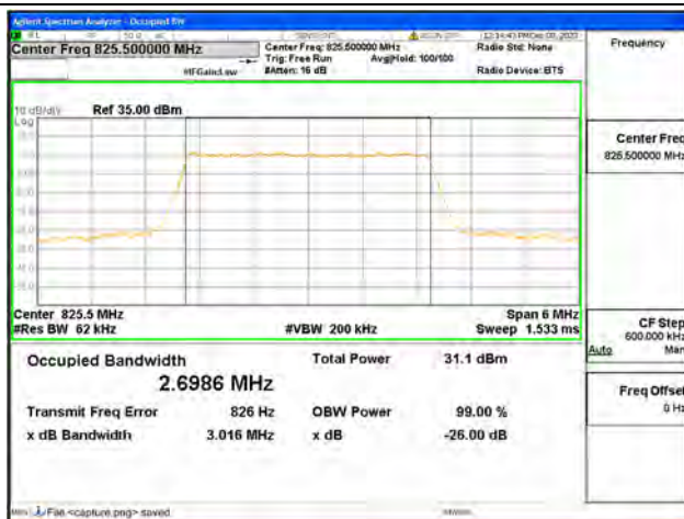
B5 / 3MHz / 16QAM/ Low CH
