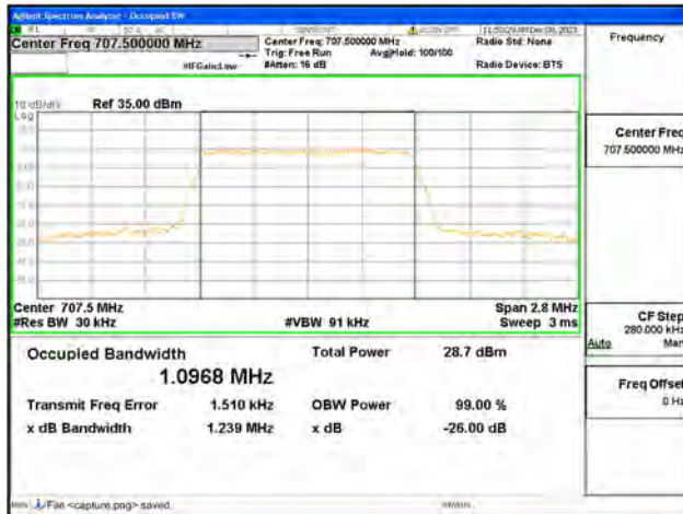
B12 / 1.4MHz / 64QAM/ Mid CH
