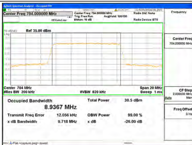
B12 / 10MHz / 16QAM/ Low CH
