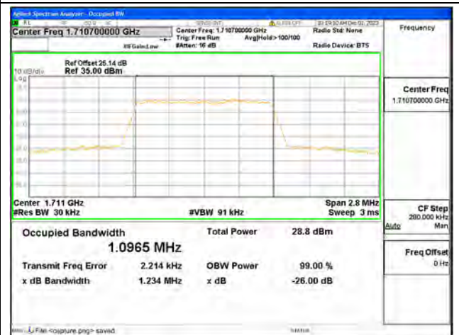
B4 / 1.4MHz / 64QAM/ Low CH
