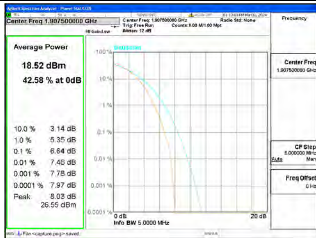
B2 / 5MHz / High CH / 64QAM
