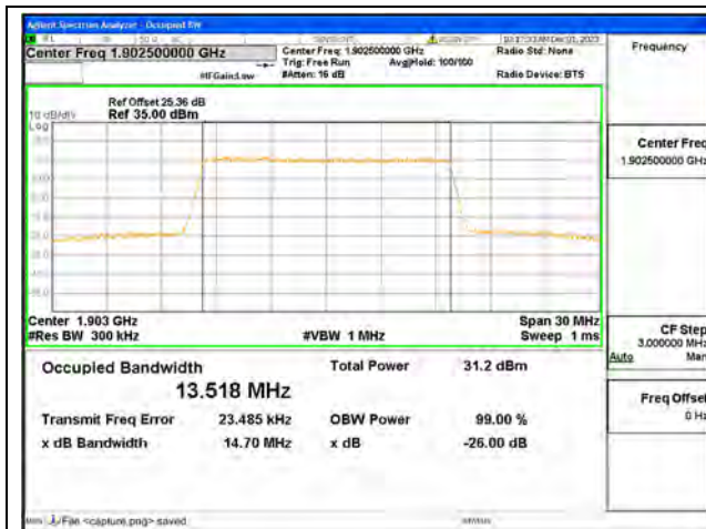
B2 / 15MHz / QPSK/ High CH
