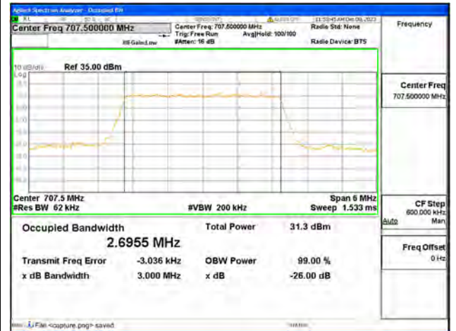
B12 / 3MHz / QPSK/ Mid CH
