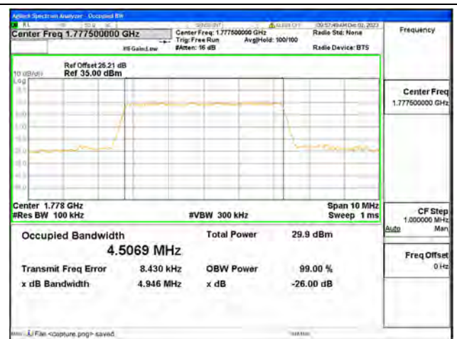
B66 / 5MHz / 16QAM/ High CH
