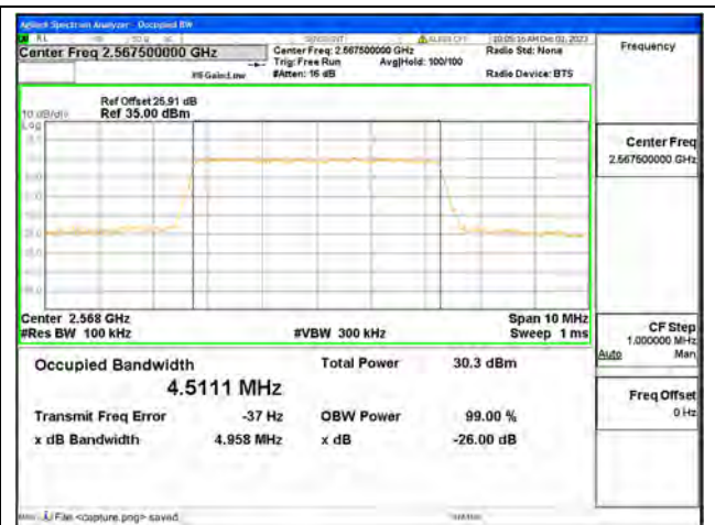
B7 / 5MHz / 16QAM/ High CH
