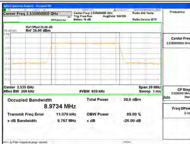
B7 / 10MHz / 16QAM/ Mid CH
