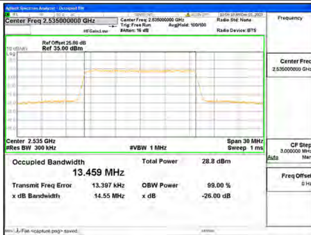
B7 / 15MHz / 64QAM/ Mid CH
