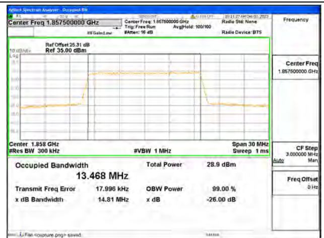
B2 / 15MHz / 64QAM/ Low CH
