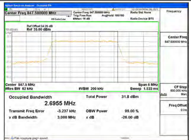
B5 / 3MHz / QPSK/ High CH
