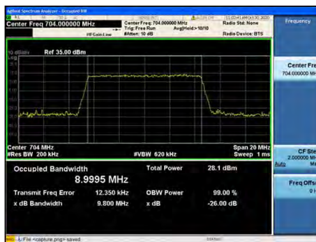
Band12 / 10MHz / Low CH / 64QAM
