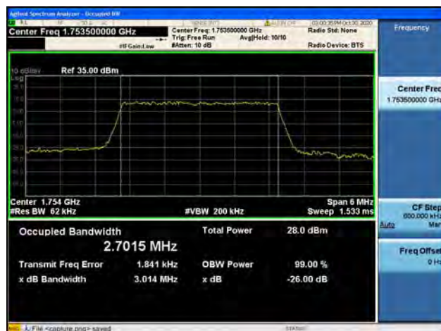
Band4 / 3MHz / High CH / 16QAM
