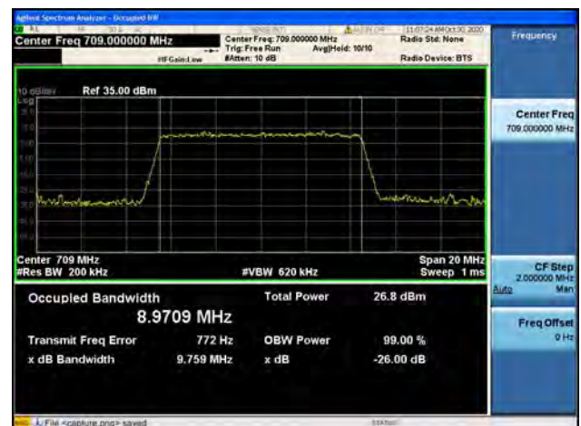
Band17 / 10MHz / Low CH / 64QAM
