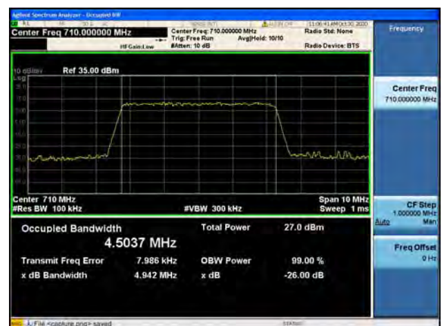
Band17 / 5MHz / Mid CH / 64QAM
