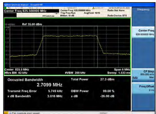
Band5 / 3MHz / Low CH / 64QAM
