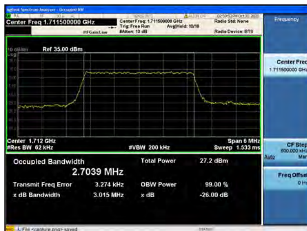
Band4 / 3MHz / Low CH / 16QAM
