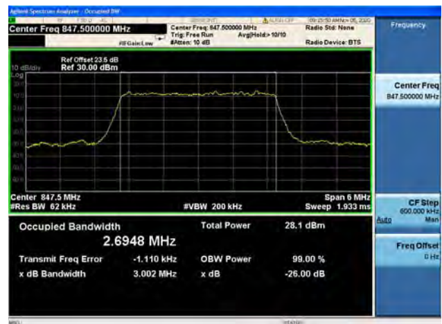
Band26 / 3MHz / High CH / 64QAM
