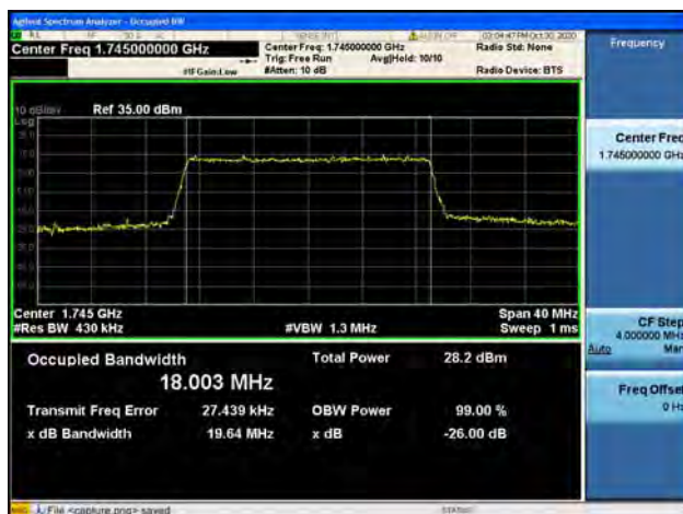
Band4 / 20MHz / High CH / 16QAM
