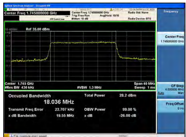
Band4 / 20MHz / High CH / 64QAM
