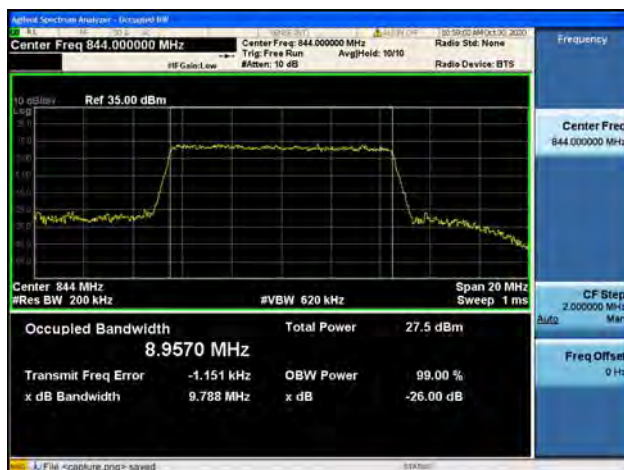
Band5 / 10MHz / High CH / 16QAM
