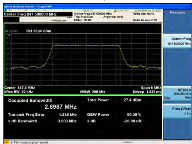
Band5 / 3MHz / High CH / 16QAM
