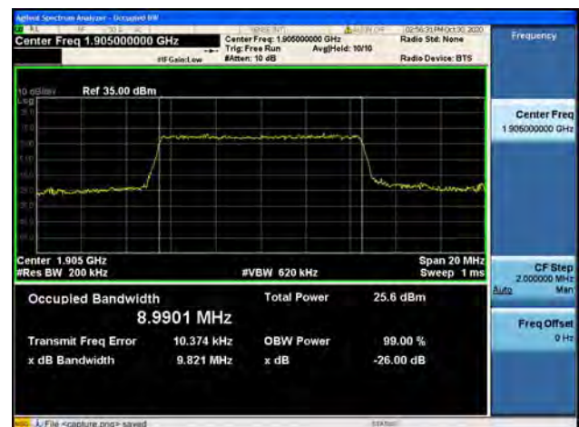
Band2 / 10MHz / High CH / 64QAM
