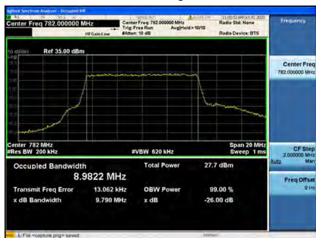
Band13 / 10MHz / High CH / 64QAM
