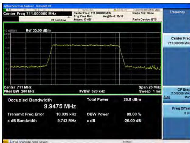
Band17 / 10MHz / High CH / 16QAM
