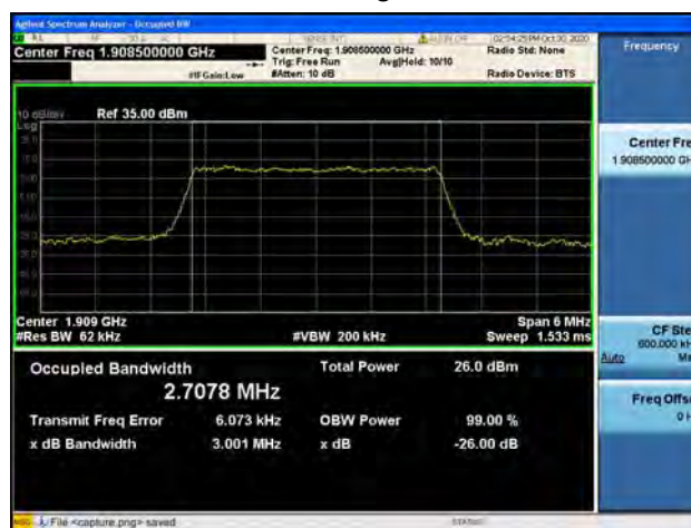
Band2 / 3MHz / High CH / 64QAM
