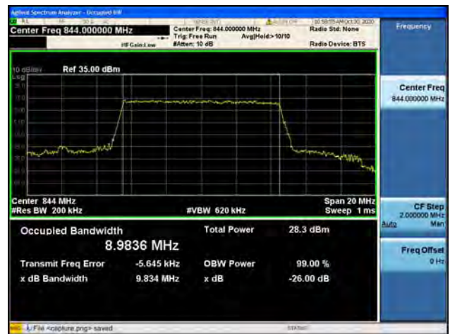
Band5 / 10MHz / High CH / 64QAM
