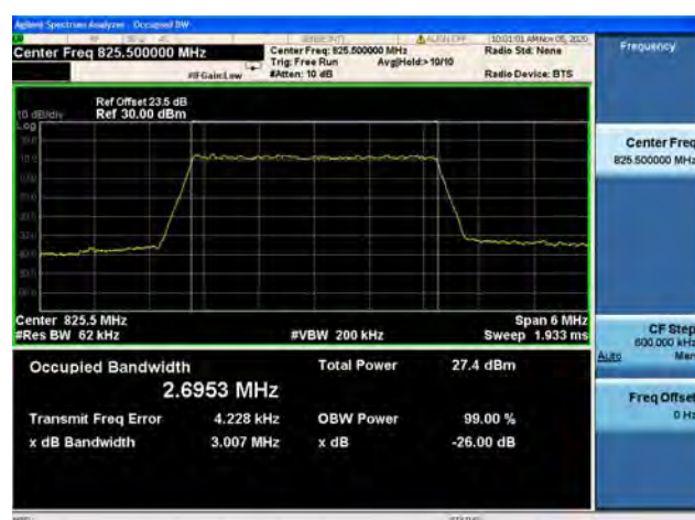
Band26 / 3MHz / Low CH / 16QAM
