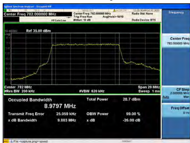
Band13 / 10MHz / High CH / 64QAM
