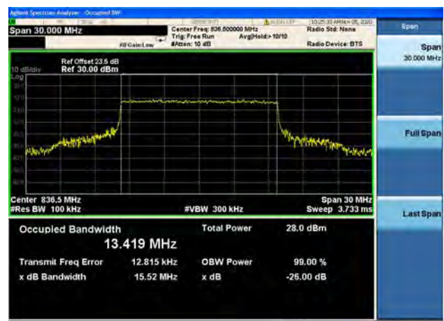
Band26 / 15MHz / Mid CH / 64QAM
