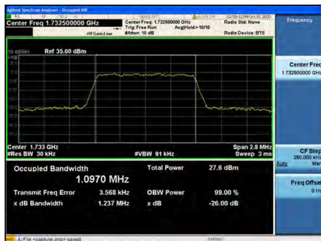
Band4 / 1.4MHz / Mid CH / 16QAM
