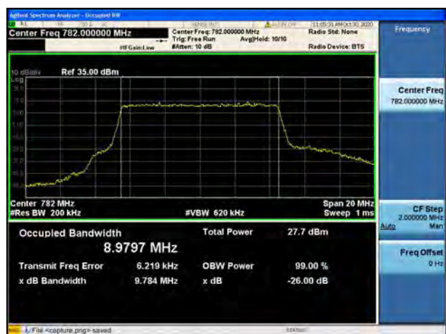
Band13 / 10MHz / High CH / 16QAM
