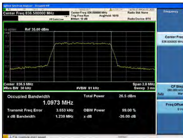
Band5 / 1.4MHz / Mid CH / 16QAM
