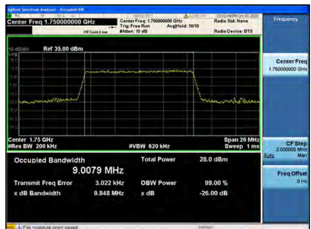
Band4 / 10MHz / High CH / 64QAM
