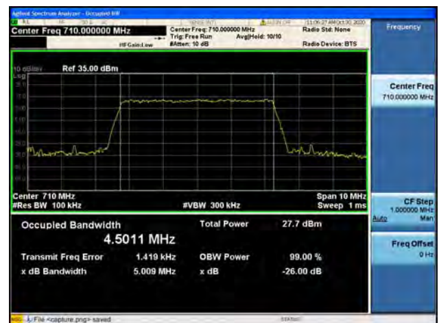
Band17 / 5MHz / Mid CH / 64QAM
