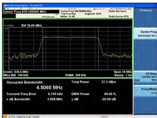
Band5 / 5MHz / Mid CH / 64QAM
