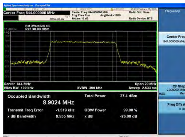
Band26 / 10MHz / High CH / 16QAM
