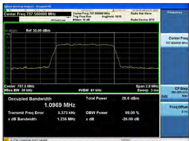
Band12 / 1.4MHz / Mid CH / 16QAM
