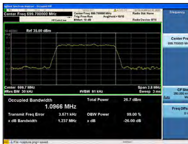
Band12 / 1.4MHz / Mid CH / QPSK
