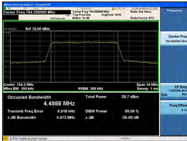
Band13 / 5MHz / High CH / 64QAM
