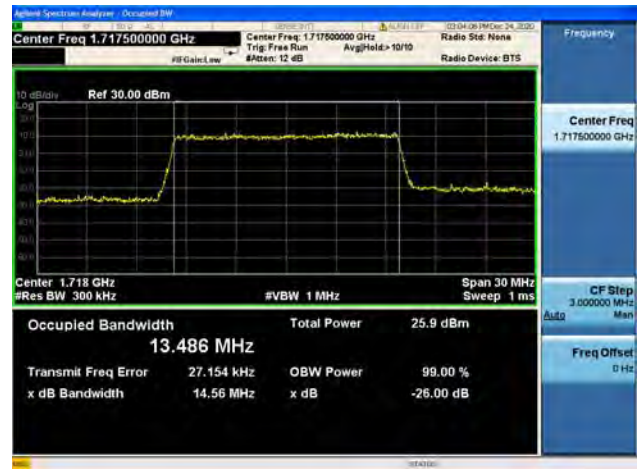
Band66 / 15MHz / Mid CH / QPSK
