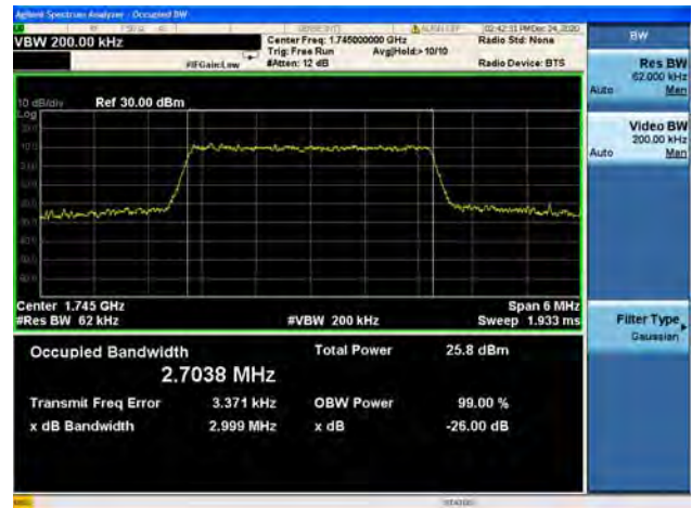
Band66 / 3MHz / High CH / QPSK
