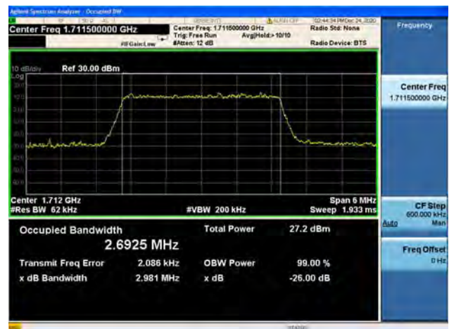
Band66 / 3MHz / Low CH / 64QAM
