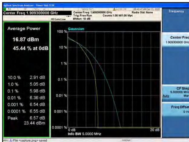
Band2 / 3MHz / Low CH / 16QAM
