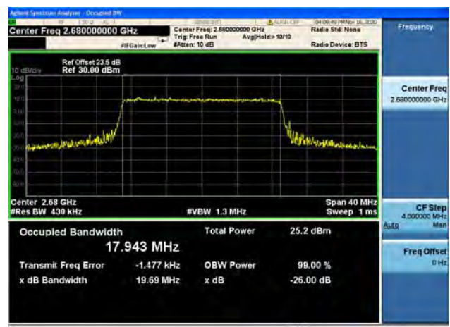
Band41 / 20MHz / High CH / 64QAM
