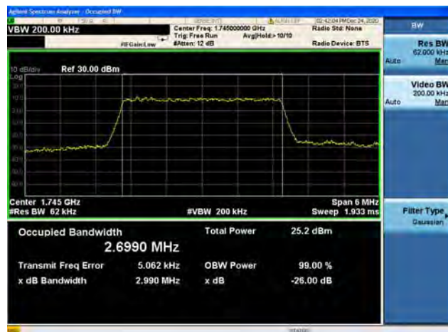
Band66 / 3MHz / High CH / 16QAM
