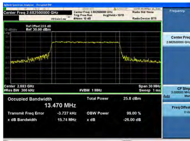
Band41 / 15MHz / High CH / 64QAM
