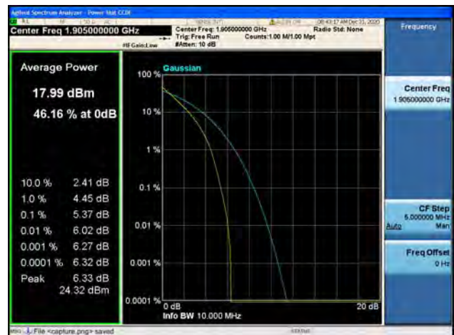
Band2 / 10MHz / High CH / 64QAM
