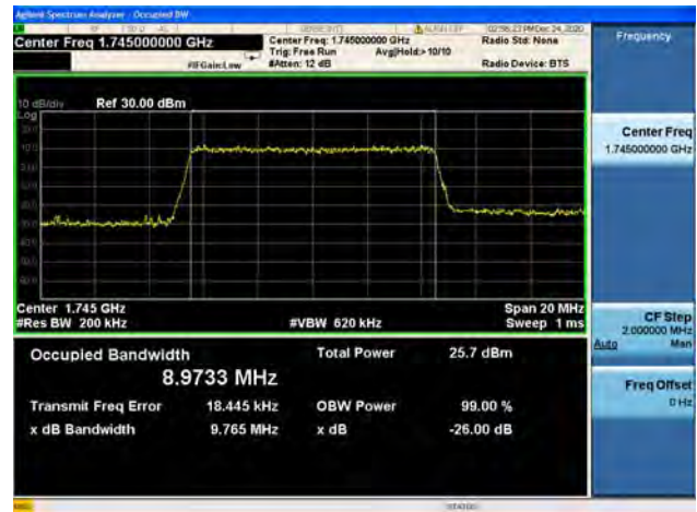
Band66 / 10MHz / High CH / QPSK
