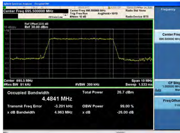
Band71 / 5MHz / High CH / 64QAM
