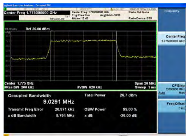
Band66 / 10MHz / High CH / 64QAM
