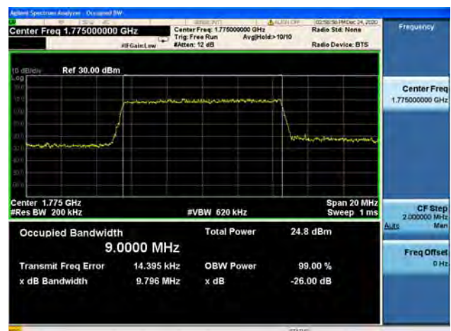
Band66 / 10MHz / High CH / 64QAM
