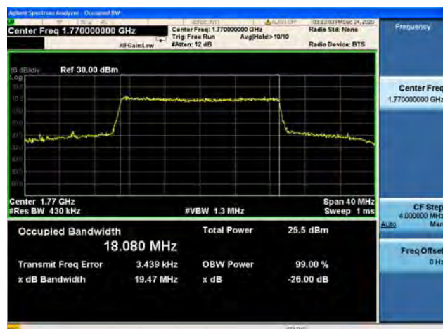
Band66 / 20MHz / High CH / 16QAM
