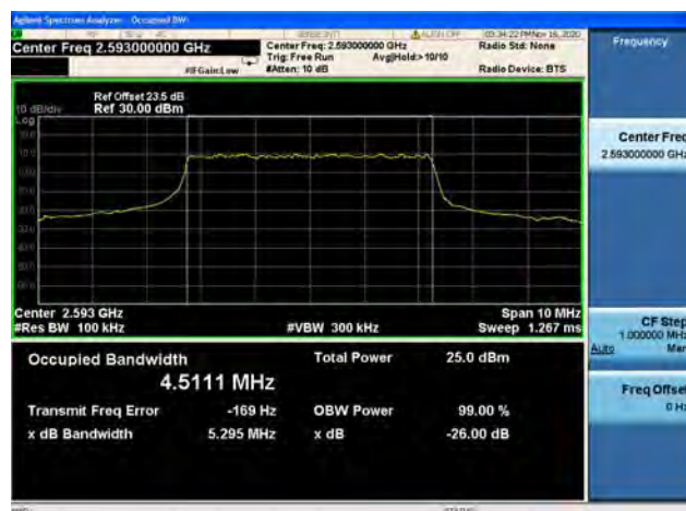
Band41 / 5MHz / Mid CH / 16QAM
