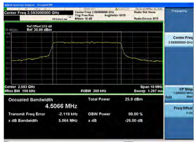
Band41 / 5MHz / Mid CH / 64QAM
