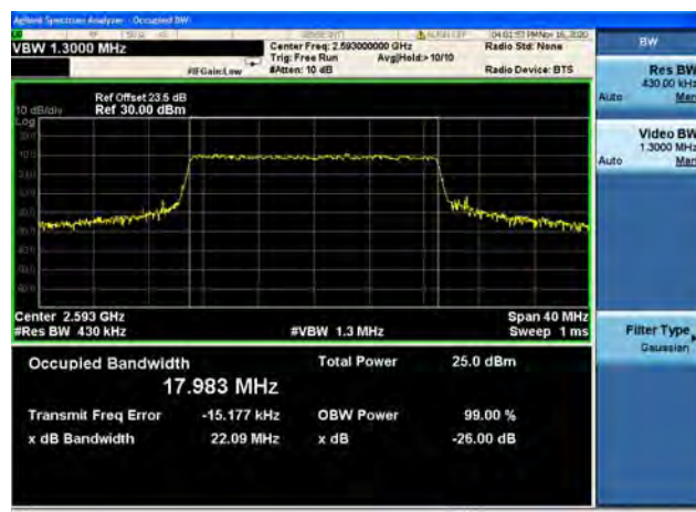
Band41 / 20MHz / High CH / 16QAM
