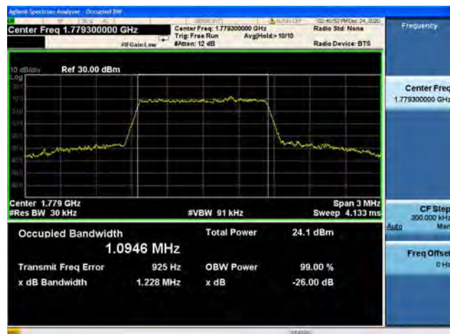
Band66 / 3MHz / Low CH / 16QAM
