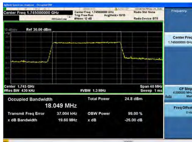
Band66 / 20MHz / High CH / 16QAM
