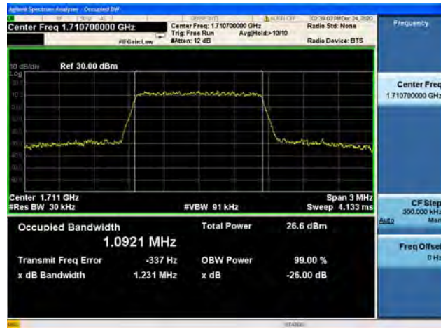
Band66 / 1.4MHz / Low CH / 64QAM
