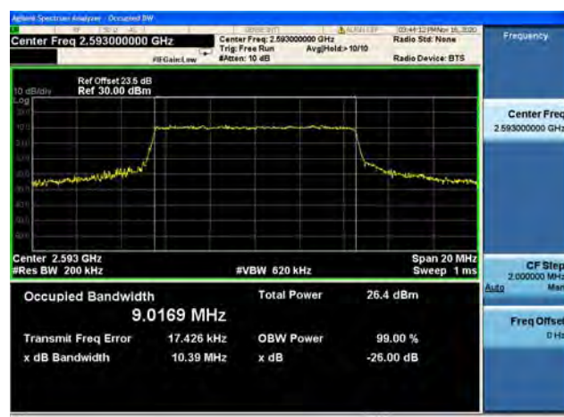
Band41 / 10MHz / Mid CH / 64QAM
