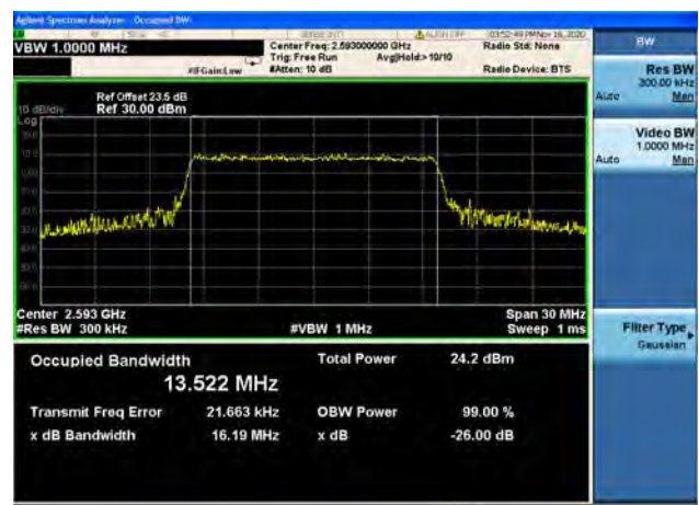
Band41 / 15MHz / Mid CH / 64QAM
