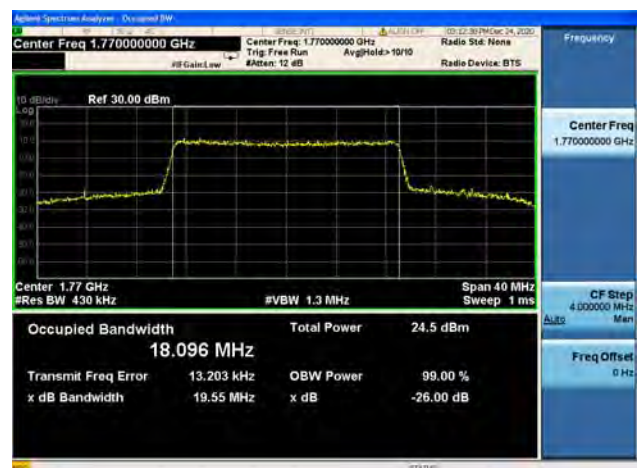
Band66 / 20MHz / High CH / 64QAM
