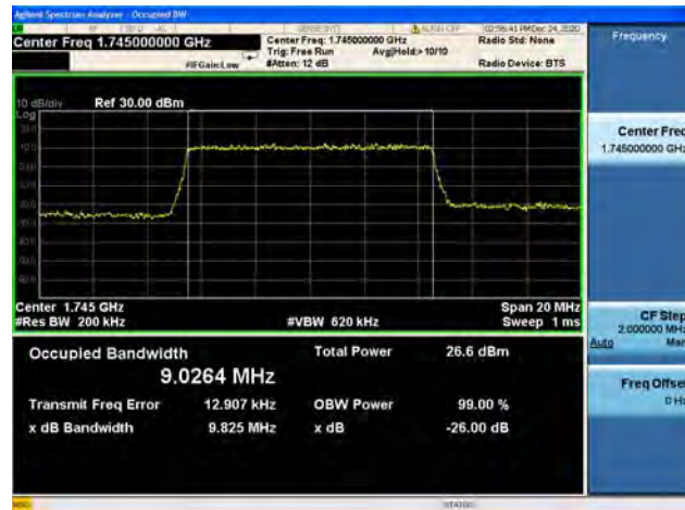
Band66 / 10MHz / Mid CH / 64QAM
