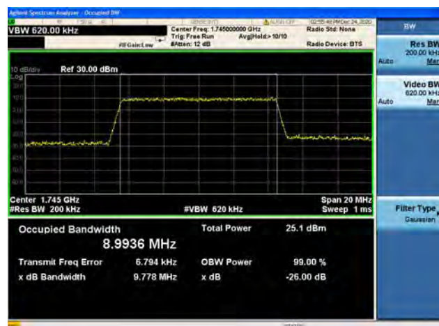
Band66 / 10MHz / High CH / 16QAM
