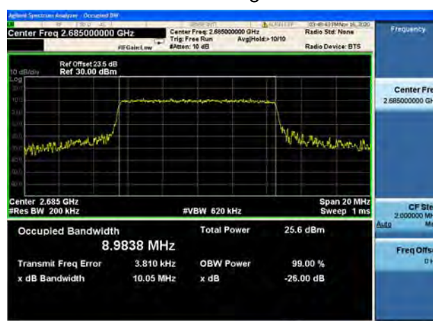
Band41 / 10MHz / High CH / 64QAM
