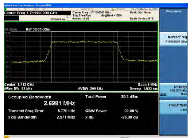
Band66 / 3MHz / Low CH / 64QAM
