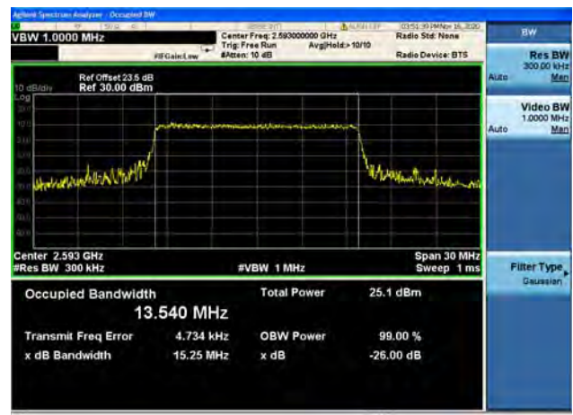
Band41 / 15MHz / Mid CH / 64QAM
