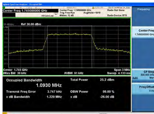
Band66 / 1.4MHz / Mid CH / 16QAM
