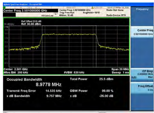
Band41 / 10MHz / Low CH / 64QAM
