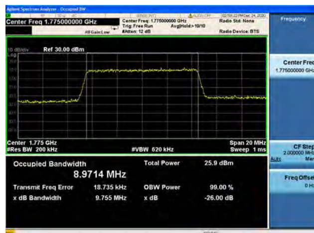
Band66 / 10MHz / High CH / 16QAM
