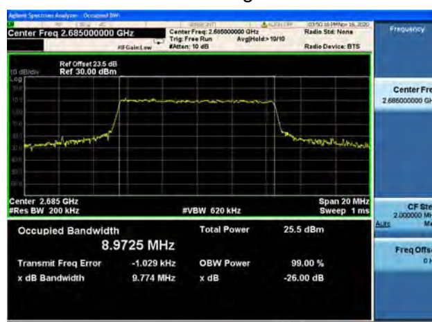
Band41 / 10MHz / High CH / 64QAM
