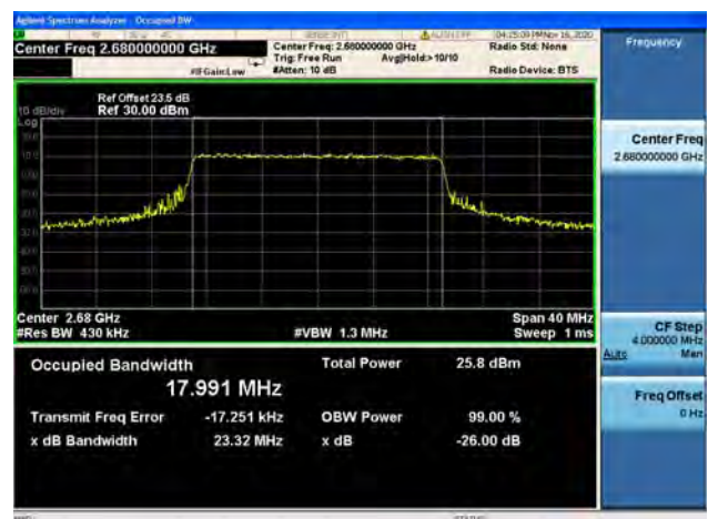
Band41 / 20MHz / High CH / 64QAM
