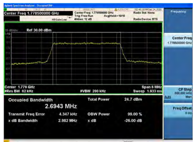
Band66 / 3MHz / High CH / 64QAM
