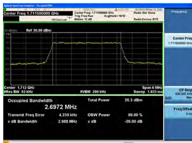
Band66 / 3MHz / Low CH / 16QAM
