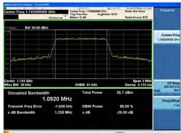
Band66 / 1.4MHz / Mid CH / 64QAM
