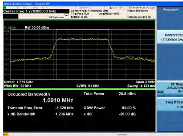
Band66 / 1.4MHz / High CH / 64QAM
