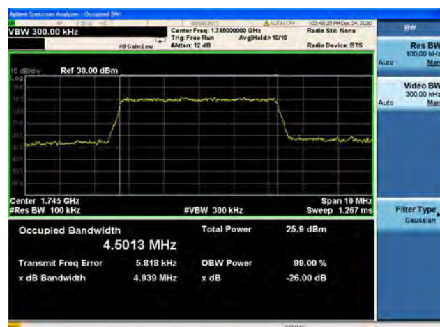
Band66 / 5MHz / Mid CH / 16QAM
