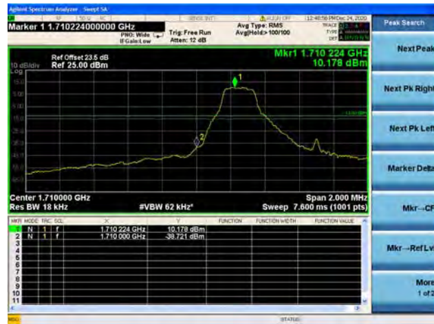
Band66 / 1.4MHz / High CH / QPSK / 1 RB
