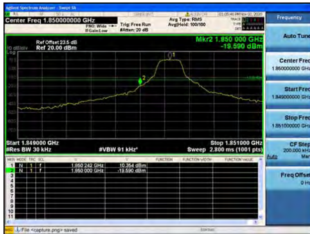
Band25 / 3MHz / High CH / QPSK / 1 RB
