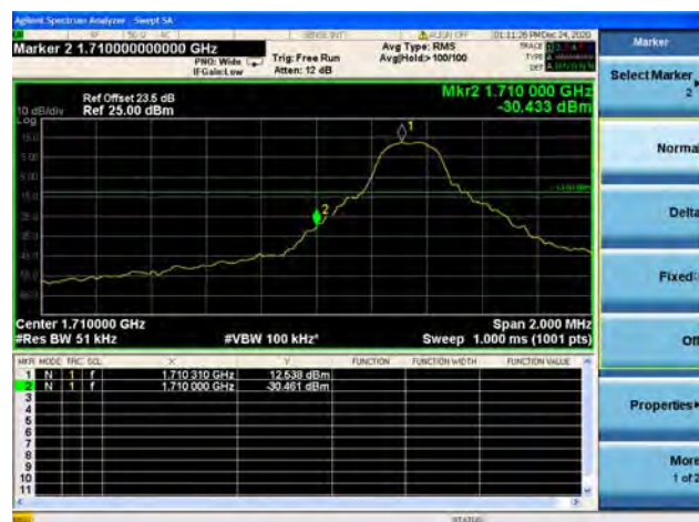
Band66 / 5MHz / High CH / QPSK / 1 RB
