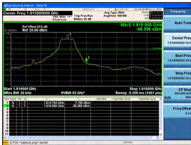
Band25 / 1.4MHz / High CH / QPSK / 1 RB
