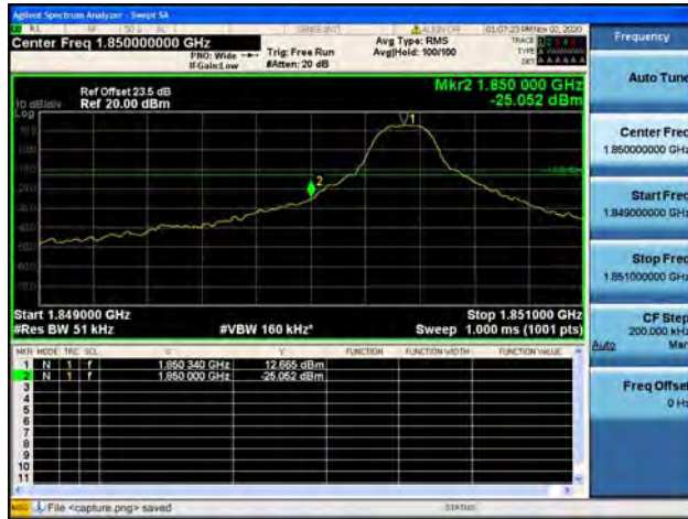
Band25 / 5MHz / High CH / QPSK / 1 RB
