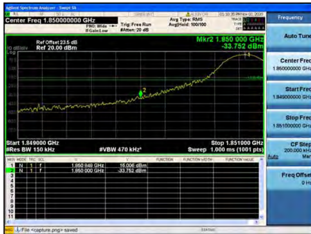
Band25 / 15MHz / High CH / QPSK / 1 RB
