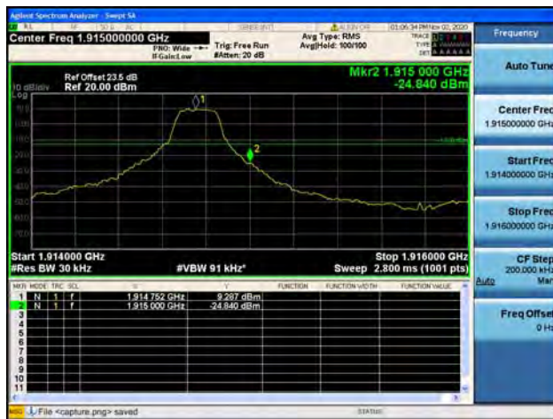
Band25 / 3MHz / High CH / QPSK / 1 RB
