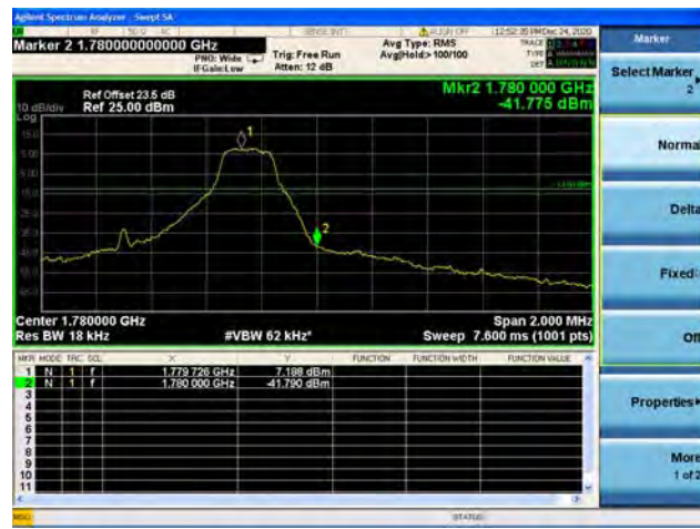
Band66 / 1.4MHz / High CH / QPSK / 1 RB
