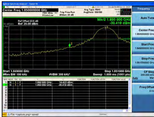
Band25 / 10MHz / High CH / QPSK / 1 RB
