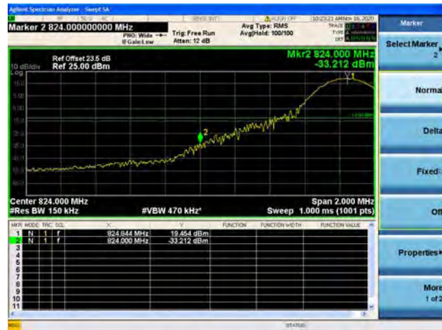
Band26 / 15MHz / High CH / QPSK / 1 RB
