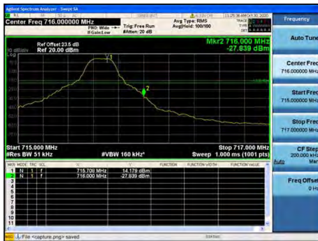
Band17 / 5MHz / High CH / QPSK / 1 RB
