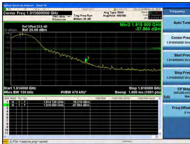
Band25 / 15MHz / High CH / QPSK / 1 RB
