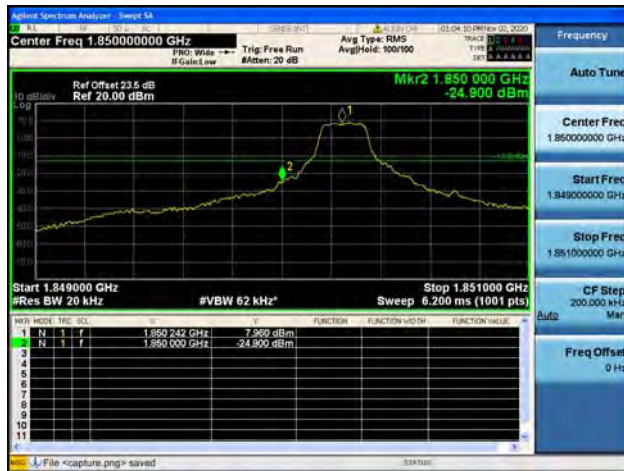
Band25 / 1.4MHz / High CH / QPSK / 1 RB
