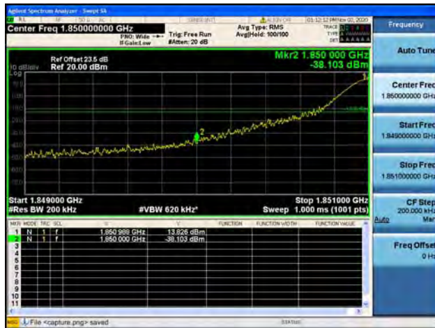
Band25 / 20MHz / High CH / QPSK / 1 RB
