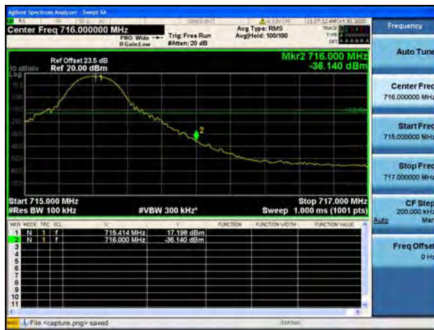
Band17 / 10MHz / High CH / QPSK / 1 RB
