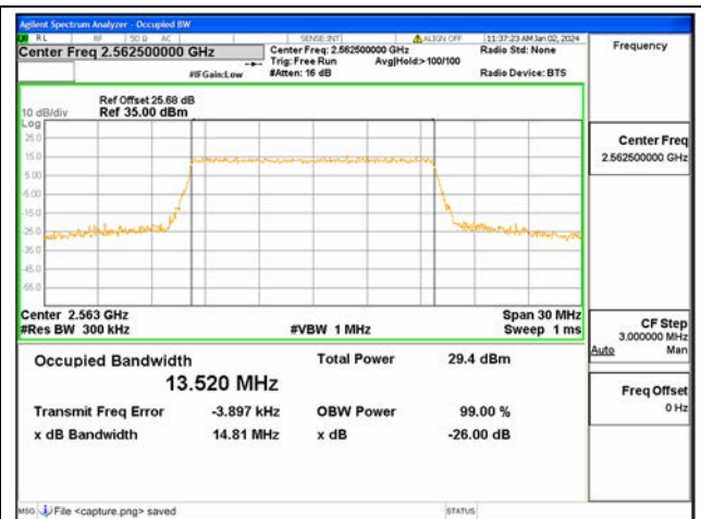
B7 / 15MHz / 16QAM/ High CH
