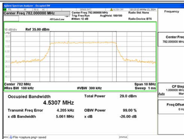
B13 / 5MHz / 16QAM/ Mid CH
