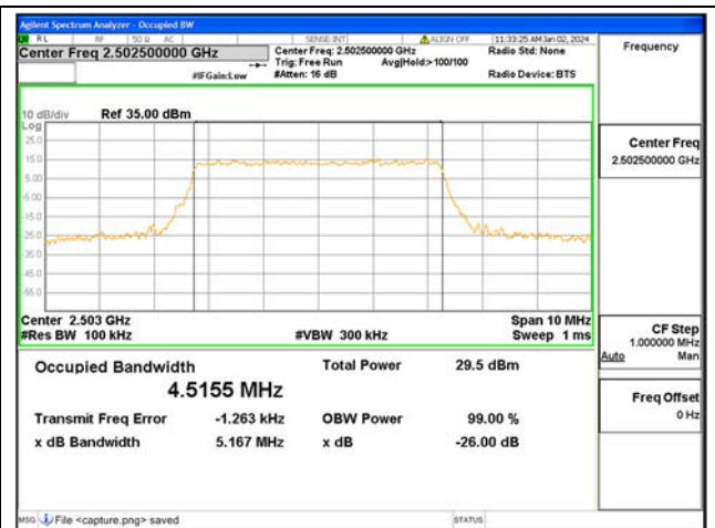
B7 / 5MHz / 16QAM/ Low CH
