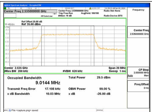
B7 / 10MHz / 16QAM/ Mid CH
