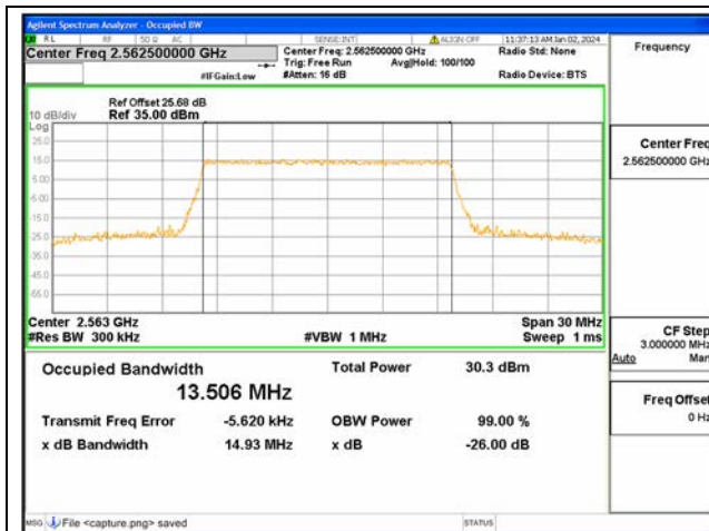
B7 / 15MHz / QPSK/ High CH
