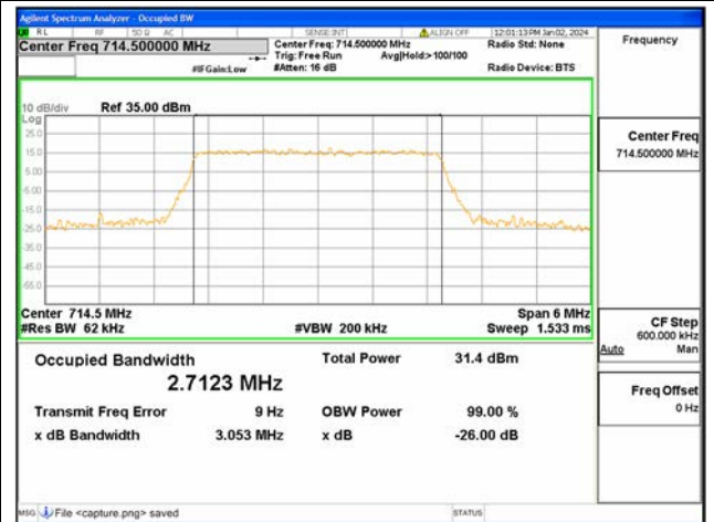
B12 / 3MHz / QPSK/ High CH
