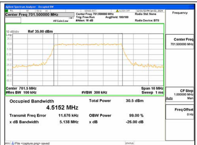
B12 / 5MHz / 16QAM/ Low CH
