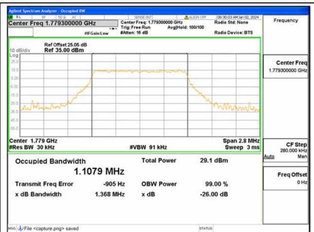
B66 / 1.4MHz / 16QAM/ High CH
