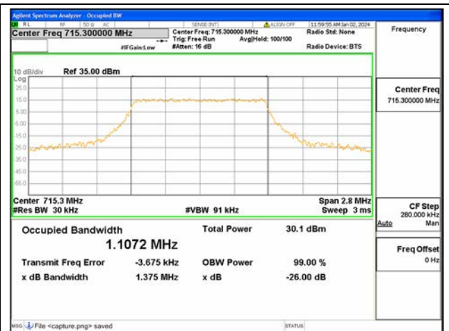
B12 / 1.4MHz / 16QAM/ High CH
