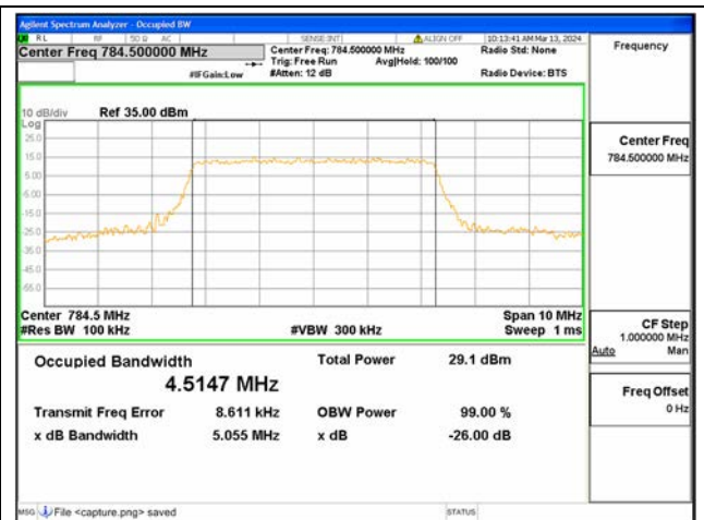
B13 / 5MHz / 16QAM/ High CH
