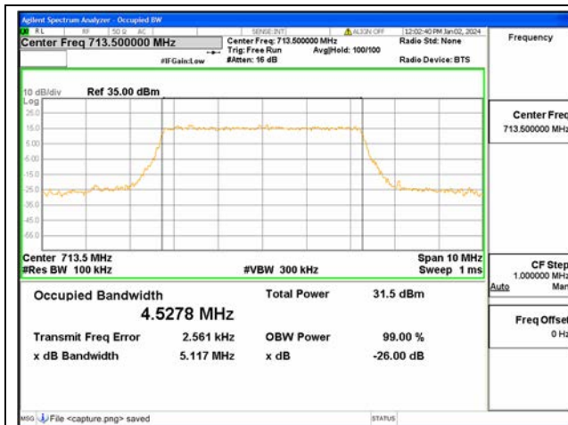
B12 / 5MHz / QPSK/ High CH
