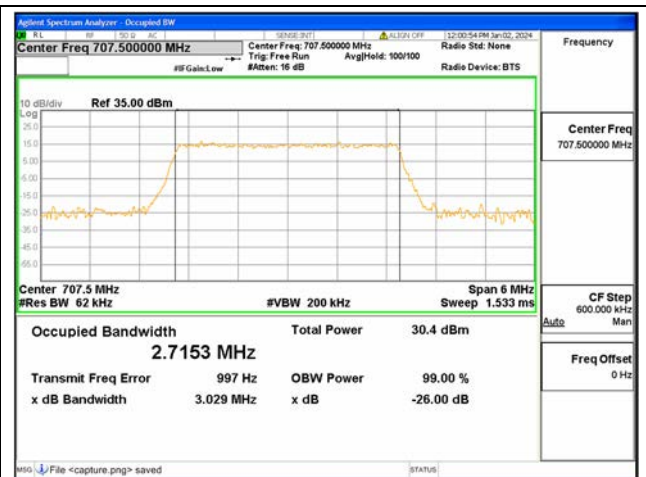
B12 / 3MHz / 16QAM/ Mid CH
