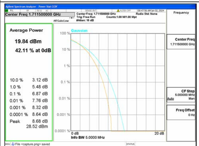
B66 / 3MHz / Low CH / 64QAM
