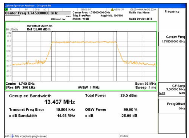
B66 / 15MHz / 64QAM/ Mid CH
