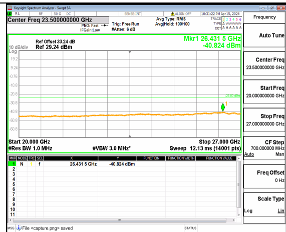
n41 (20GHz-27GHz) 50M DFT-s-OFDM QPSK Inner_1RB_Right Low
