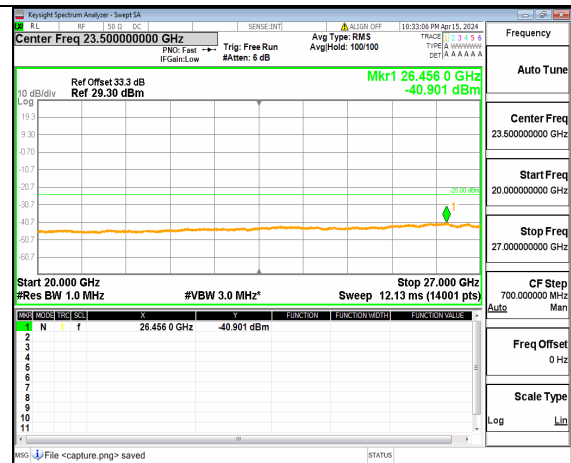
n41 (20GHz-27GHz) 50M DFT-s-OFDM BPSK Inner_1RB_Left Mid
