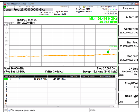
n41 (20GHz-27GHz) 90M DFT-s-OFDM BPSK Inner_1RB_Left Low
