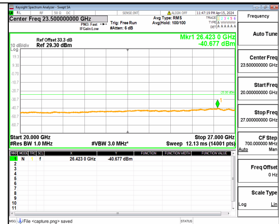
n41 (20GHz-27GHz) 90M DFT-s-OFDM QPSK Inner_1RB_Right Mid
