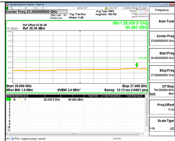
n41 (20GHz-27GHz) 60M DFT-s-OFDM QPSK Inner_1RB_Left High
