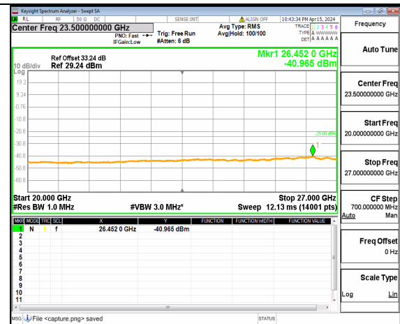
n41 (20GHz-27GHz) 60M DFT-s-OFDM BPSK Inner_1RB_Left Low
