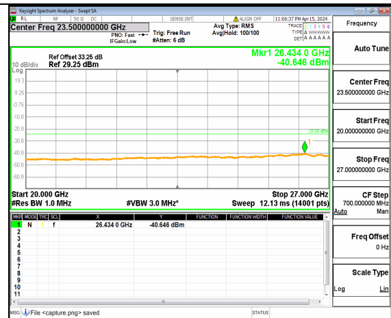
n41 (20GHz-27GHz) 70M DFT-s-OFDM BPSK Inner_1RB_Left Low
