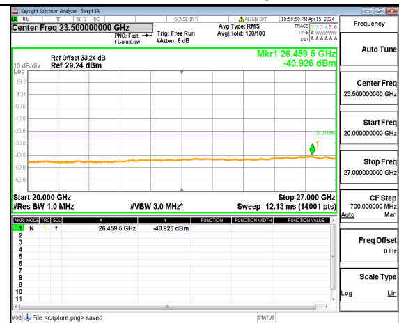
n41 (20GHz-27GHz) 60M DFT-s-OFDM QPSK Inner_1RB_Left Low
