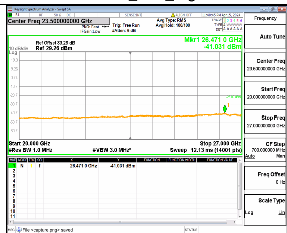
n41 (20GHz-27GHz) 90M DFT-s-OFDM QPSK Inner_1RB_Left Low
