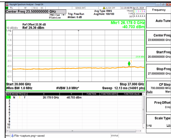
n41 (20GHz-27GHz) 70M DFT-s-OFDM QPSK Inner_1RB_Left High
