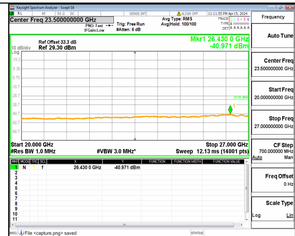
n41 (20GHz-27GHz) 70M DFT-s-OFDM BPSK Inner_1RB_Left Mid
