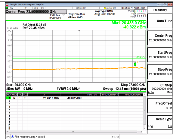
n41 (20GHz-27GHz) 80M DFT-s-OFDM QPSK Inner_1RB_Left High
