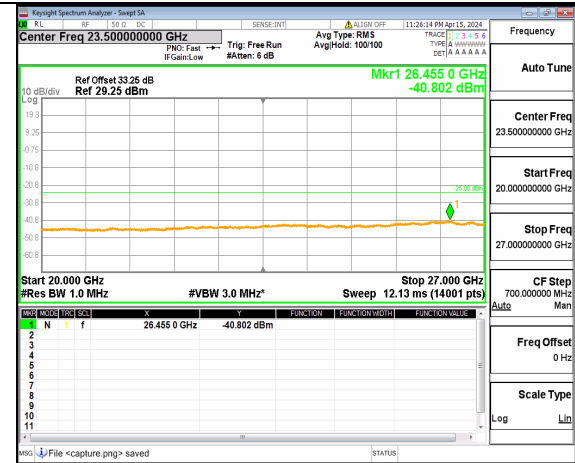
n41 (20GHz-27GHz) 80M DFT-s-OFDM QPSK Inner_1RB_Right Low
