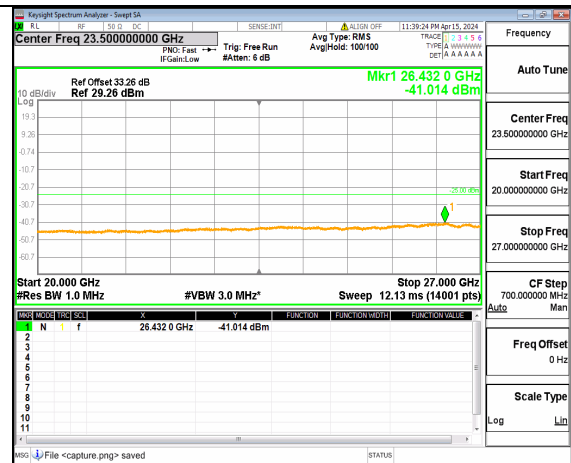
n41 (20GHz-27GHz) 90M DFT-s-OFDM BPSK Inner_1RB_Right Low
