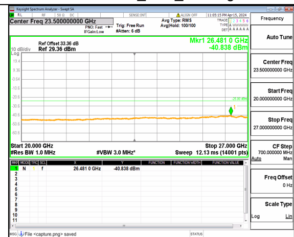
n41 (20GHz-27GHz) 60M DFT-s-OFDM QPSK Inner_1RB_Right High
