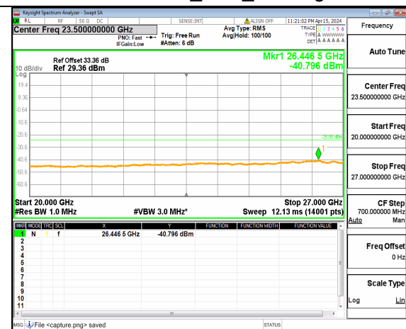
n41 (20GHz-27GHz) 70M DFT-s-OFDM QPSK Inner_1RB_Right High
