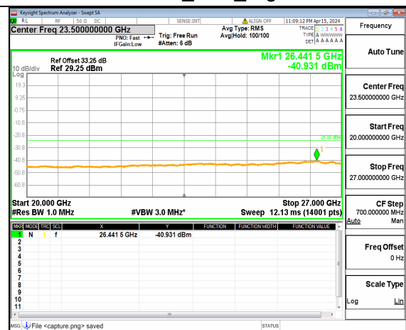
n41 (20GHz-27GHz) 70M DFT-s-OFDM QPSK Inner_1RB_Left Low
