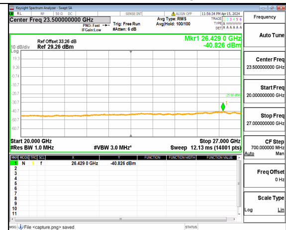
n41 (20GHz-27GHz) 100M DFT-s-OFDM QPSK Inner_1RB_Left Low
