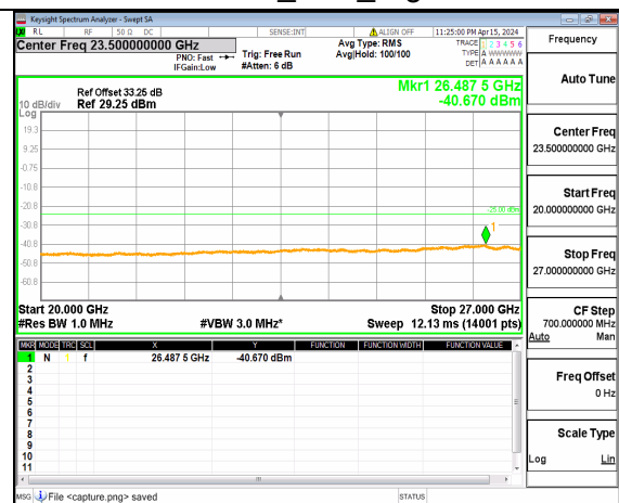
n41 (20GHz-27GHz) 80M DFT-s-OFDM QPSK Inner_1RB_Left Low
