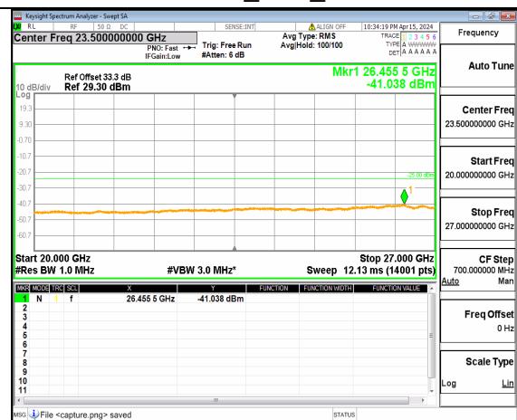
n41 (20GHz-27GHz) 50M DFT-s-OFDM BPSK Inner_1RB_Right Mid
