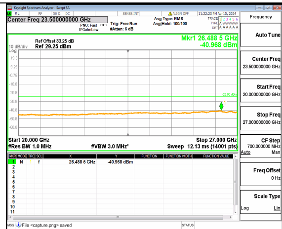
n41 (20GHz-27GHz) 80M DFT-s-OFDM BPSK Inner_1RB_Left Low
