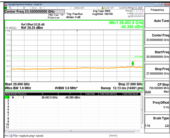
n41 (20GHz-27GHz) 70M DFT-s-OFDM BPSK Inner_1RB_Right Low
