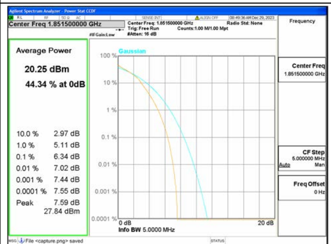
B2 / 3MHz / Low CH / 64QAM
