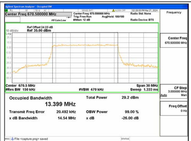
B71 / 15MHz / 16QAM/ Low CH
