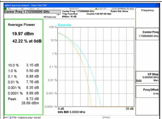
B4 / 1.4MHz / Mid CH / 64QAM
