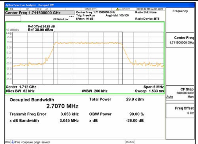
B66 / 3MHz / 64QAM/ Low CH
