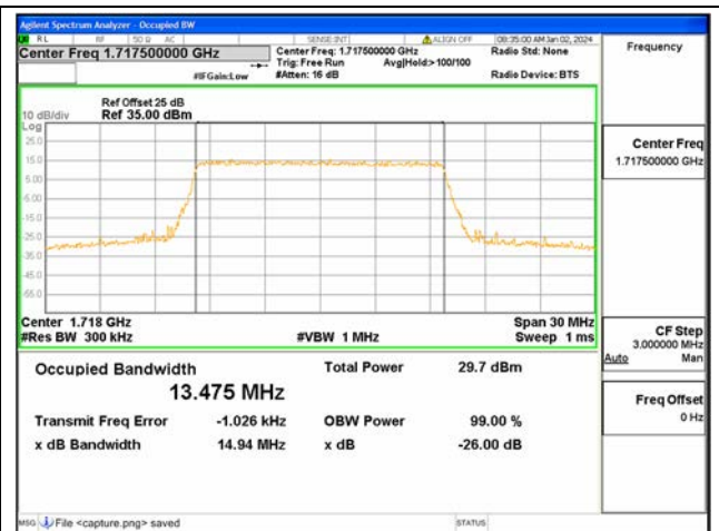
B66 / 15MHz / 16QAM/ Low CH
