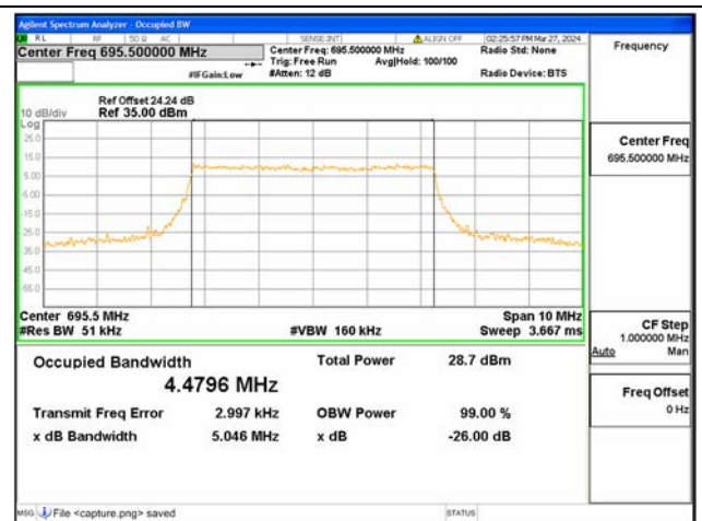
B71 / 5MHz / 16QAM/ High CH
