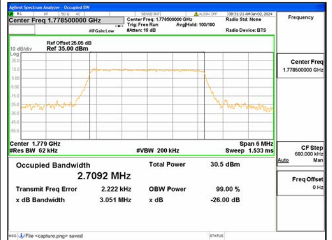
B66 / 3MHz / QPSK/ High CH
