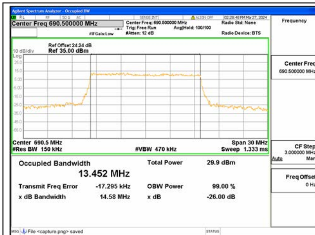
B71 / 15MHz / QPSK/ High CH
