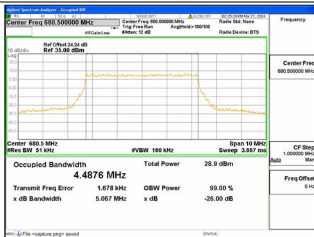
B71 / 5MHz / 16QAM/ Mid CH
