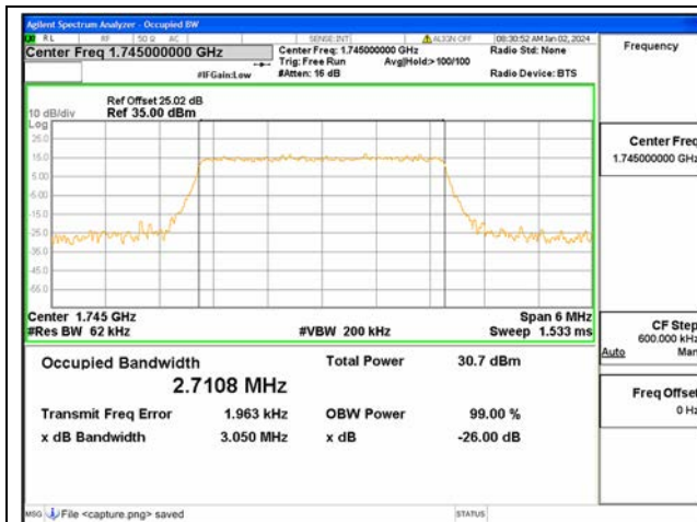
B66 / 3MHz / QPSK/ Mid CH
