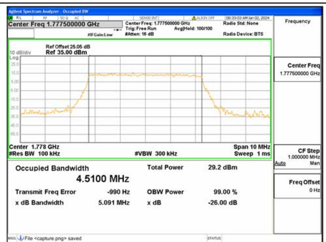
B66 / 5MHz / 16QAM/ High CH
