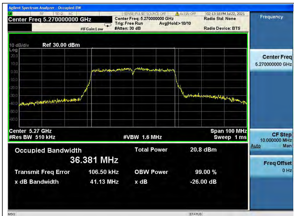
(Channel 54, 5270MHz, 802.11ac (VHT40))
