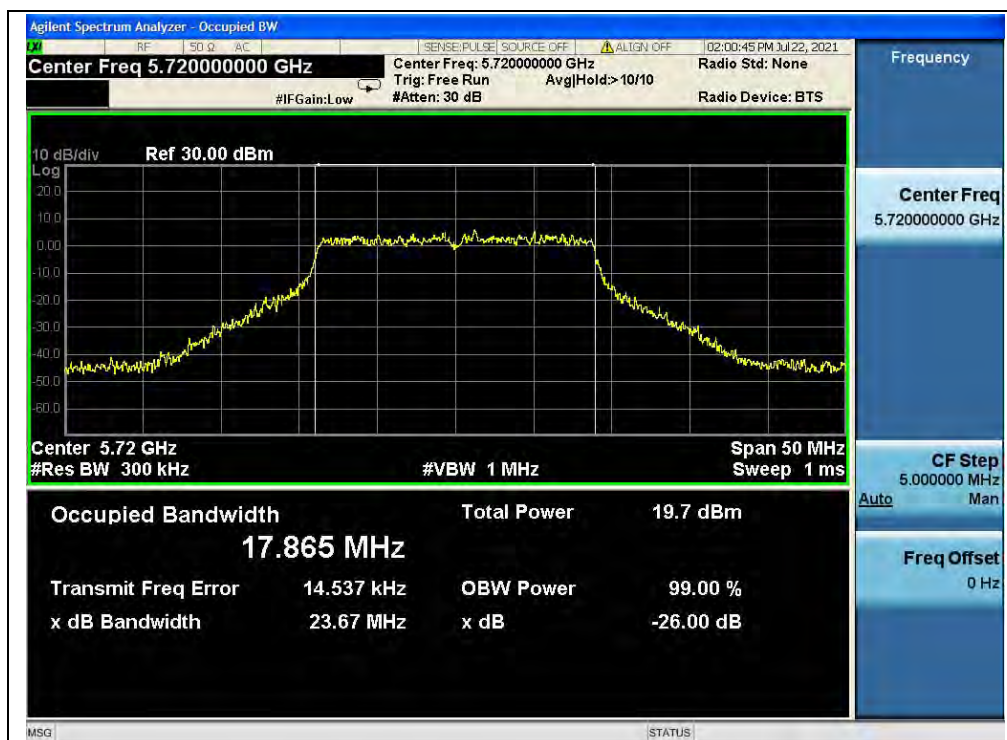
(Channel 144, 5720MHz, 802.11ac (VHT20))
