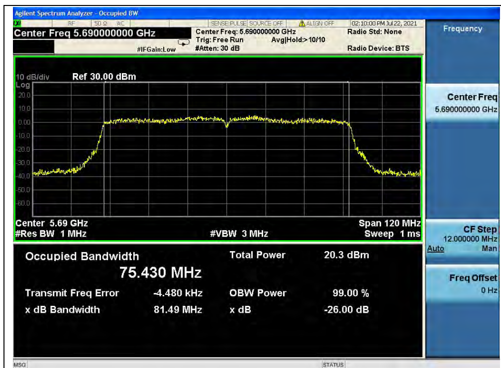
(Channel 138, 5690MHz, 802.11ac (VHT80))
