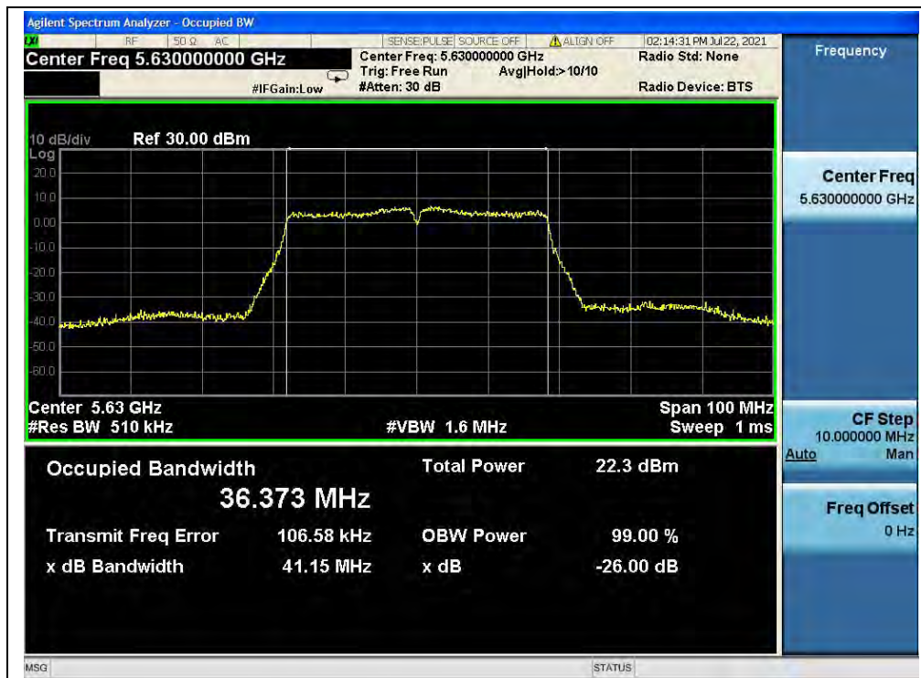
(Channel 126, 5630MHz, 802.11ac (VHT40))
