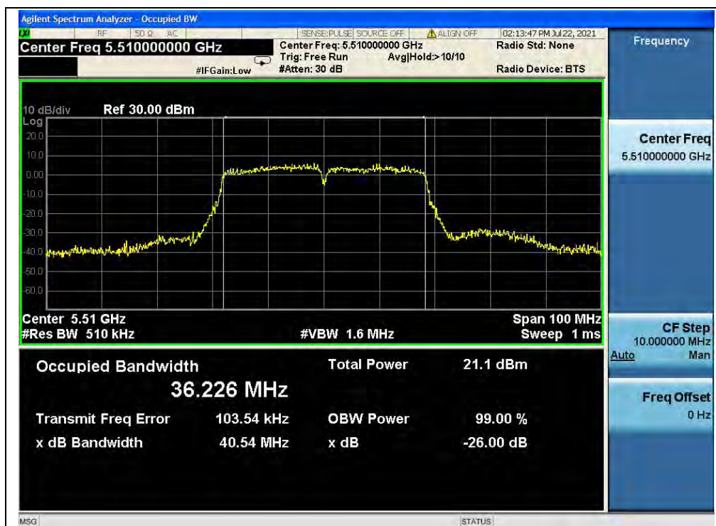
(Channel 102, 5510MHz, 802.11ac (VHT40))
