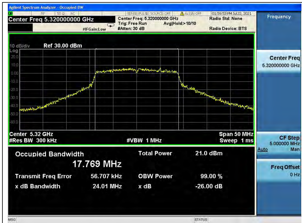
(Channel 64, 5320MHz, 802.11ac (VHT20))
