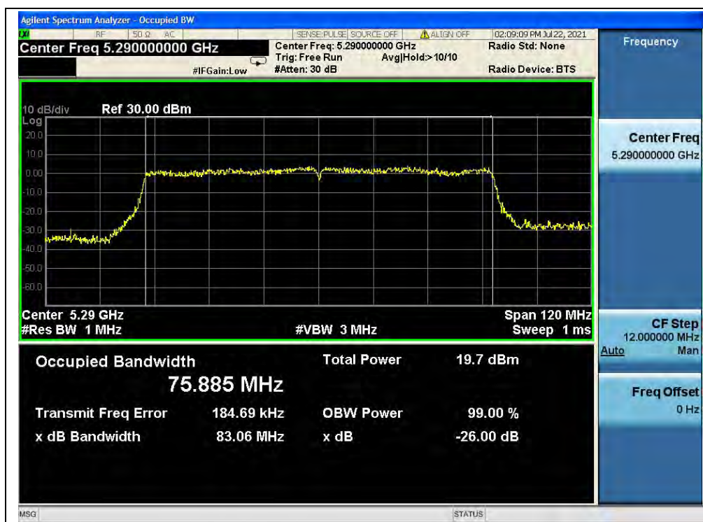
(Channel 58, 5290MHz, 802.11ac (VHT80))
