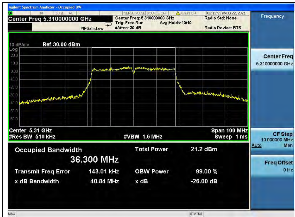
(Channel 62, 5310MHz, 802.11ac (VHT40))
