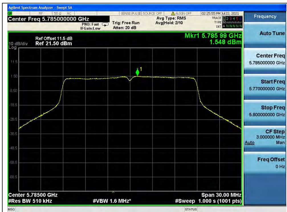
(Channel 157, 5785MHz, 802.11ac (VHT20), ANT1)
