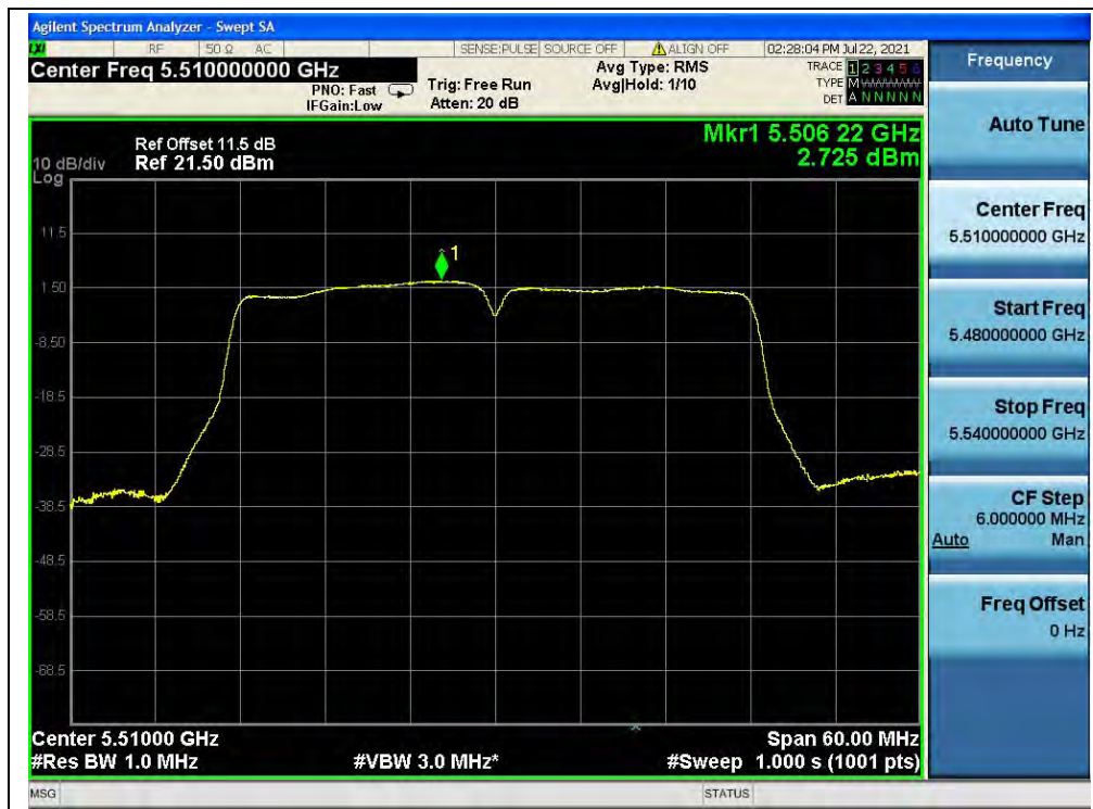
(Channel 102, 5510MHz, 802.11ac (VHT40), ANT1)
