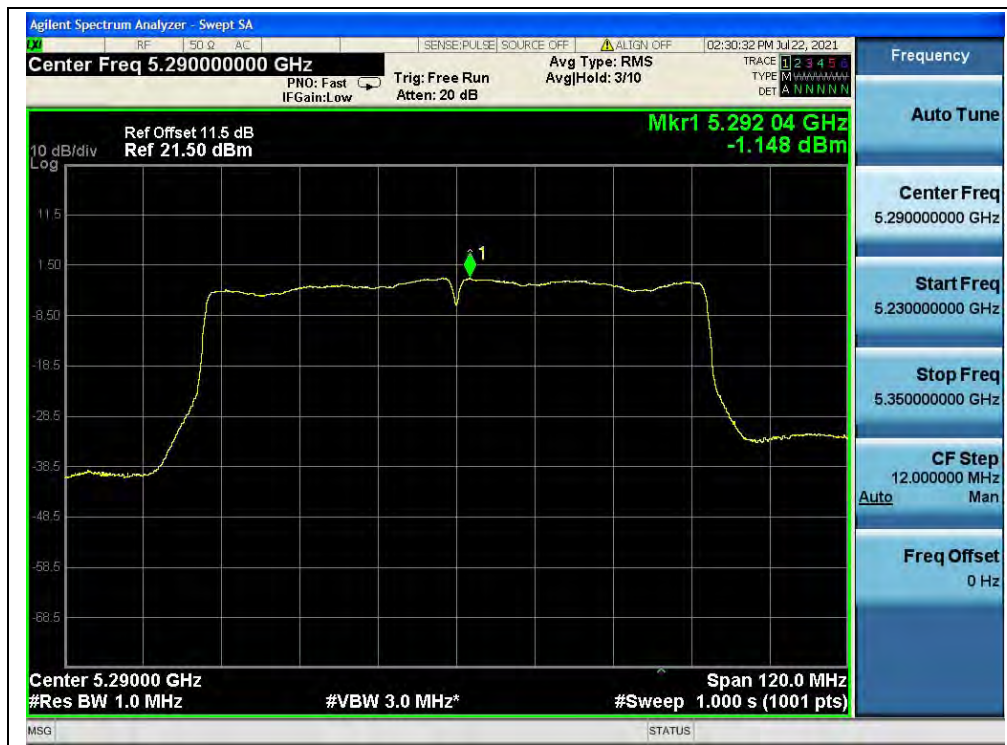
(Channel 58, 5290MHz, 802.11ac (VHT80), ANT1)
