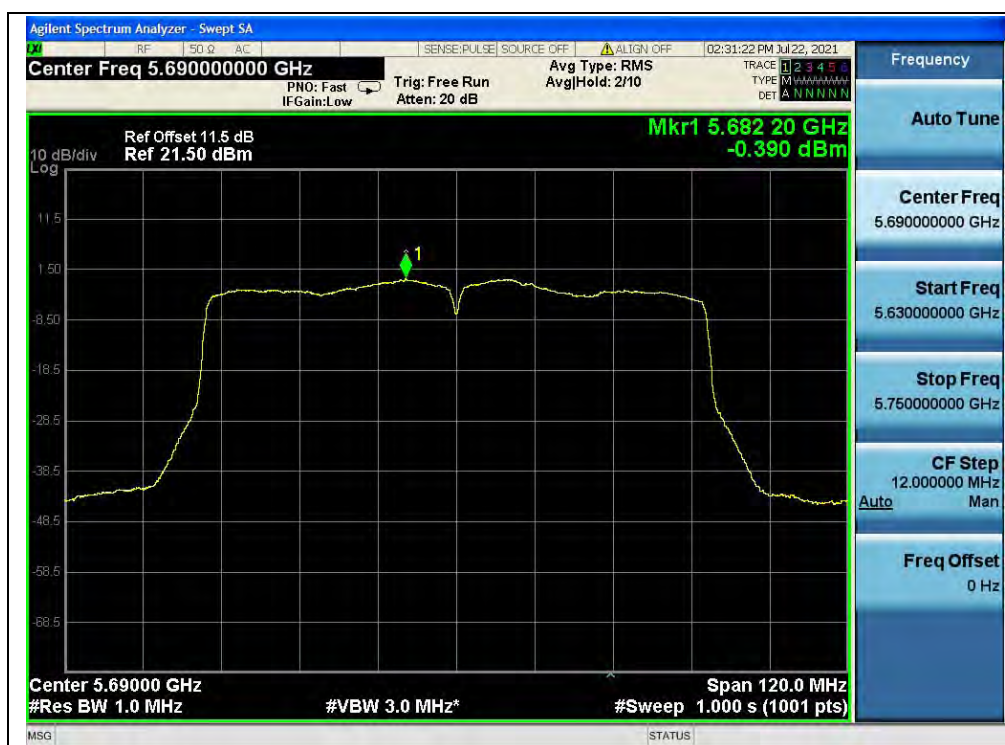
(Channel 138, 5690MHz, 802.11ac (VHT80), ANT1)
