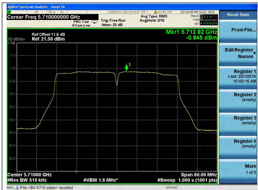
(Channel 142, 5710MHz, 802.11ac (VHT40), ANT1)
