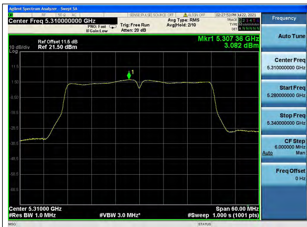
(Channel 62, 5310MHz, 802.11ac (VHT40), ANT1)
