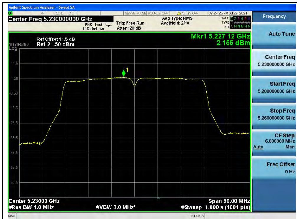
(Channel 46, 5230MHz, 802.11ac (VHT40), ANT1)
