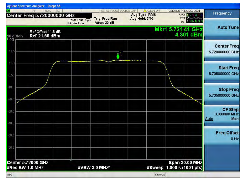
(Channel 144, 5720MHz, 802.11ac (VHT20), ANT1)
