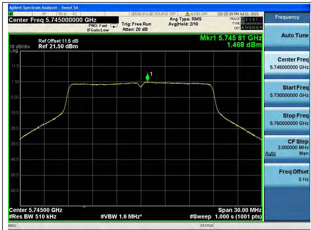
(Channel 149, 5745MHz, 802.11ac (VHT20), ANT1)
