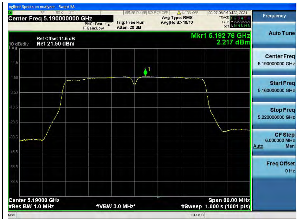
(Channel 38, 5190MHz, 802.11ac (VHT40), ANT1)
