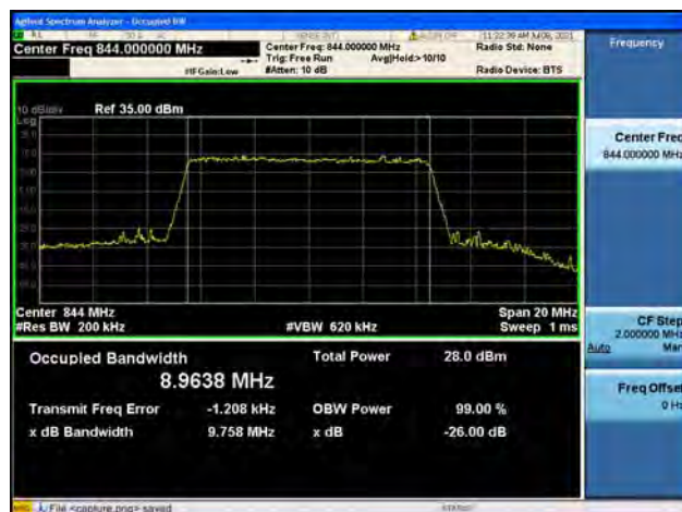
Band5 / 10MHz / High CH / 16QAM
