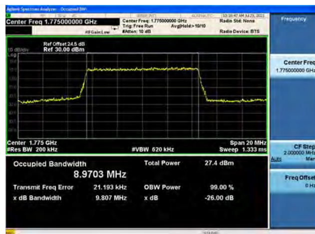
Band66 / 10MHz / High CH / 16QAM
