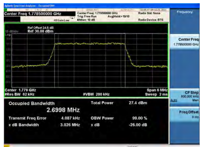
Band66 / 3MHz / High CH / 64QAM
