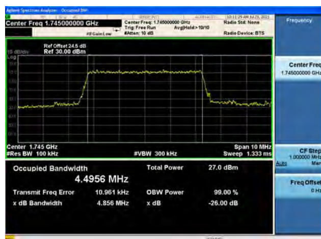
Band66 / 5MHz / Mid CH / 16QAM
