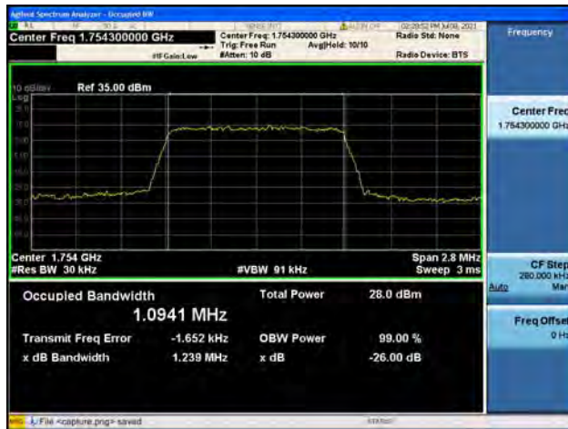
Band4 / 1.4MHz / High CH / 64QAM
