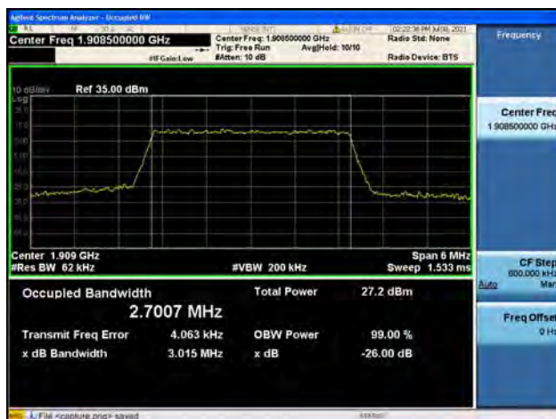
Band2 / 3MHz / High CH / 16QAM
