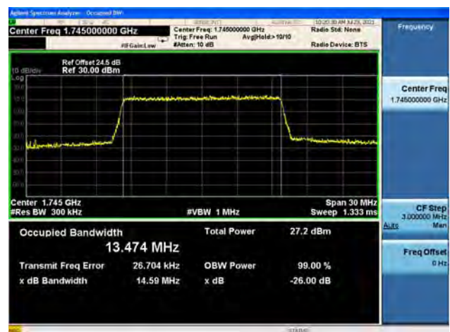
Band66 / 15MHz / Mid CH / 64QAM
