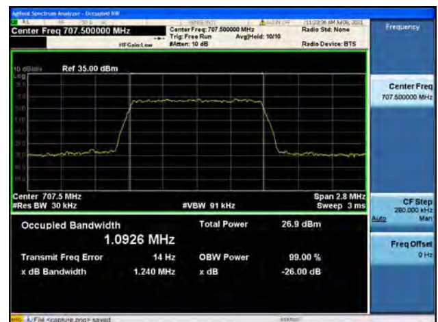
Band12 / 1.4MHz / Mid CH / 64QAM
