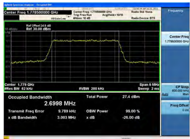
Band66 / 3MHz / High CH / 64QAM
