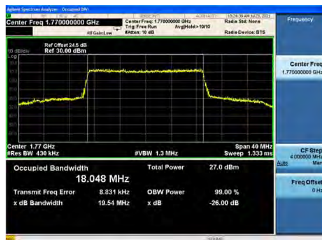
Band66 / 20MHz / High CH / 16QAM
