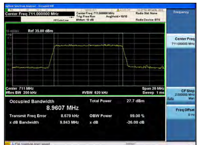
Band12 / 10MHz / High CH / 64QAM
