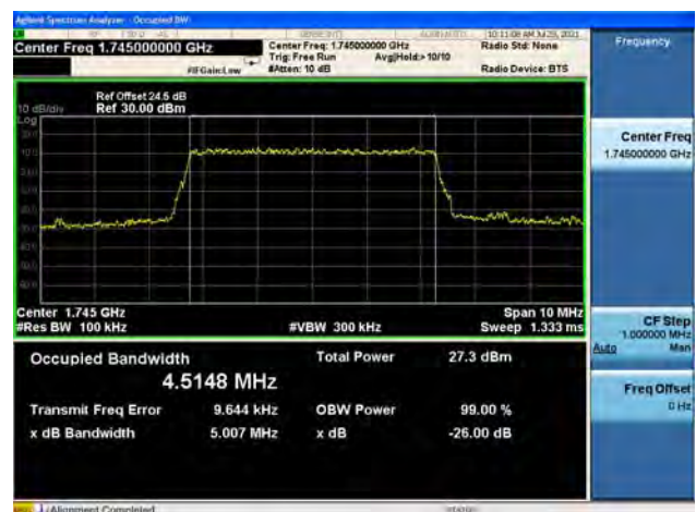
Band66 / 5MHz / Mid CH / 64QAM
