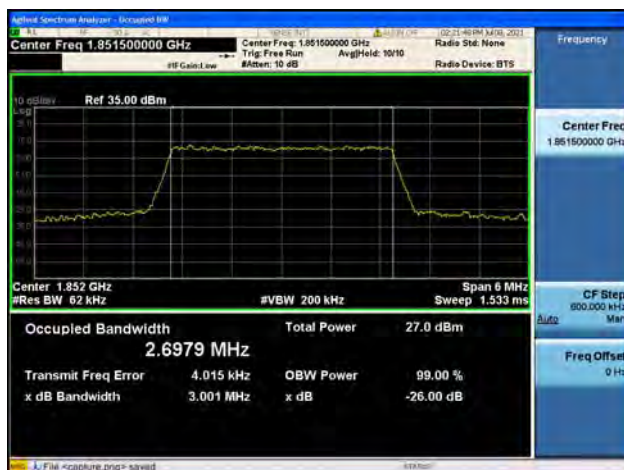
Band2 / 3MHz / Low CH / 16QAM
