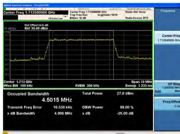
Band66 / 5MHz / Mid CH / 16QAM
