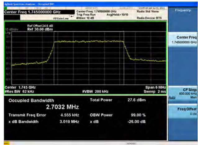
Band66 / 3MHz / High CH / QPSK
