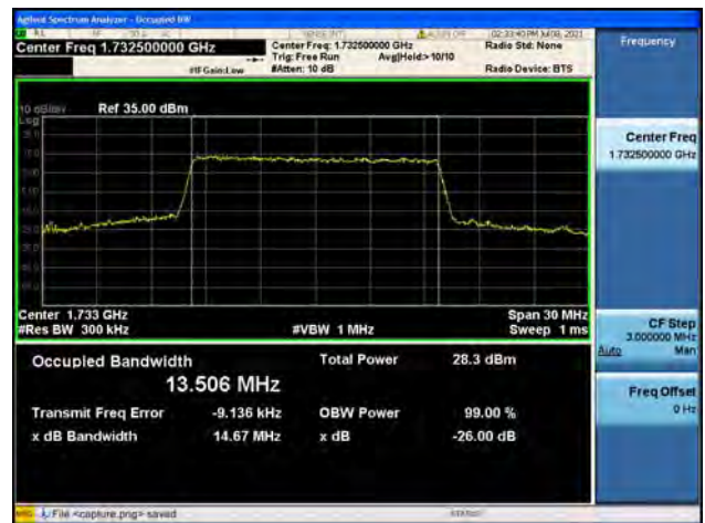
Band4 / 15MHz / Mid CH / 64QAM
