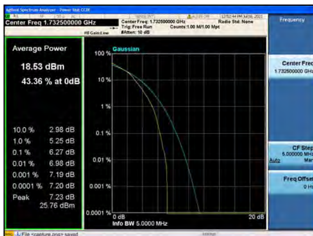
Band4 / 1.4MHz / Mid CH / 16QAM
