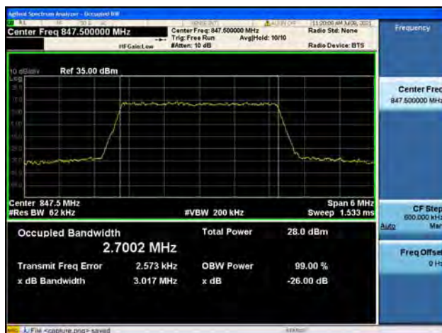
Band5 / 3MHz / High CH / 16QAM
