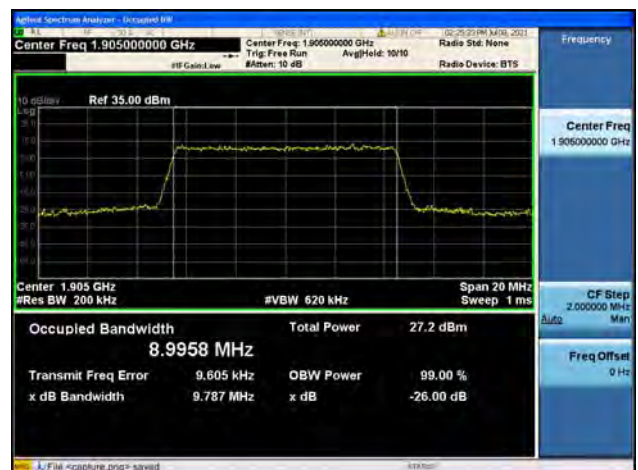
Band2 / 10MHz / High CH / 64QAM
