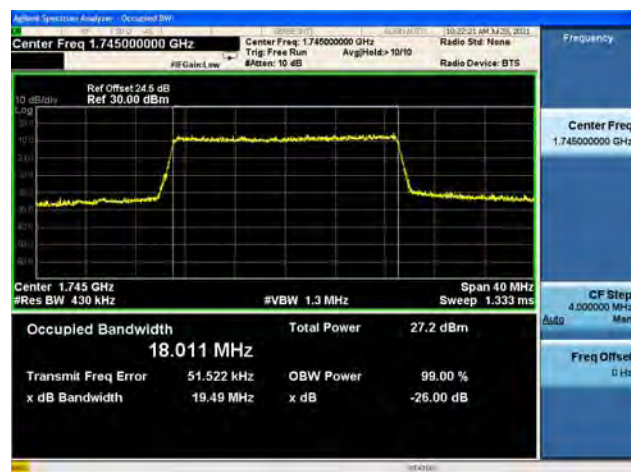
Band66 / 20MHz / High CH / 16QAM
