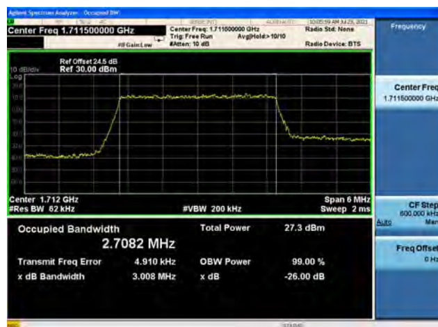
Band66 / 3MHz / Low CH / 16QAM
