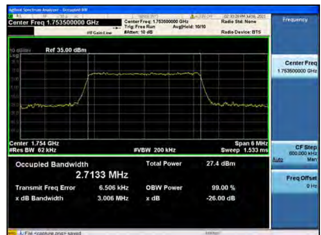
Band4 / 3MHz / High CH / 64QAM
