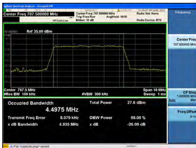
Band12 / 5MHz / Mid CH / 16QAM
