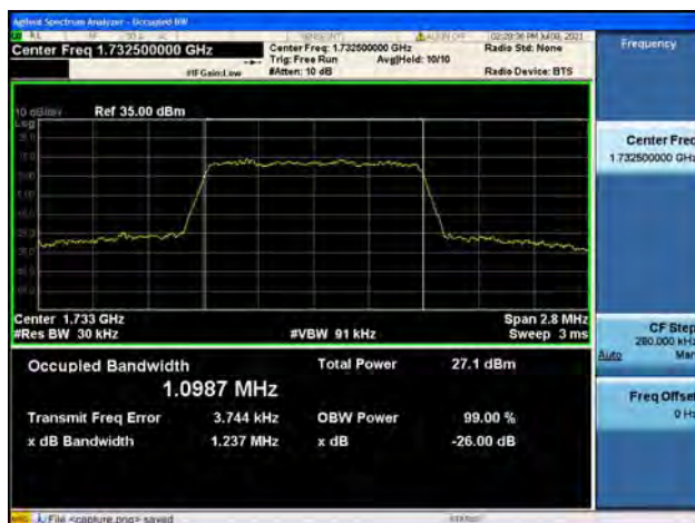
Band4 / 1.4MHz / Mid CH / 16QAM
