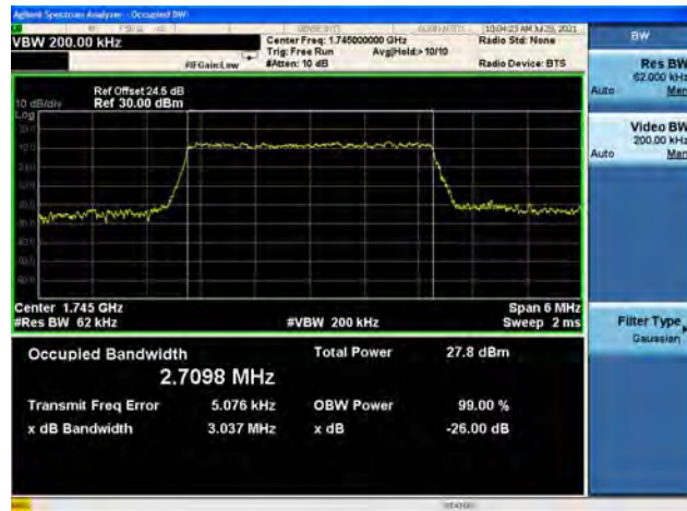
Band66 / 3MHz / Mid CH / 64QAM
