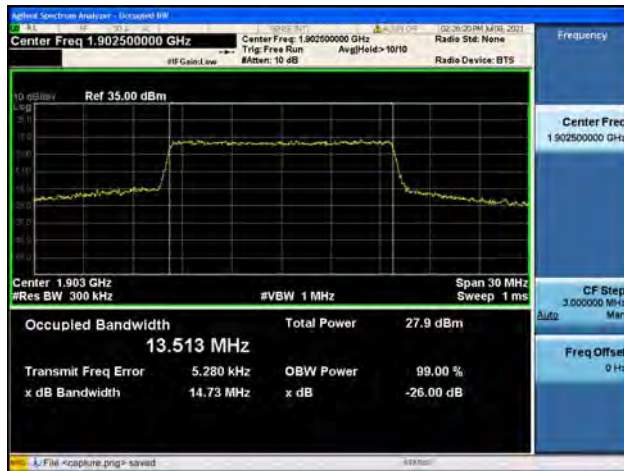
Band2 / 15MHz / High CH / 64QAM
