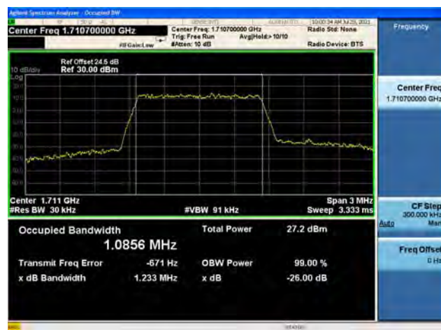
Band66 / 1.4MHz / Mid CH / 16QAM
