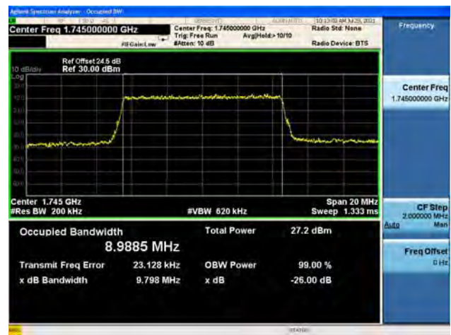
Band66 / 10MHz / High CH / QPSK
