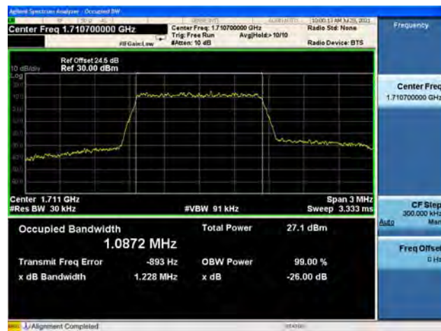
Band66 / 1.4MHz / Low CH / 64QAM
