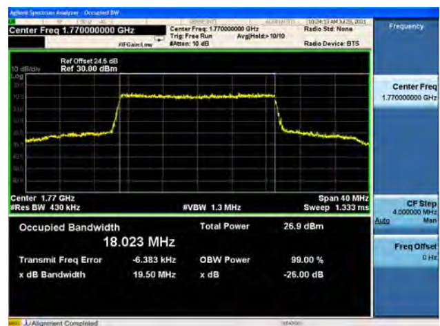
Band66 / 20MHz / High CH / 64QAM
