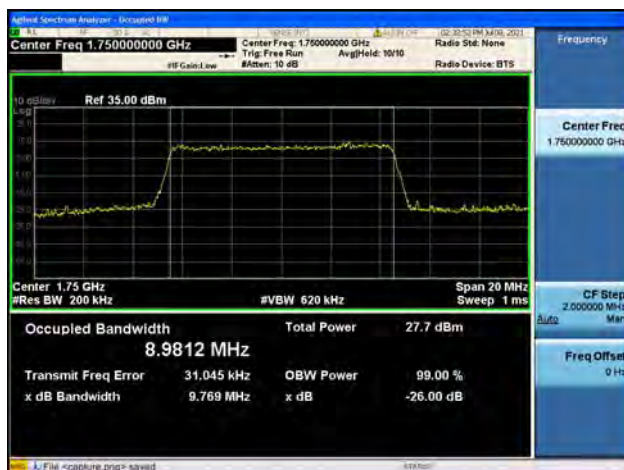
Band4 / 10MHz / High CH / 16QAM
