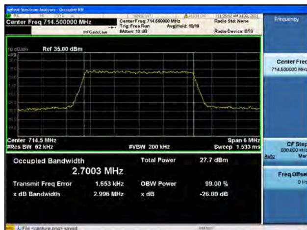
Band12 / 3MHz / High CH / 16QAM
