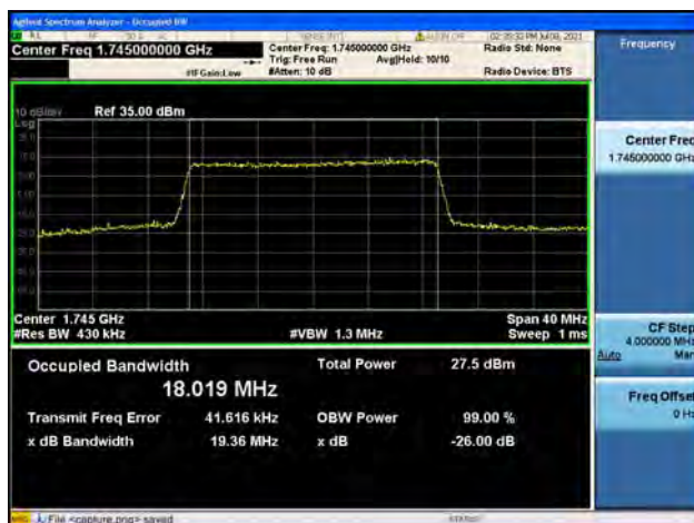
Band4 / 20MHz / High CH / 16QAM
