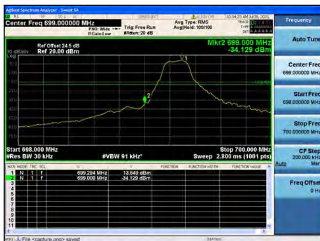
Band12 / 1.4MHz / Low CH / QPSK / 1 RB
