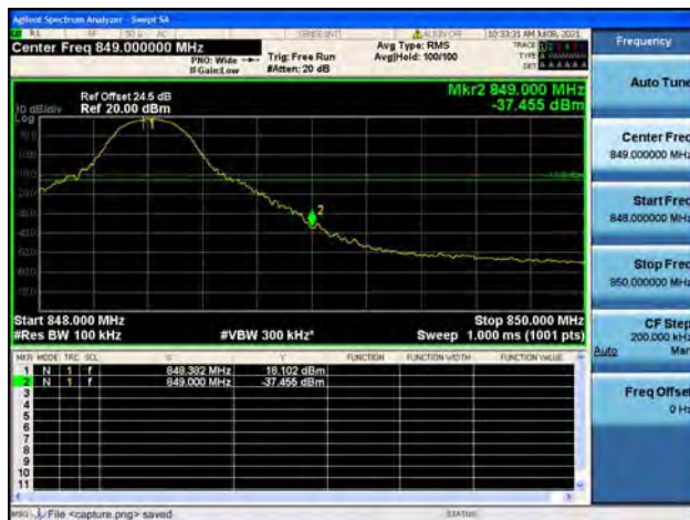
Band12 / 1.4MHz / Low CH / QPSK / 1 RB
