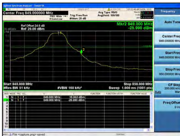
Band5 / 5MHz / High CH / QPSK / 1 RB
