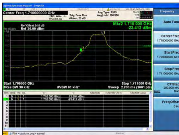
Band4 / 3MHz / Low CH / QPSK / 1 RB
