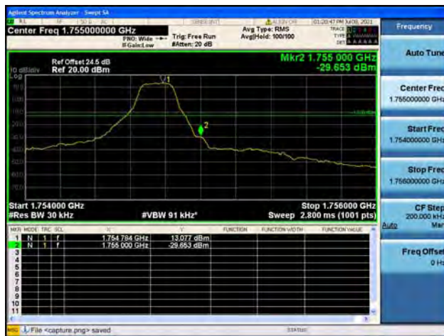
Band4 / 3MHz / Low CH / QPSK / 1 RB
