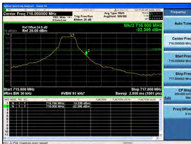
Band12 / 3MHz / High CH / QPSK / 1 RB
