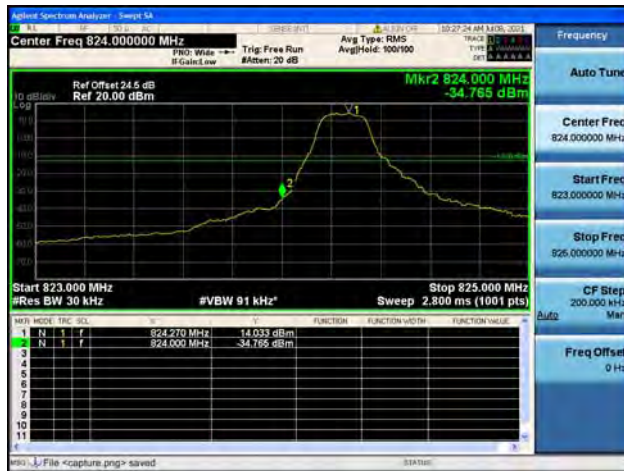
Band5 / 1.4MHz / High CH / QPSK / 1 RB
