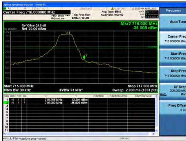
Band12 / 3MHz / Low CH / QPSK / 1 RB
