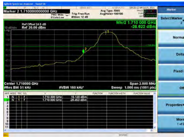
Band66 / 5MHz / High CH / QPSK / 1 RB
