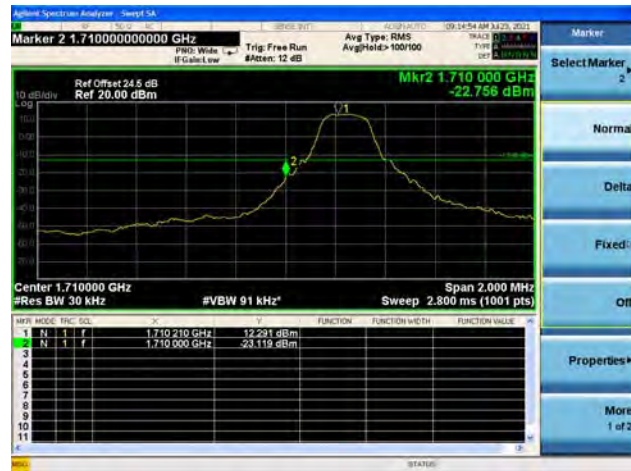
Band66 / 3MHz / High CH / QPSK / 1 RB
