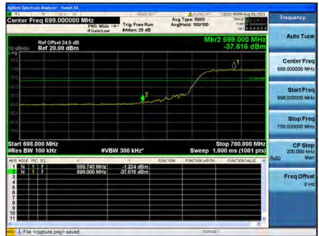
Band12 / 10MHz / High CH / QPSK / FULL RB
