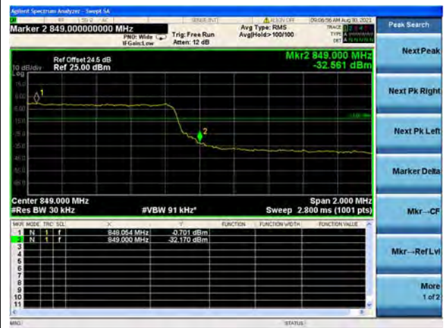
Band26 / 3MHz / High CH / QPSK / FULL RB
