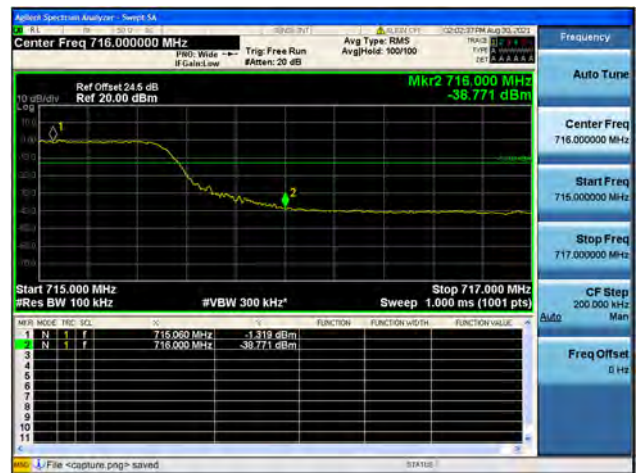
Band12 / 10MHz / High CH / QPSK / FULL RB
