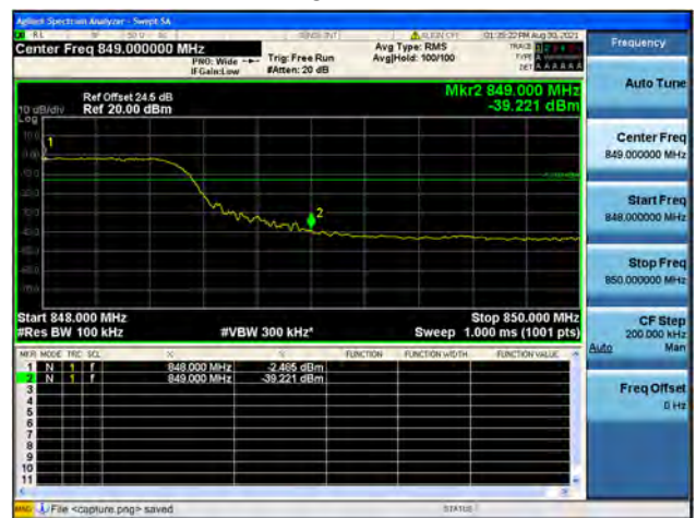
Band5 / 10MHz / High CH / QPSK / FULL RB
