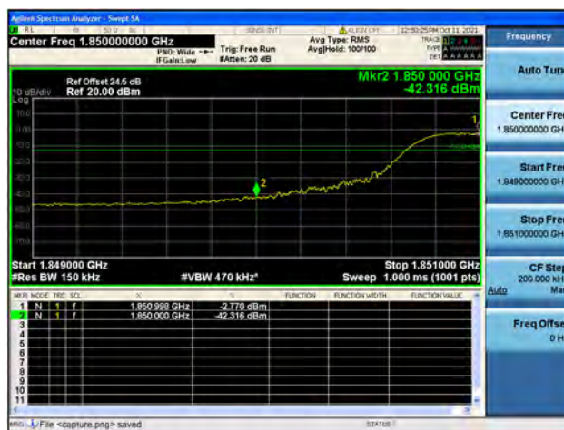
Band25 / 15MHz / High CH / QPSK / FULL RB
