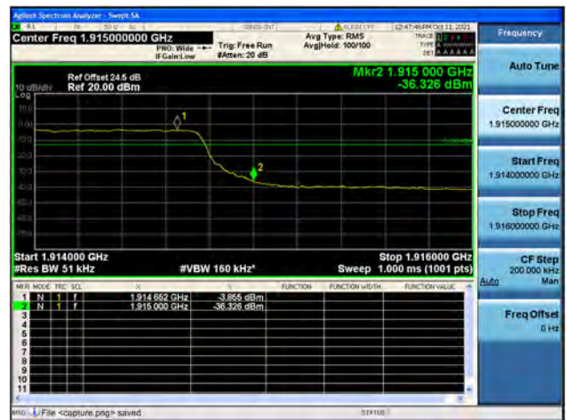
Band25 / 5MHz / High CH / QPSK / FULL RB
