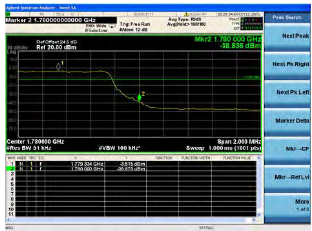
Band66 / 5MHz / High CH / QPSK / FULL RB
