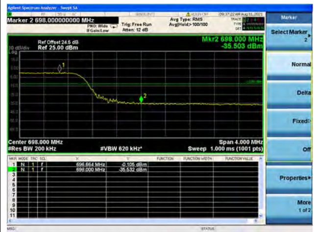
Band71 / 20MHz / High CH / QPSK / FULL RB
