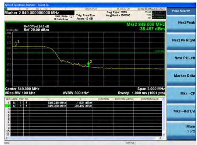
Band26 / 10MHz / High CH / QPSK / FULL RB
