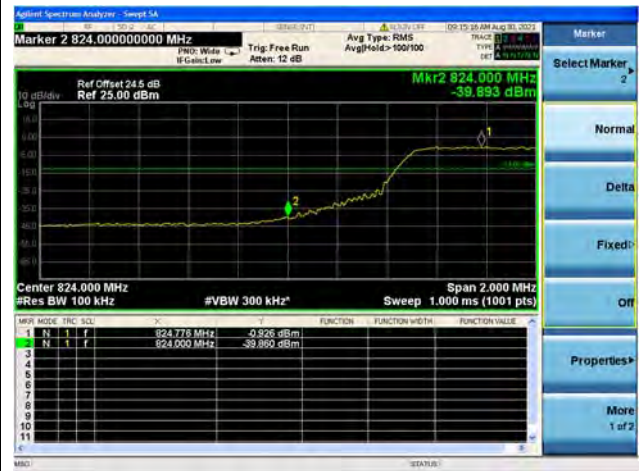
Band26 / 10MHz / High CH / QPSK / FULL RB
