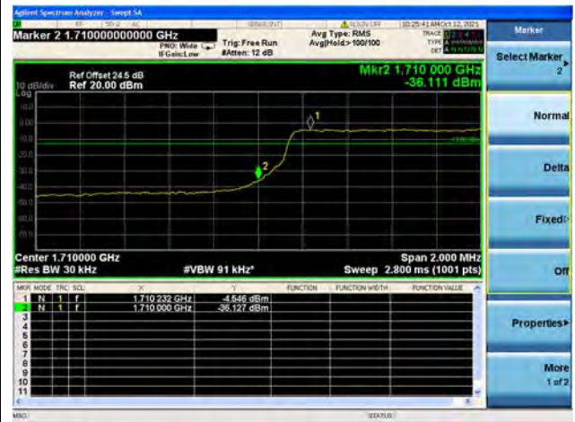
Band66 / 3MHz / High CH / QPSK / FULL RB
