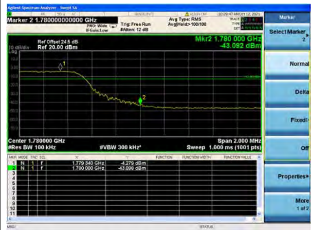
Band66 / 10MHz / High CH / QPSK / FULL RB
