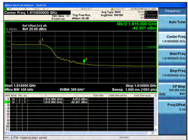
Band25 / 10MHz / High CH / QPSK / FULL RB
