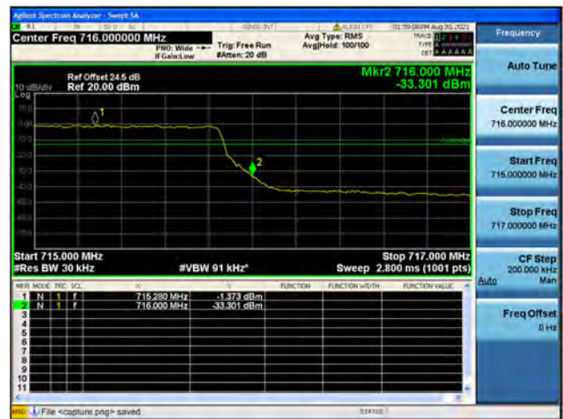
Band12 / 3MHz / High CH / QPSK / FULL RB
