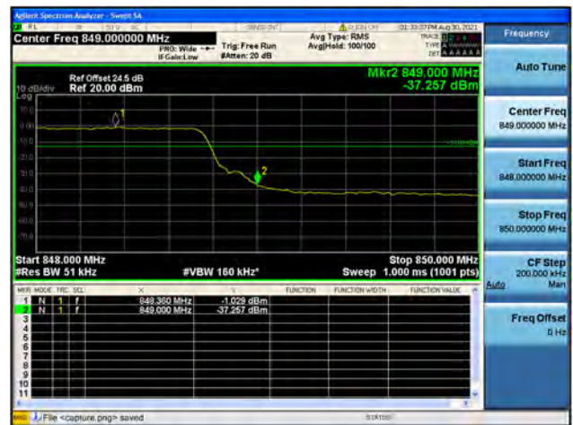
Band5 / 5MHz / High CH / QPSK / FULL RB
