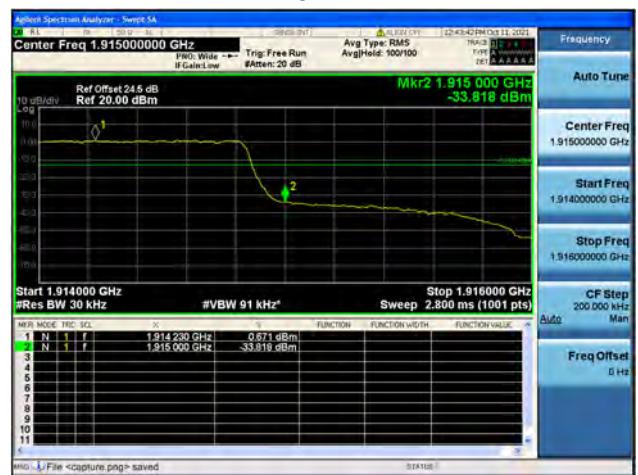
Band25 / 1.4MHz / High CH / QPSK / FULL RB
