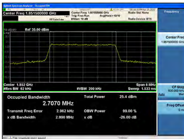
Band2 / 3MHz / Low CH / 16QAM
