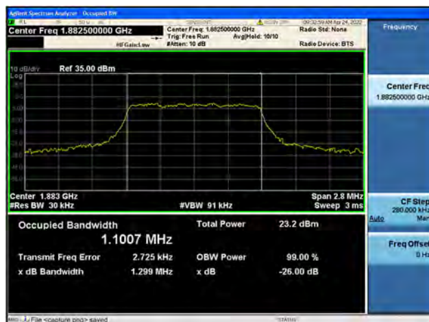
Band25 / 1.4MHz / Mid CH / 16QAM
