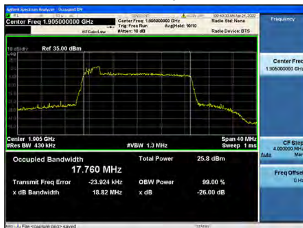
Band25 / 20MHz / High CH / 16QAM
