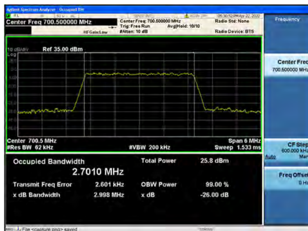
Band12 / 3MHz / Low CH / 16QAM
