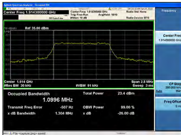
Band25 / 3MHz / Low CH / 16QAM
