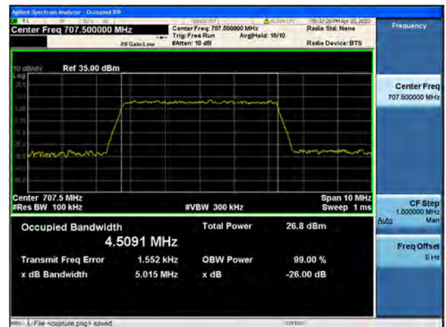
Band12 / 5MHz / Mid CH / 64QAM
