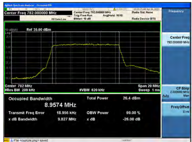
Band13 / 10MHz / High CH / 64QAM
