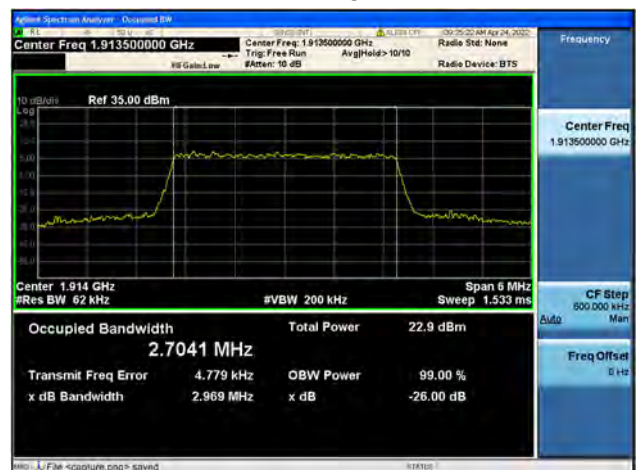
Band25 / 3MHz / High CH / 64QAM
