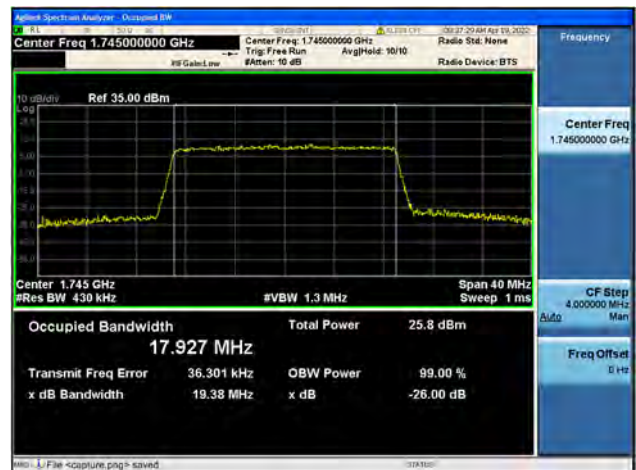
Band4 / 20MHz / High CH / 64QAM
