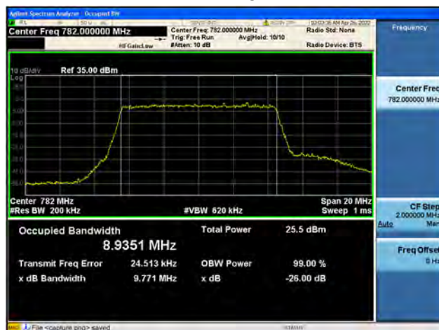
Band13 / 10MHz / High CH / 16QAM
