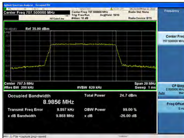
Band12 / 10MHz / High CH / 16QAM
