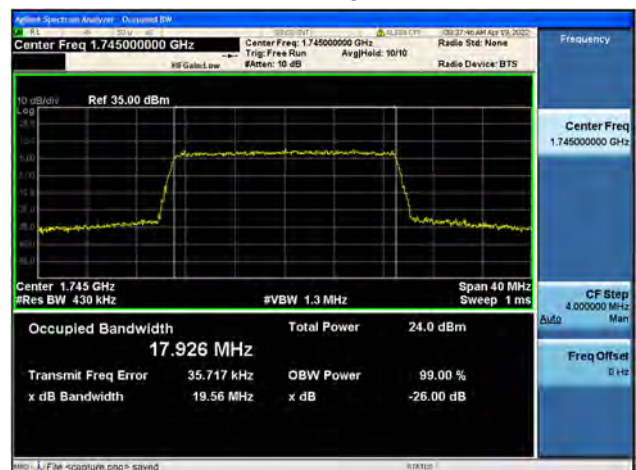
Band4 / 20MHz / High CH / 64QAM
