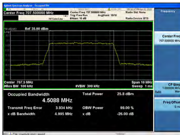
Band12 / 5MHz / Mid CH / 16QAM
