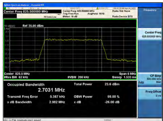
Band26Part22 / 3MHz / Low CH / 64QAM
