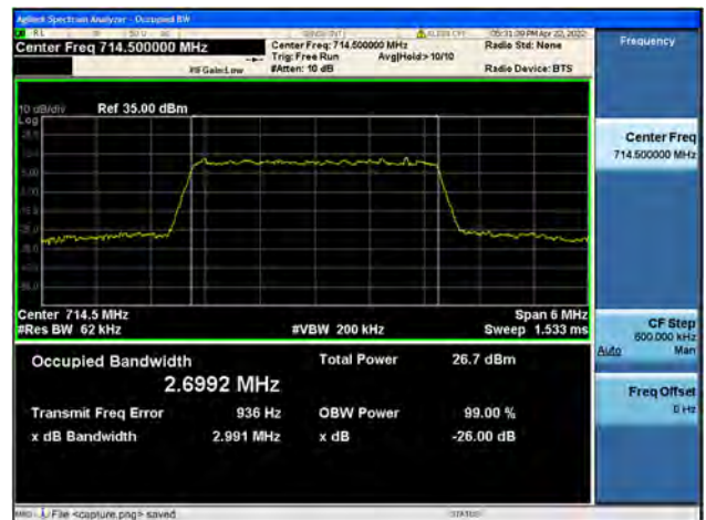
Band12 / 3MHz / High CH / 64QAM
