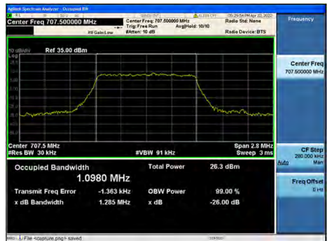
Band12 / 1.4MHz / Mid CH / 64QAM
