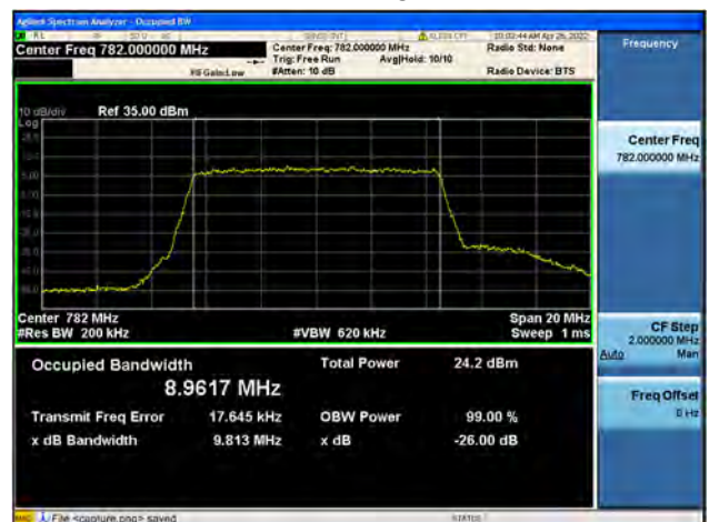
Band13 / 10MHz / High CH / 64QAM
