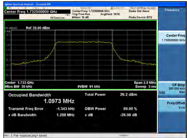
Band4 / 1.4MHz / Mid CH / 64QAM
