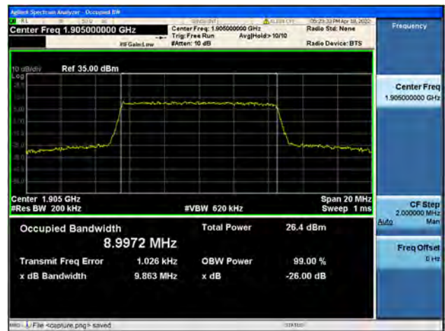
Band2 / 10MHz / High CH / 64QAM
