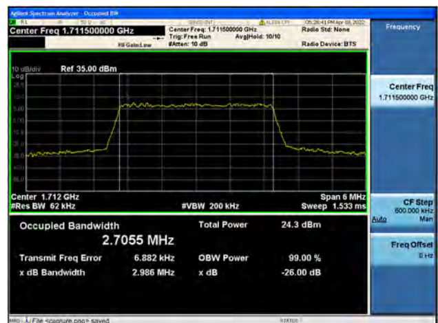
Band4 / 3MHz / Low CH / 64QAM
