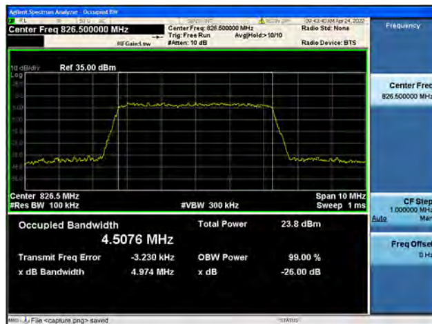
Band26Part22 / 5MHz / Mid CH / 16QAM
