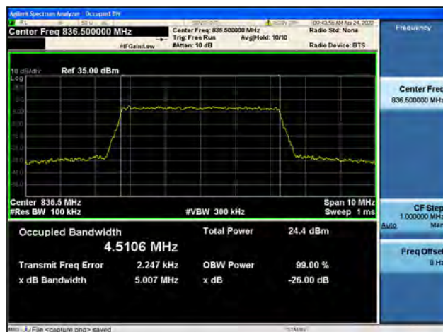
Band26Part22 / 5MHz / Mid CH / 16QAM
