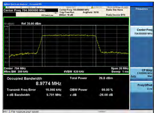
Band12 / 10MHz / Low CH / 64QAM
