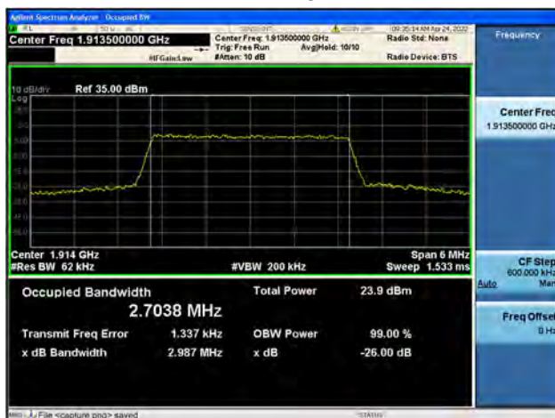
Band25 / 3MHz / High CH / 16QAM
