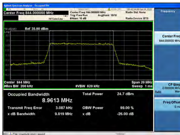
Band26Part22 / 10MHz / High CH / 16QAM
