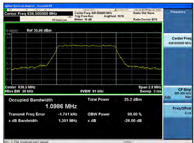
Band5 / 1.4MHz / Mid CH / 64QAM
