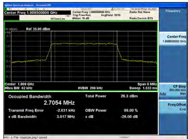
Band2 / 3MHz / High CH / 64QAM
