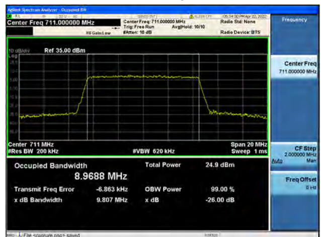
Band12 / 10MHz / High CH / 64QAM
