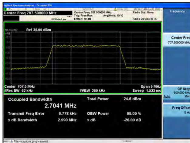
Band12 / 3MHz / High CH / 16QAM
