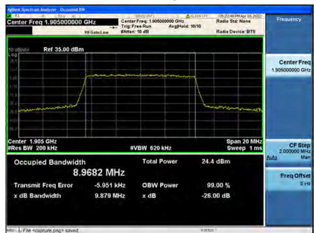
Band2 / 10MHz / High CH / 64QAM
