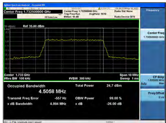
Band4 / 5MHz / Mid CH / 64QAM
