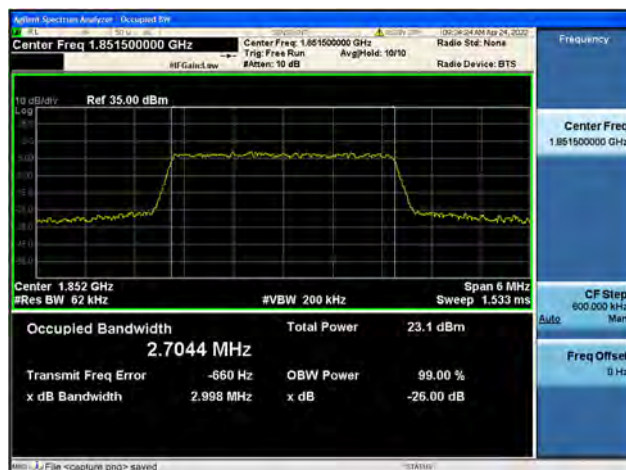
Band25 / 3MHz / Low CH / 16QAM
