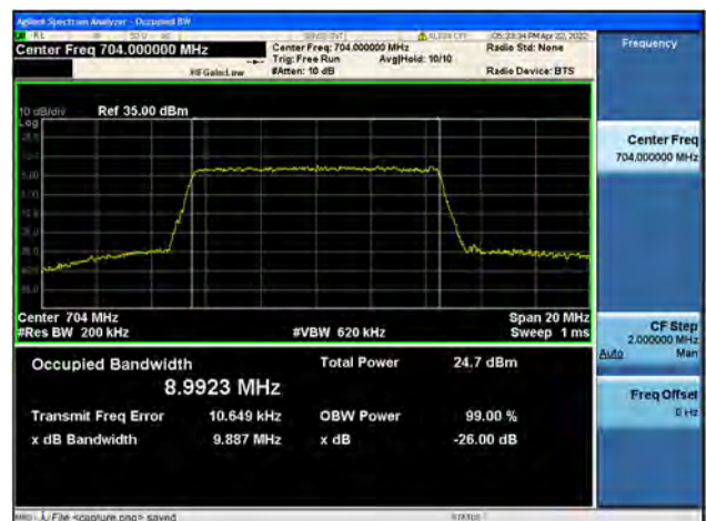
Band12 / 10MHz / Low CH / 64QAM
