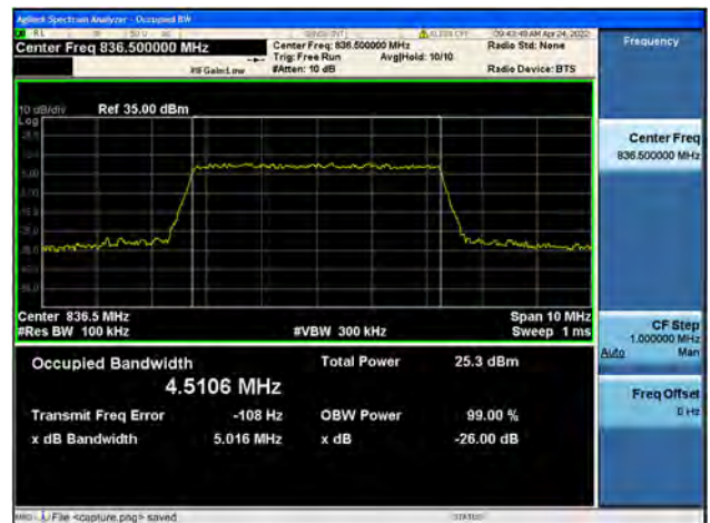
Band26Part22 / 5MHz / Mid CH / 64QAM
