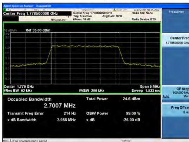
Band66 / 3MHz / High CH / 16QAM
