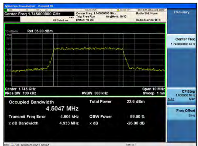
Band66 / 5MHz / Mid CH / 64QAM
