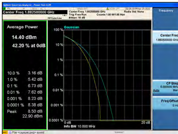
Band25 / 10MHz / High CH / 16QAM
