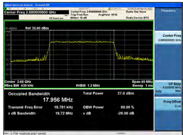
Band41 / 20MHz / High CH / 64QAM
