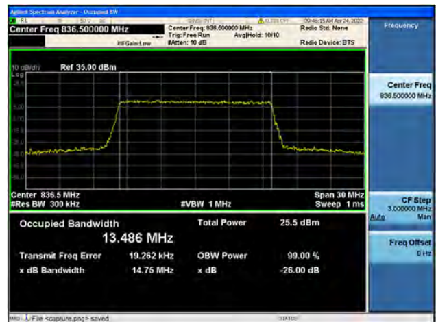
Band26Part22 / 15MHz / Mid CH / 64QAM
