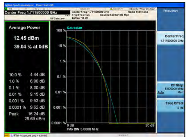
Band4 / 3MHz / Low CH / 64QAM
