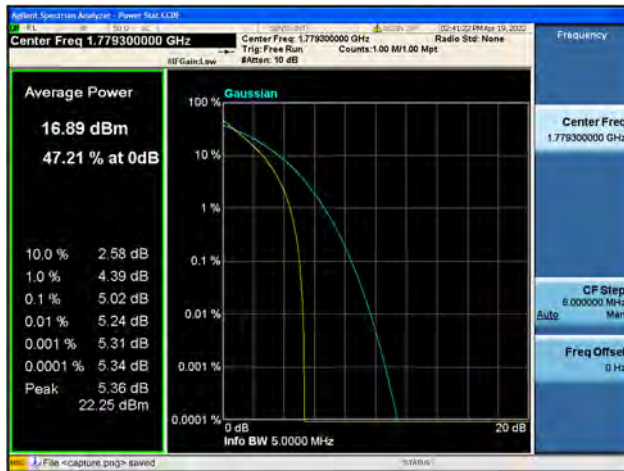
Band66 / 1.4MHz / High CH / 64QAM
