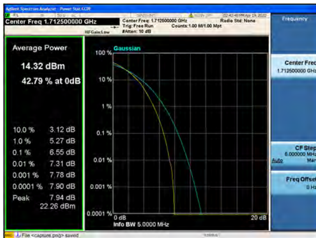
Band66 / 5MHz / Mid CH / 16QAM
