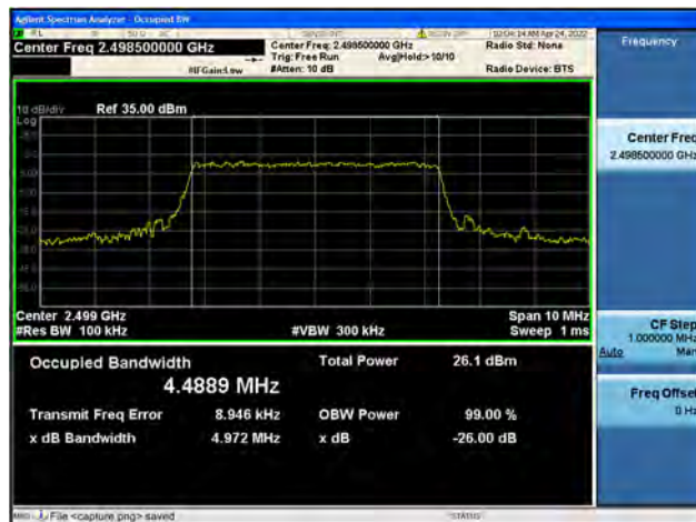
Band41 / 5MHz / Mid CH / 16QAM
