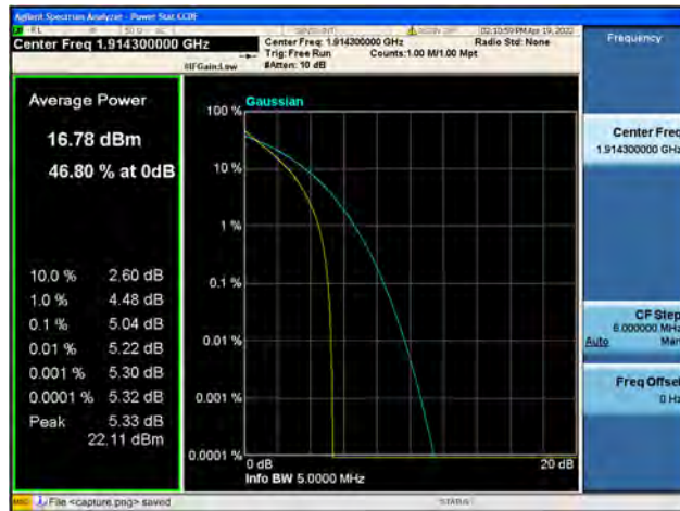
Band25 / 1.4MHz / High CH / 64QAM
