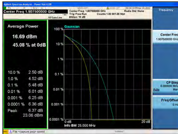
Band25 / 15MHz / High CH / 64QAM
