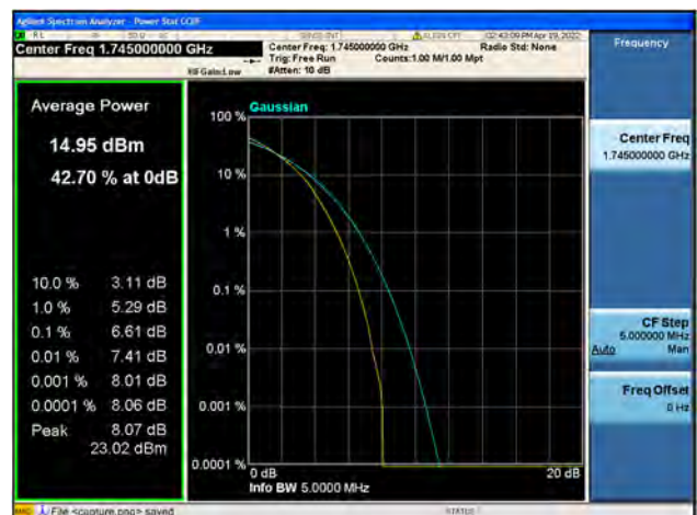
Band66 / 5MHz / Mid CH / 64QAM
