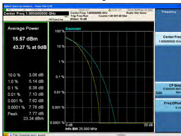
Band25 / 20MHz / High CH / 16QAM
