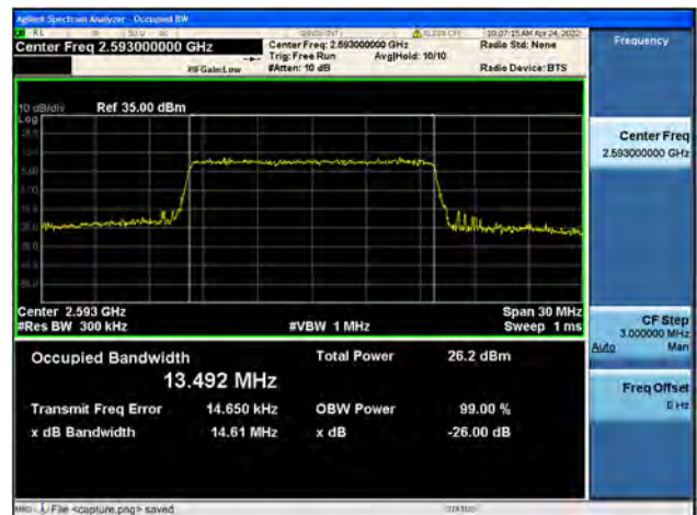
Band41 / 15MHz / Mid CH / 64QAM
