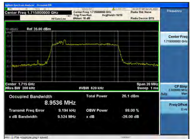
Band66 / 10MHz / Low CH / 64QAM
