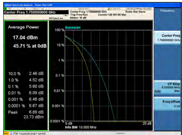
Band4 / 10MHz / High CH / 64QAM
