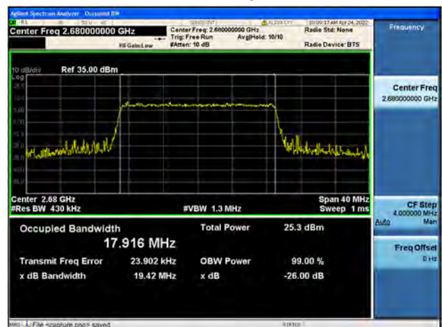
Band41 / 20MHz / High CH / 64QAM
