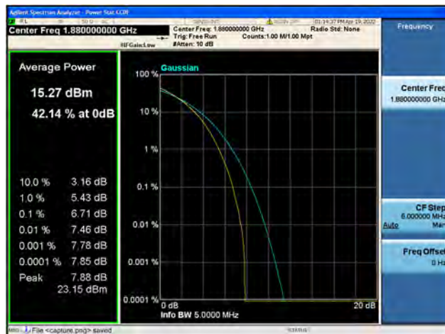
Band2 / 3MHz / High CH / 16QAM
