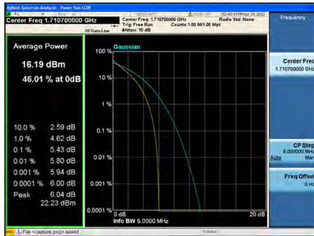
Band66 / 1.4MHz / Low CH / 64QAM
