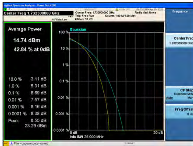
Band4 / 20MHz / High CH / 16QAM
