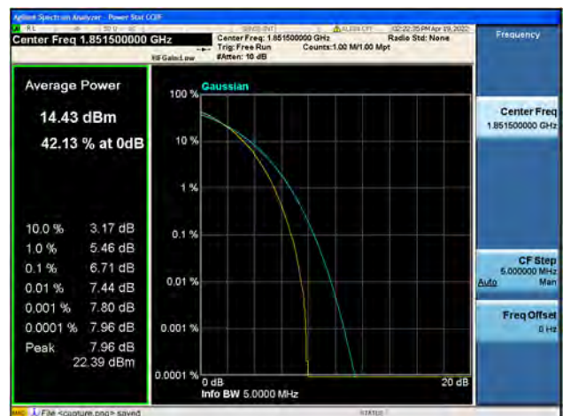
Band25 / 3MHz / Low CH / 64QAM
