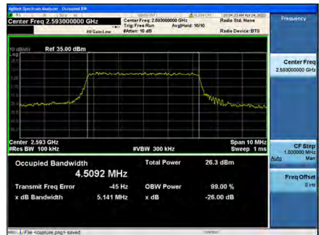
Band41 / 5MHz / Mid CH / 64QAM
