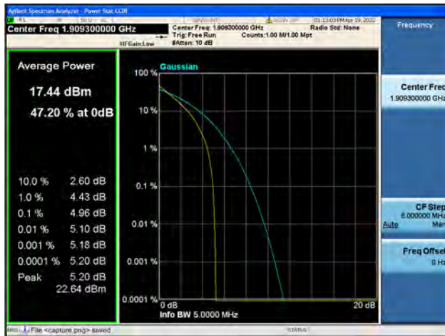
Band2 / 1.4MHz / High CH / 64QAM
