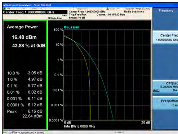
Band2 / 3MHz / Low CH / 16QAM
