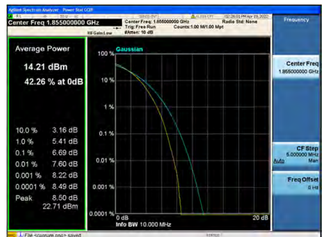
Band25 / 10MHz / Low CH / 64QAM
