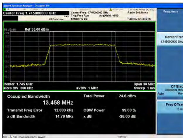
Band66 / 15MHz / Mid CH / 16QAM
