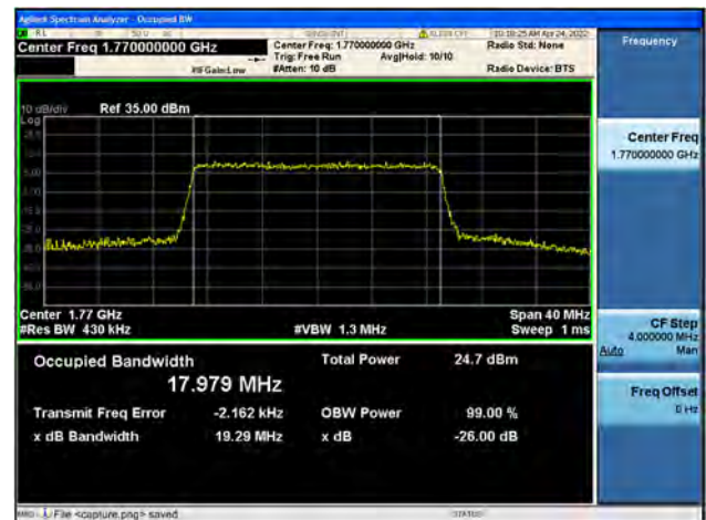
Band66 / 20MHz / High CH / 64QAM
