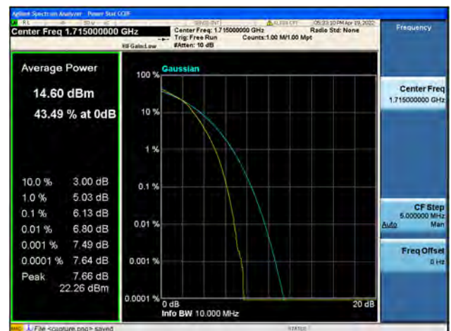
Band66 / 10MHz / Low CH / 64QAM
