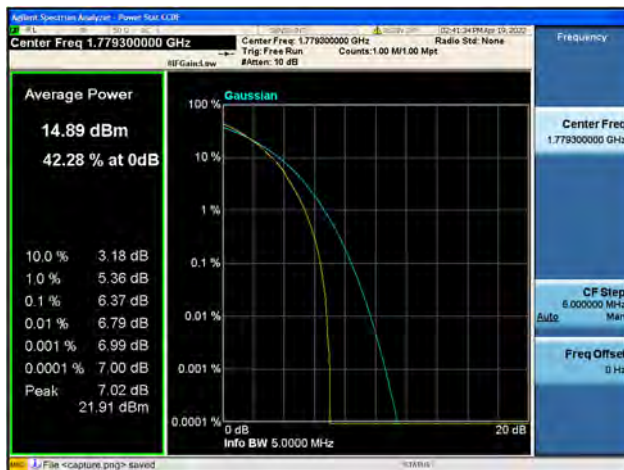
Band66 / 3MHz / Low CH / 16QAM
