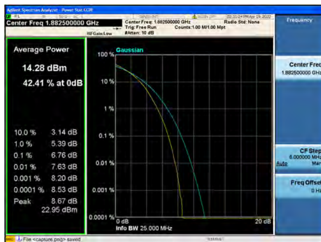
Band25 / 20MHz / High CH / 16QAM
