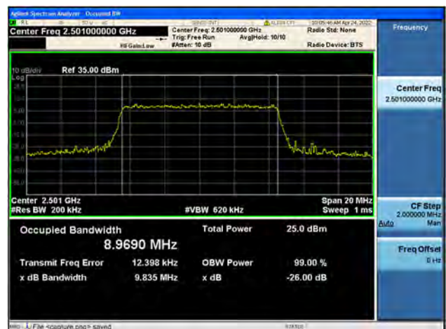
Band41 / 10MHz / Low CH / 64QAM
