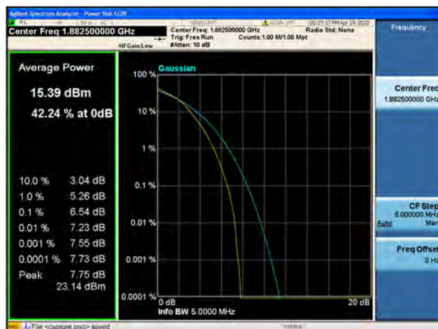
Band25 / 5MHz / Mid CH / 16QAM
