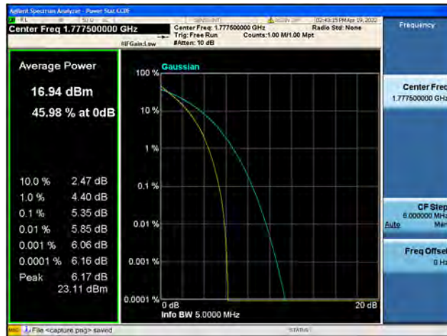
Band66 / 5MHz / High CH / 64QAM
