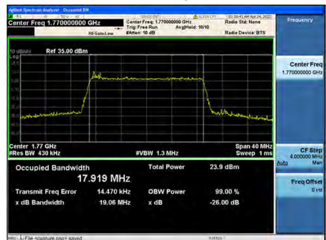
Band66 / 20MHz / High CH / 64QAM
