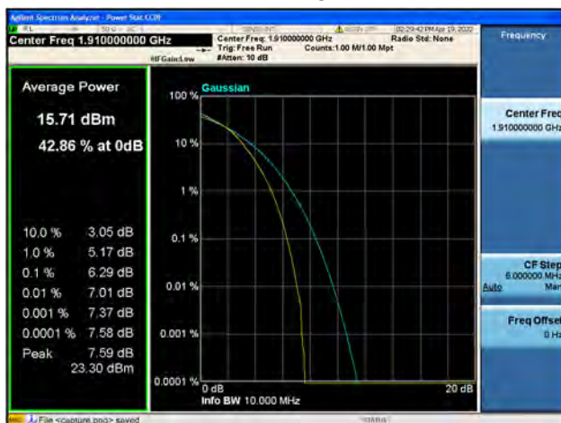
Band25 / 10MHz / High CH / 16QAM
