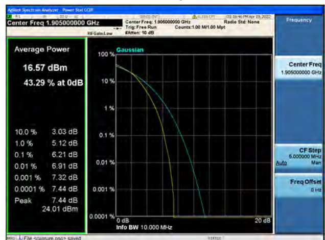
Band2 / 10MHz / High CH / 64QAM
