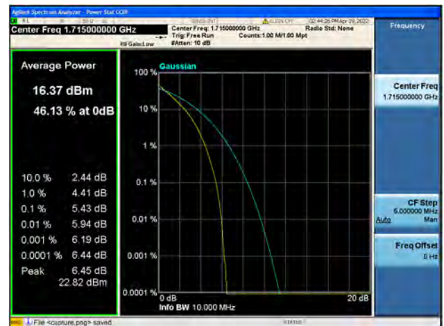
Band66 / 10MHz / Low CH / 64QAM
