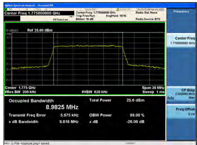
Band66 / 10MHz / High CH / 64QAM
