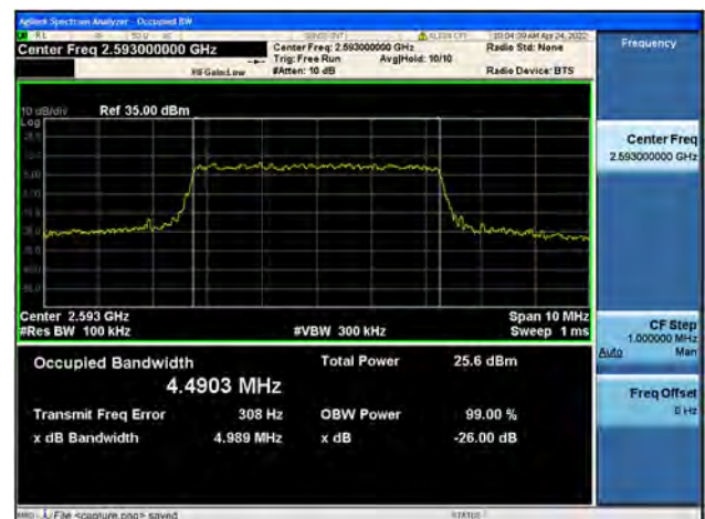
Band41 / 5MHz / Mid CH / 64QAM
