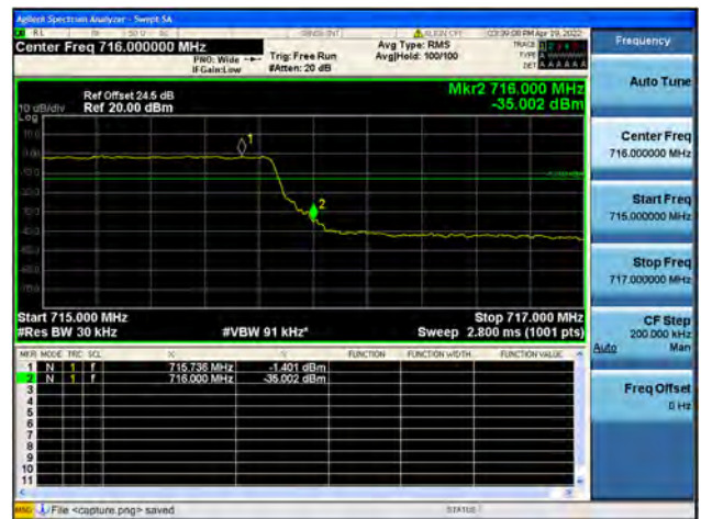
Band12 / 3MHz / High CH / QPSK / FULL RB
