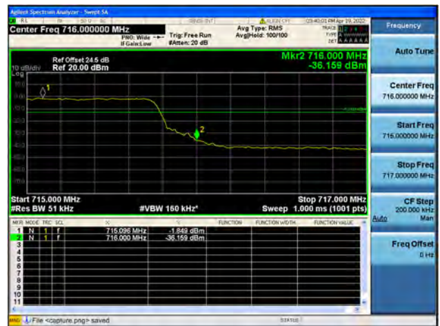
Band12 / 5MHz / High CH / QPSK / FULL RB
