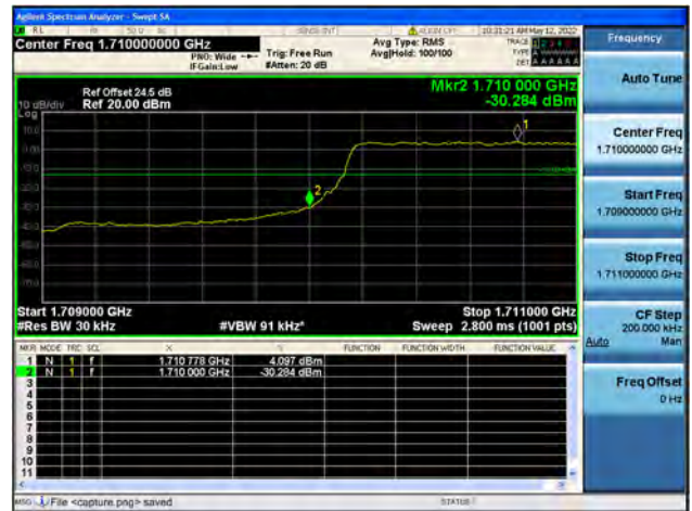
Band66 / 1.4MHz / High CH / QPSK / FULL RB
