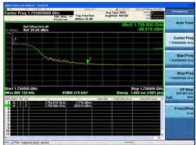
Band4 / 15MHz / High CH / QPSK / FULL RB
