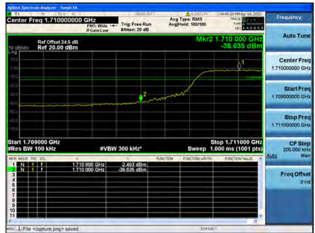
Band4 / 10MHz / High CH / QPSK / FULL RB
