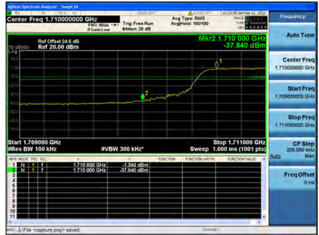
Band66 / 10MHz / High CH / QPSK / FULL RB
