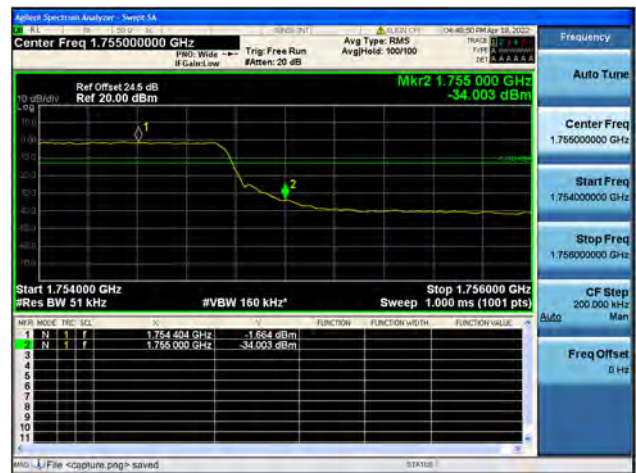
Band4 / 5MHz / High CH / QPSK / FULL RB
