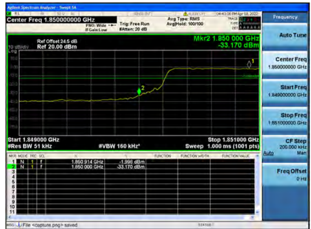
Band2 / 5MHz / High CH / QPSK / FULL RB
