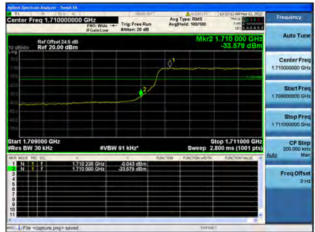
Band66 / 3MHz / High CH / QPSK / FULL RB
