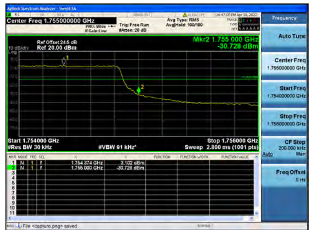
Band4 / 1.4MHz / High CH / QPSK / FULL RB
