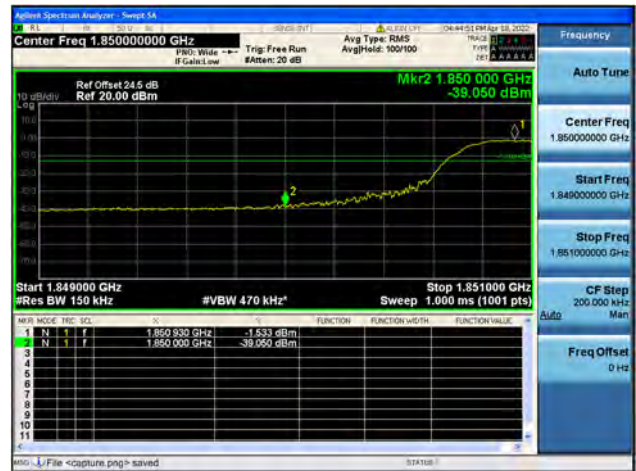
Band2 / 15MHz / High CH / QPSK / FULL RB
