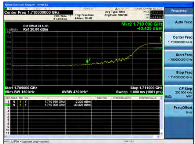
Band4 / 15MHz / High CH / QPSK / FULL RB
