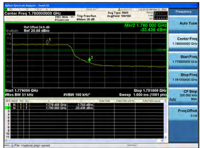
Band66 / 5MHz / High CH / QPSK / FULL RB
