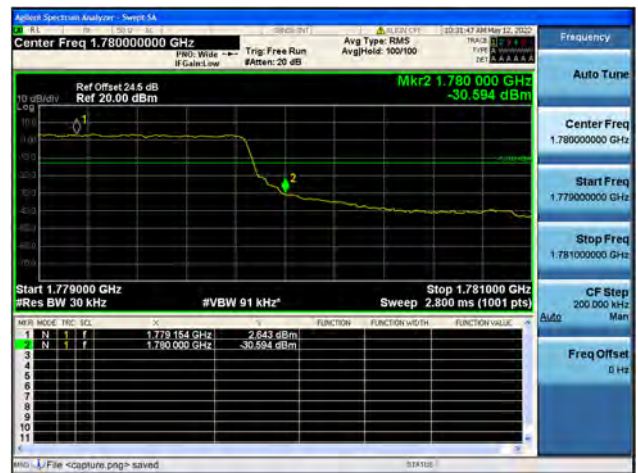
Band66 / 1.4MHz / High CH / QPSK / FULL RB
