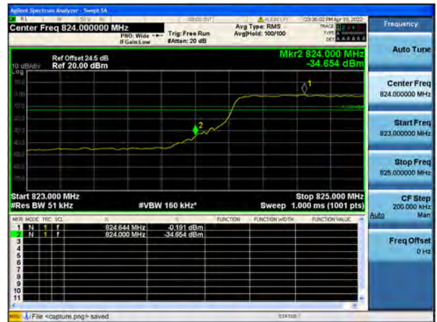
Band5 / 5MHz / High CH / QPSK / FULL RB
