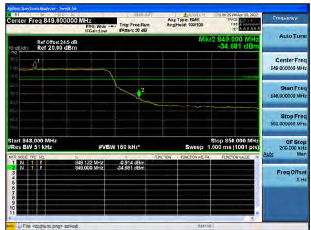
Band5 / 5MHz / High CH / QPSK / FULL RB
