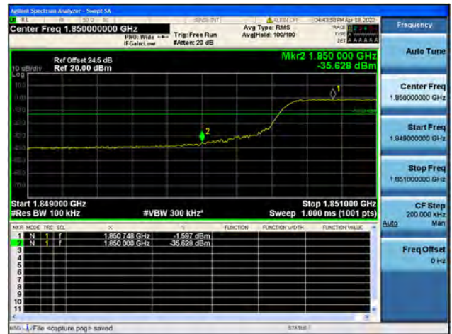
Band2 / 10MHz / High CH / QPSK / FULL RB
