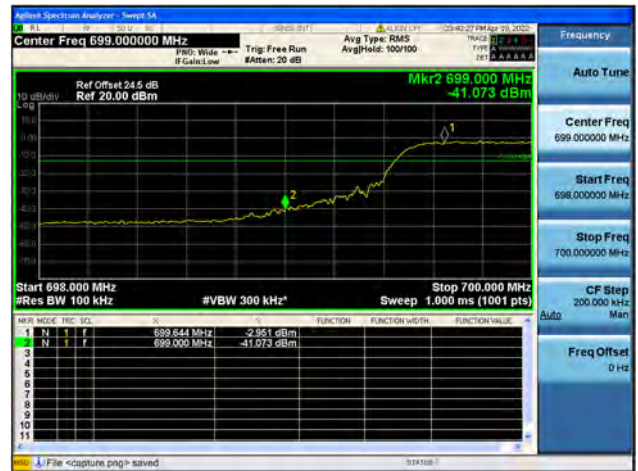
Band12 / 10MHz / High CH / QPSK / FULL RB
