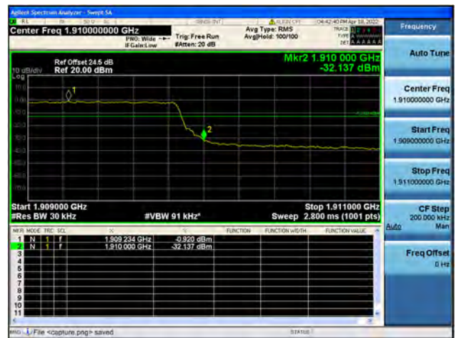
Band2 / 3MHz / High CH / QPSK / FULL RB
