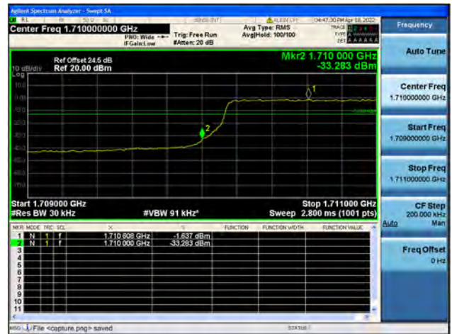
Band4 / 3MHz / High CH / QPSK / FULL RB
