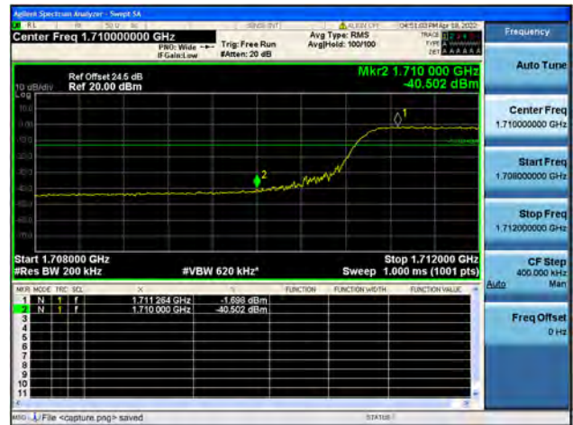
Band4 / 20MHz / High CH / QPSK / FULL RB
