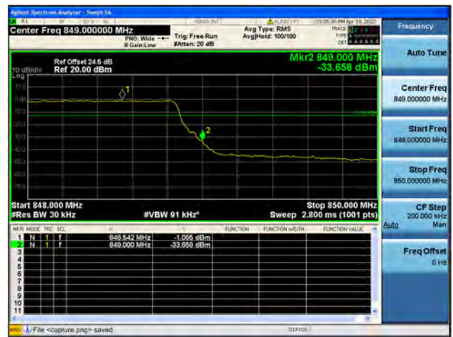
Band5 / 3MHz / High CH / QPSK / FULL RB
