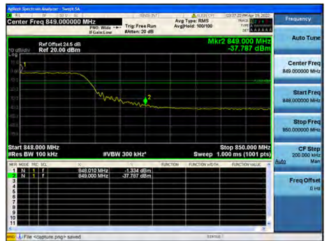
Band5 / 10MHz / High CH / QPSK / FULL RB
