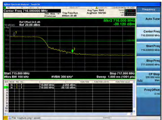
Band12 / 10MHz / High CH / QPSK / FULL RB
