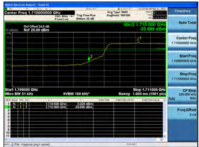
Band66 / 5MHz / High CH / QPSK / FULL RB
