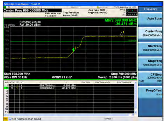
Band12 / 3MHz / High CH / QPSK / FULL RB
