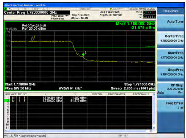
Band66 / 3MHz / High CH / QPSK / FULL RB
