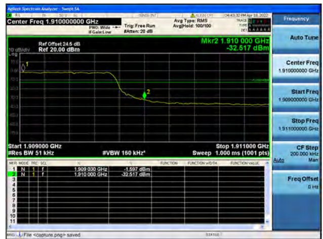
Band2 / 5MHz / High CH / QPSK / FULL RB
