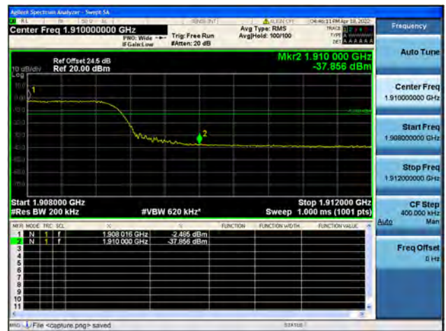
Band2 / 20MHz / High CH / QPSK / FULL RB
