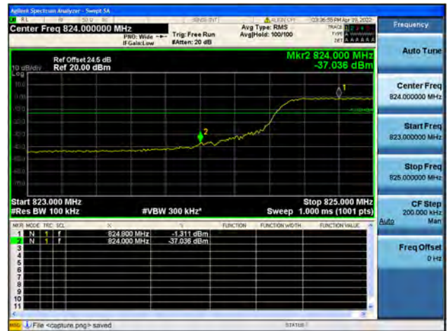
Band5 / 10MHz / High CH / QPSK / FULL RB
