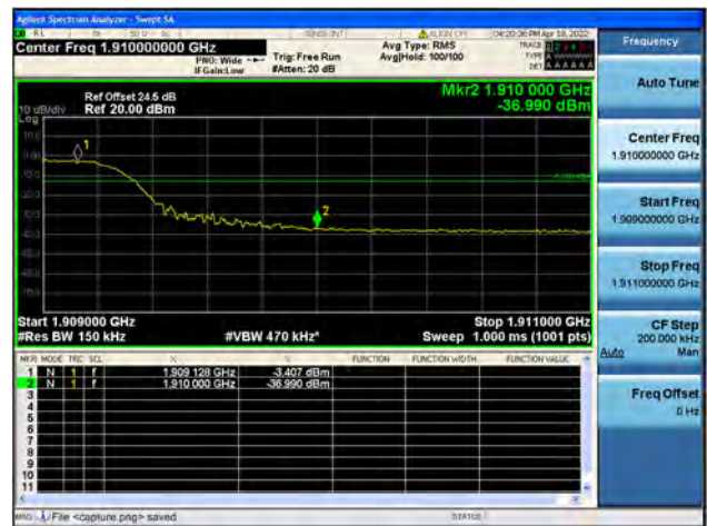
Band2 / 15MHz / High CH / QPSK / FULL RB
