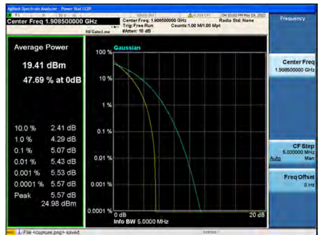
Band2 / 3MHz / High CH / 64QAM
