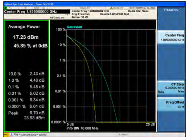
Band25 / 10MHz / Low CH / 64QAM
