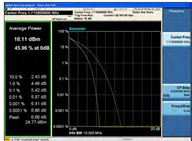
Band66 / 10MHz / Low CH / 64QAM
