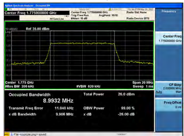
Band66 / 10MHz / High CH / 64QAM
