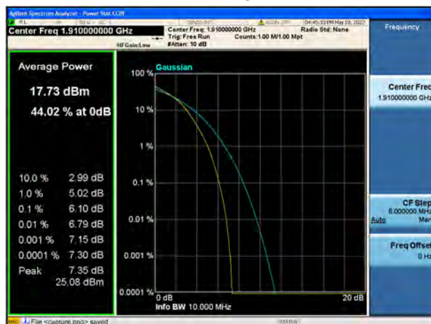
Band25 / 10MHz / High CH / 16QAM
