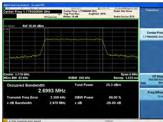
Band66 / 3MHz / High CH / 16QAM
