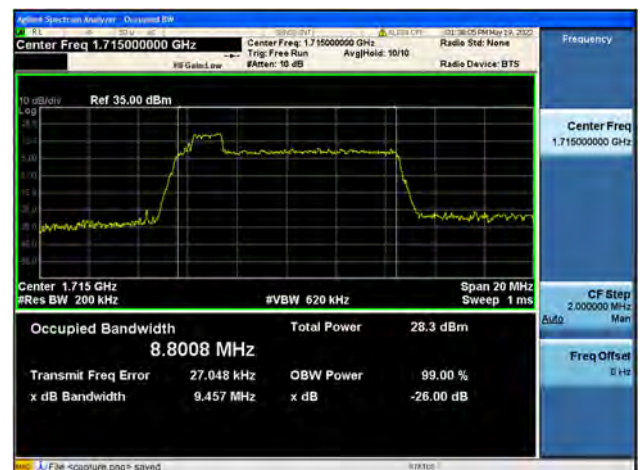
Band66 / 10MHz / Low CH / 64QAM
