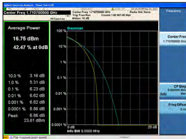
Band4 / 1.4MHz / Mid CH / 16QAM
