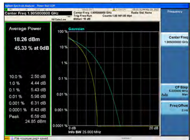
Band25 / 20MHz / High CH / 64QAM
