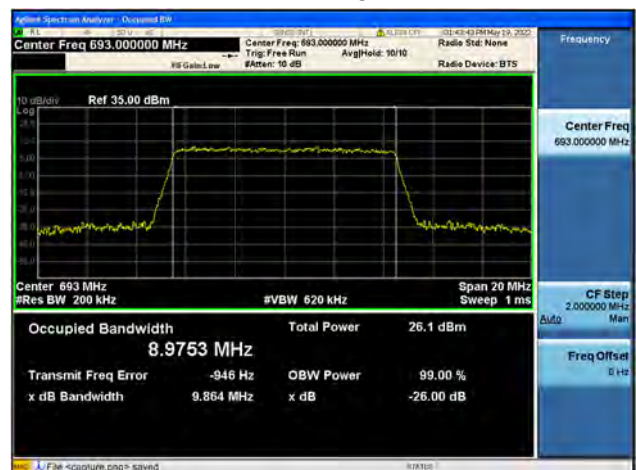
Band71 / 10MHz / High CH / 64QAM
