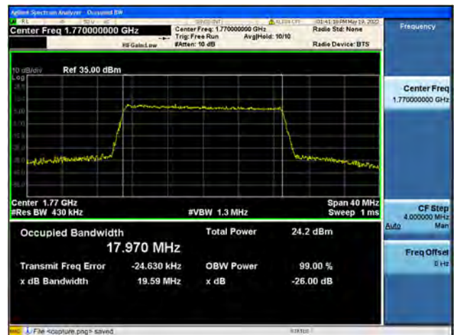
Band66 / 20MHz / High CH / 64QAM
