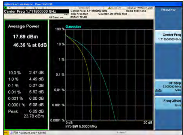
Band66 / 3MHz / Low CH / 64QAM
