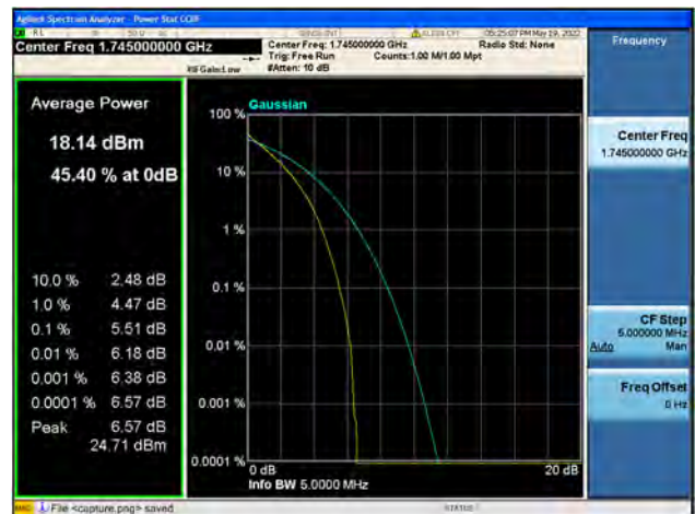
Band66 / 5MHz / Mid CH / 64QAM
