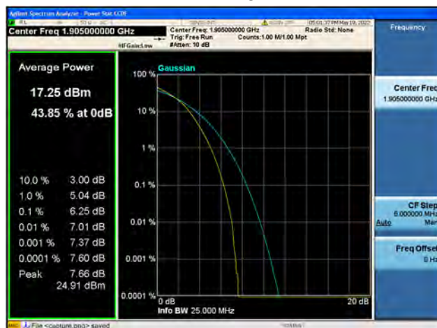
Band25 / 20MHz / High CH / 16QAM
