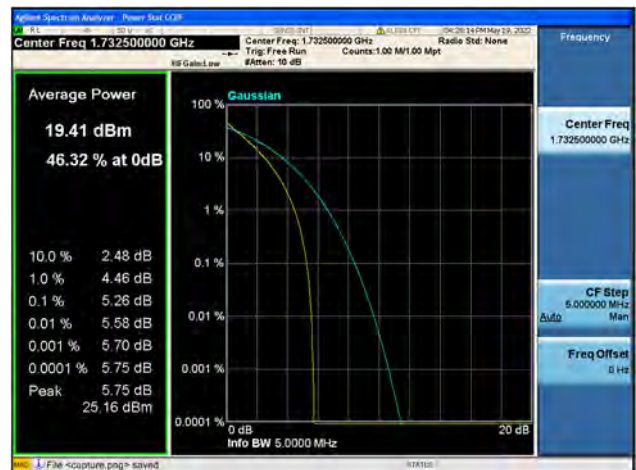
Band4 / 3MHz / Mid CH / QPSK
