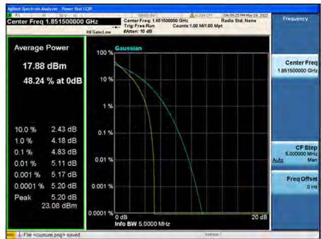
Band2 / 3MHz / Low CH / 64QAM
