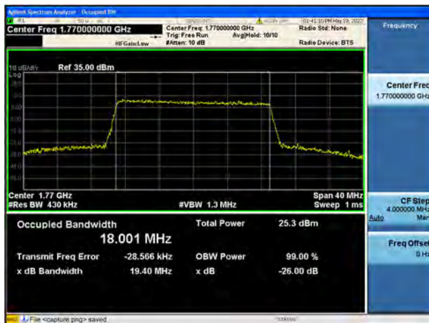
Band66 / 20MHz / High CH / 16QAM
