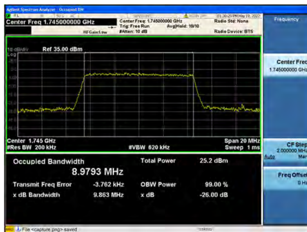
Band66 / 10MHz / High CH / 16QAM
