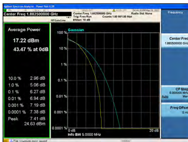
Band25 / 5MHz / Mid CH / 16QAM
