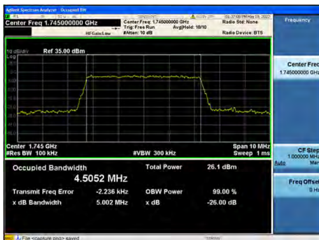
Band66 / 5MHz / Mid CH / 16QAM
