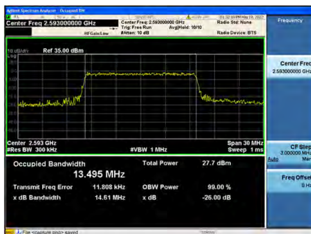
Band41 / 15MHz / Mid CH / 16QAM
