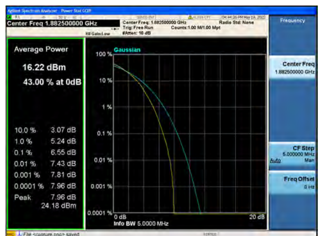
Band25 / 5MHz / Mid CH / 64QAM
