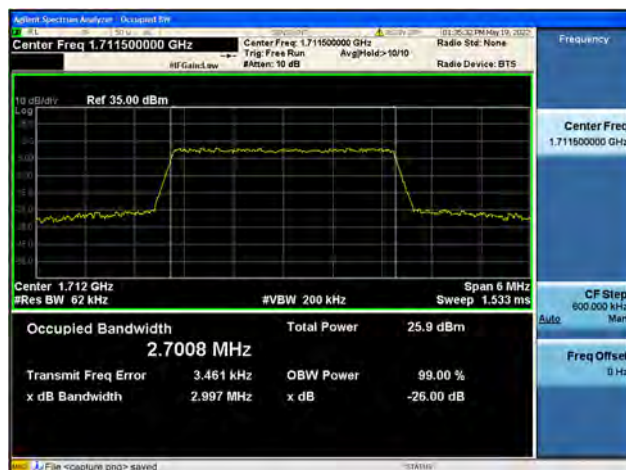
Band66 / 3MHz / Low CH / 16QAM
