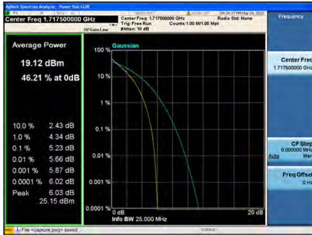
Band4 / 15MHz / Low CH / 64QAM
