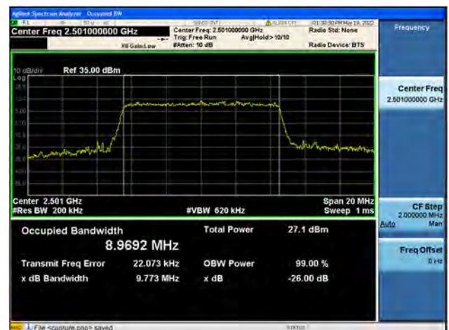
Band41 / 10MHz / Low CH / 64QAM
