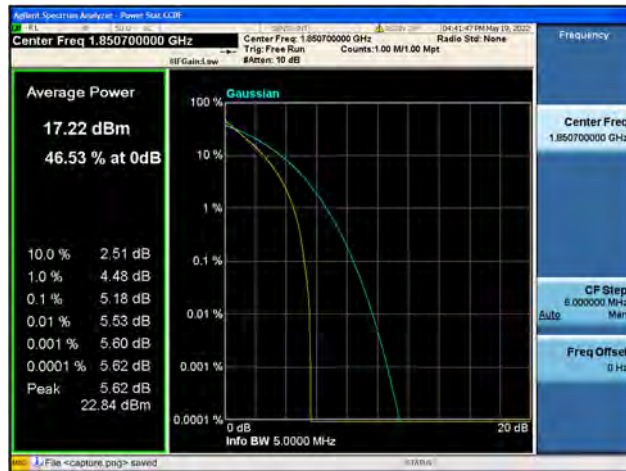
Band25 / 1.4MHz / Low CH / 64QAM
