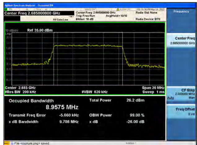
Band41 / 10MHz / High CH / 64QAM
