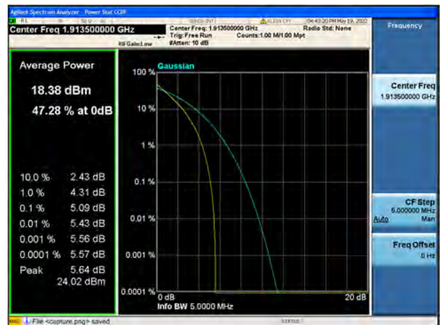
Band25 / 3MHz / High CH / 64QAM
