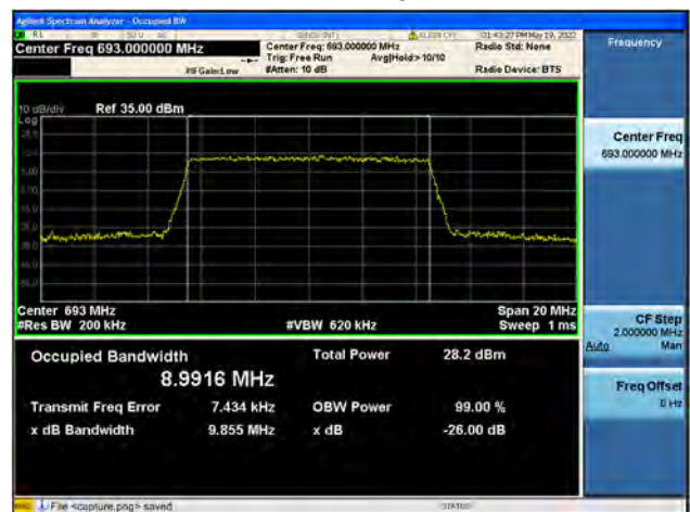
Band71 / 10MHz / High CH / 64QAM
