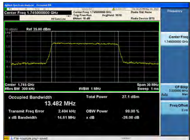
Band66 / 15MHz / Mid CH / 64QAM
