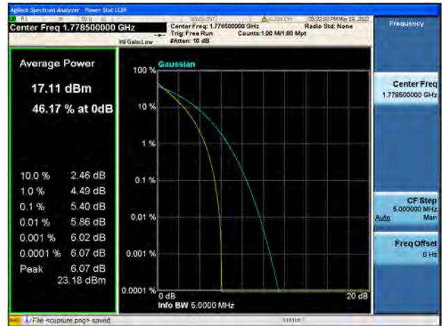
Band66 / 3MHz / High CH / 64QAM
