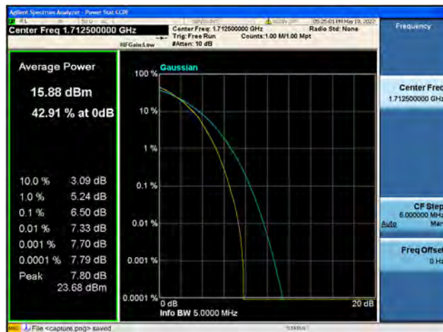
Band66 / 5MHz / Mid CH / 16QAM
