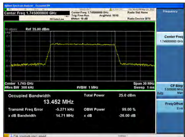
Band66 / 15MHz / Mid CH / 64QAM
