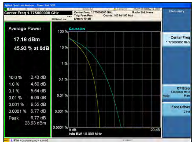
Band66 / 10MHz / High CH / 64QAM
