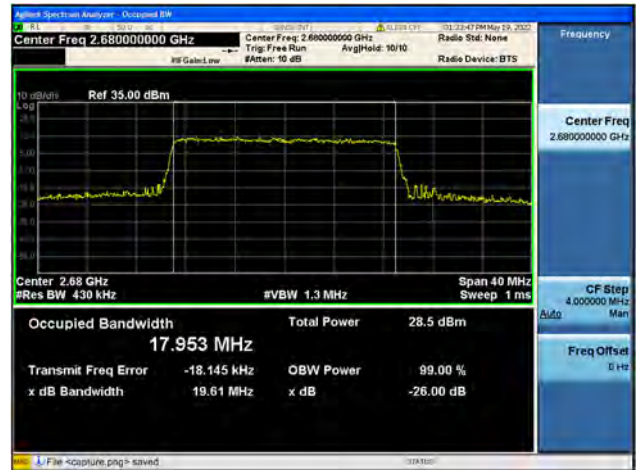
Band41 / 20MHz / High CH / 64QAM
