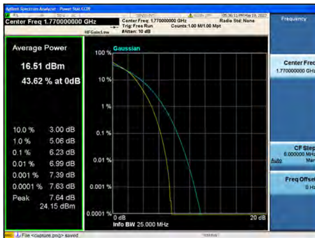
Band66 / 20MHz / High CH / 16QAM
