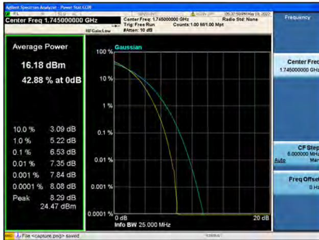
Band66 / 20MHz / High CH / 16QAM
