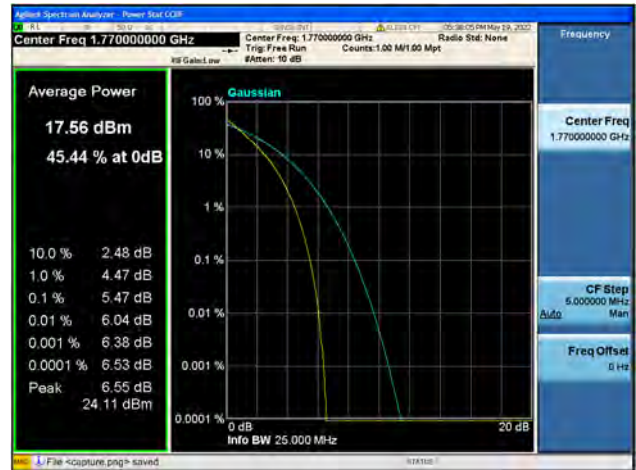
Band66 / 20MHz / High CH / 64QAM
