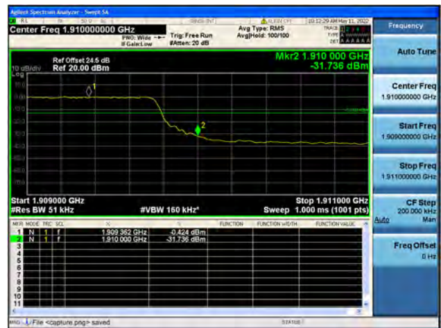
Band2 / 5MHz / High CH / QPSK / FULL RB
