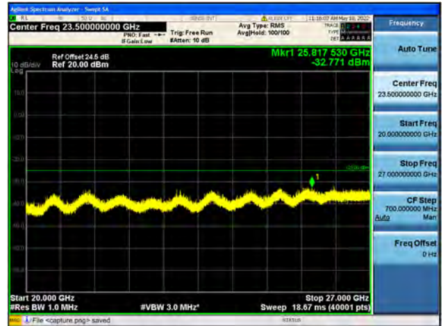
Band41-20G-27G / 10MHz / High CH / 16QAM
