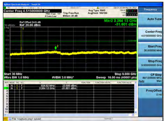
Band26 / 3MHz / Low CH / 64QAM
