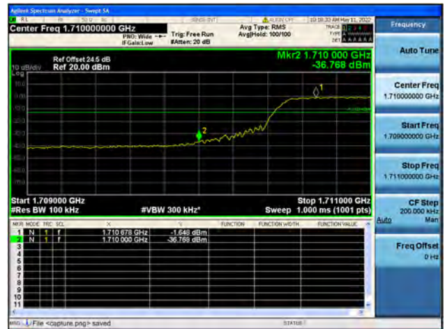
Band4 / 10MHz / High CH / QPSK / FULL RB
