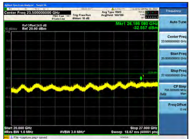
Band41-20G-27G / 15MHz / High CH / 64QAM
