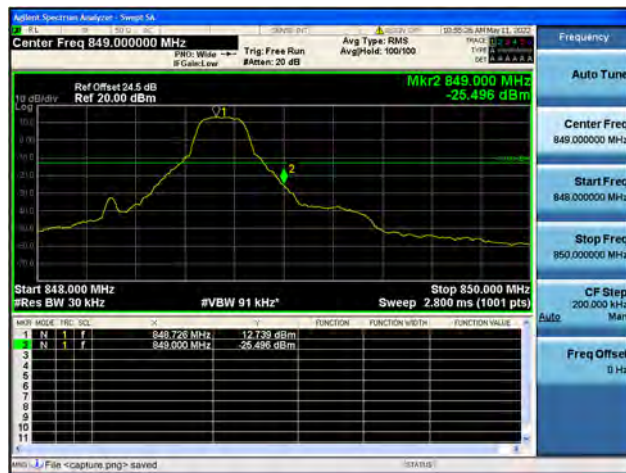
Band5 / 1.4MHz / High CH / QPSK / 1 RB
