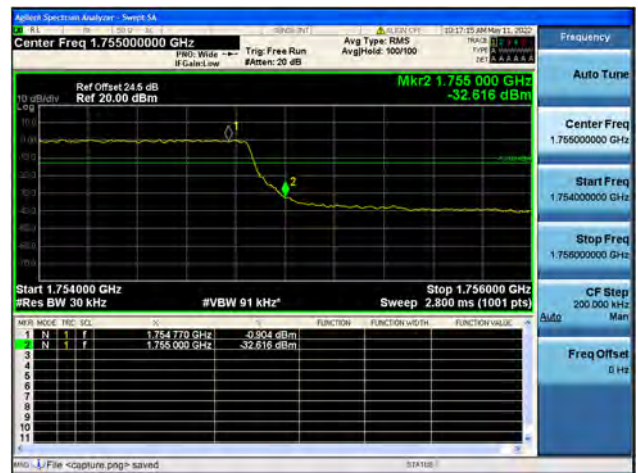
Band4 / 3MHz / High CH / QPSK / FULL RB
