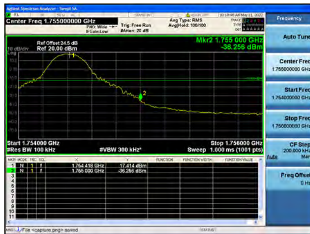
Band4 / 10MHz / High CH / QPSK / 1 RB
