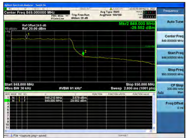
Band5 / 1.4MHz / High CH / QPSK / FULL RB
