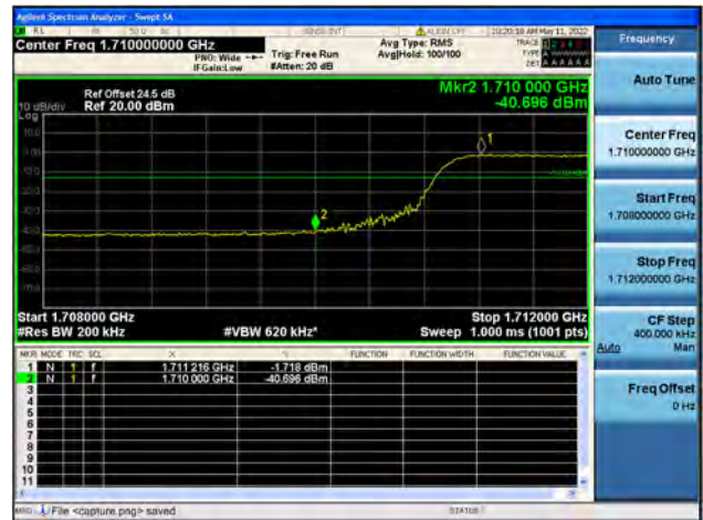
Band4 / 20MHz / High CH / QPSK / FULL RB
