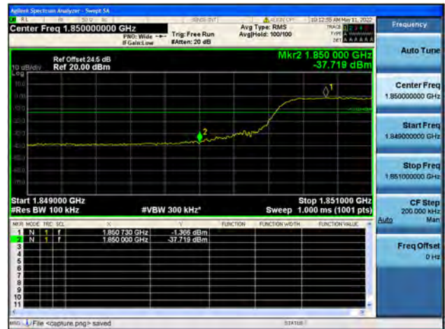
Band2 / 10MHz / High CH / QPSK / FULL RB
