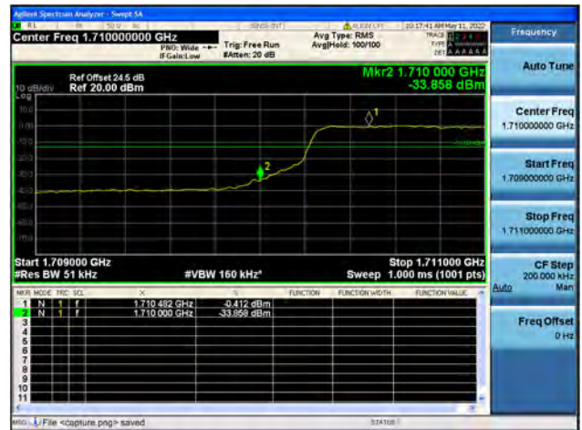
Band4 / 5MHz / High CH / QPSK / FULL RB
