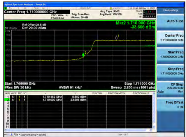
Band4 / 3MHz / High CH / QPSK / FULL RB
