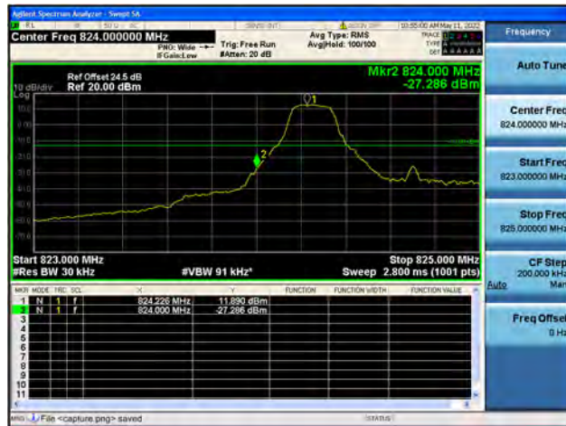
Band5 / 1.4MHz / High CH / QPSK / 1 RB
