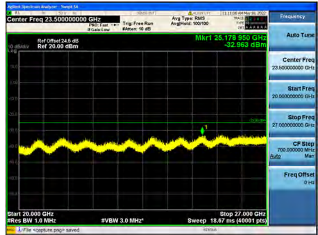
Band41-20G-27G / 5MHz / High CH / 16QAM
