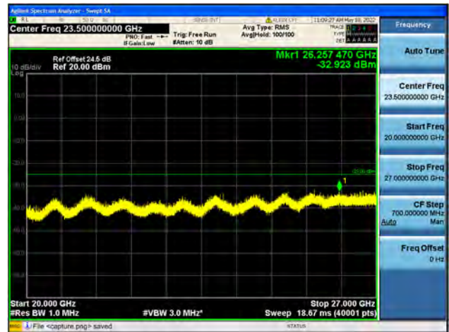
Band41-20G-27G / 5MHz / Mid CH / 16QAM
