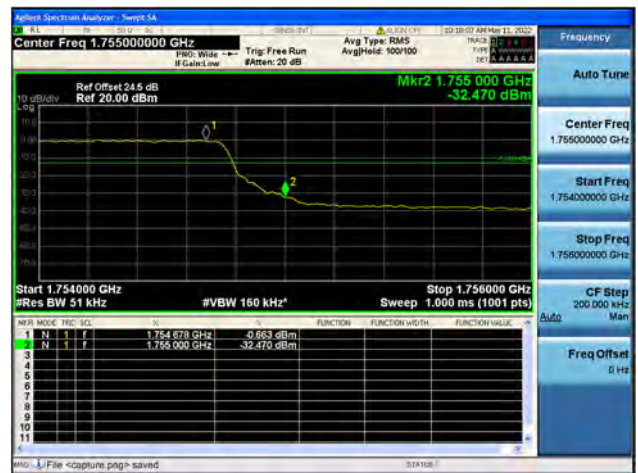
Band4 / 5MHz / High CH / QPSK / FULL RB
