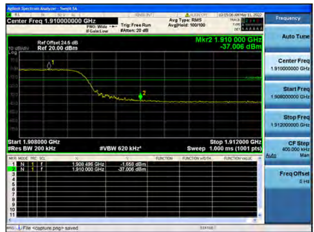
Band2 / 20MHz / High CH / QPSK / FULL RB
