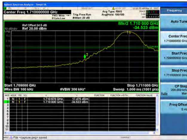
Band4 / 10MHz / High CH / QPSK / 1 RB
