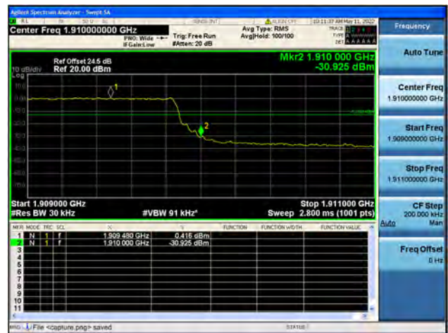
Band2 / 3MHz / High CH / QPSK / FULL RB
