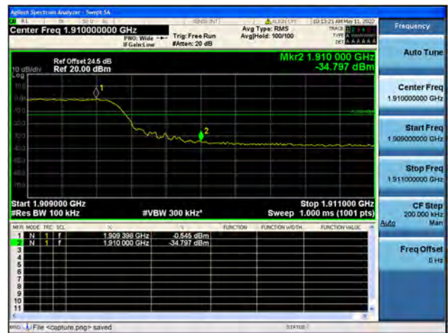
Band2 / 10MHz / High CH / QPSK / FULL RB
