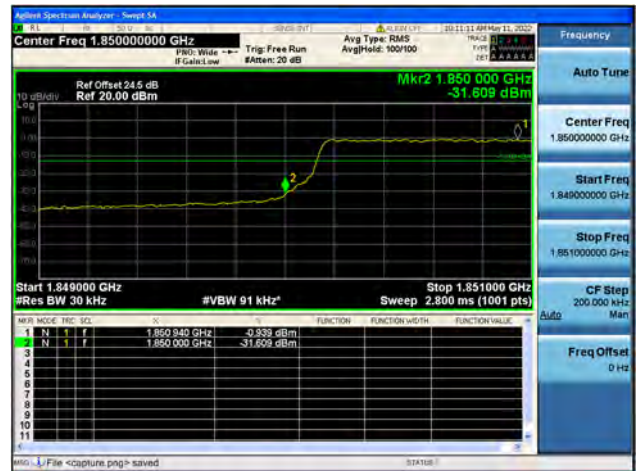
Band2 / 3MHz / High CH / QPSK / FULL RB
