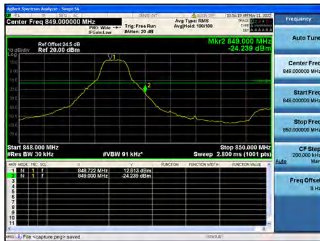
Band5 / 3MHz / High CH / QPSK / 1 RB
