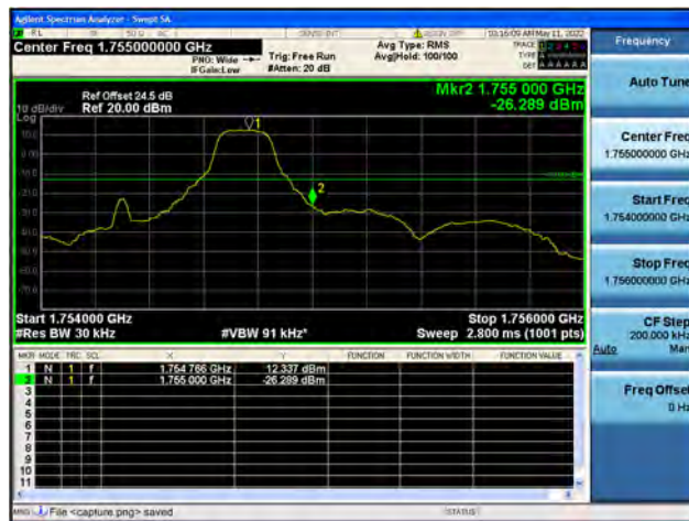
Band4 / 1.4MHz / High CH / QPSK / 1 RB
