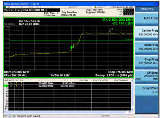
Band5 / 1.4MHz / High CH / QPSK / FULL RB
