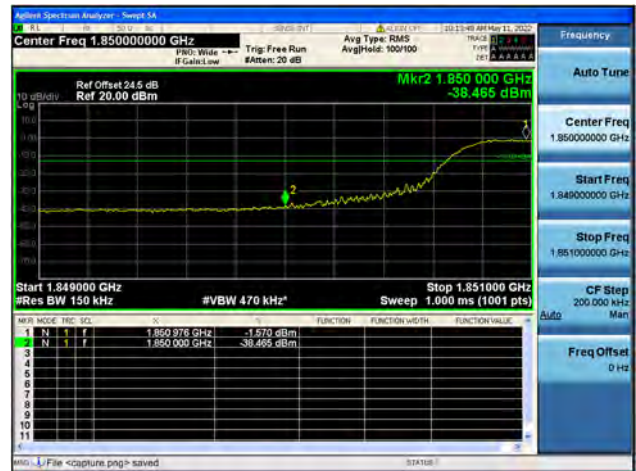
Band2 / 15MHz / High CH / QPSK / FULL RB
