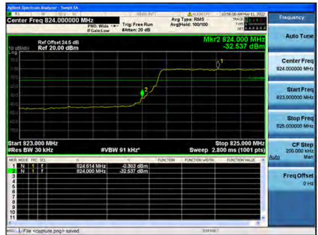
Band5 / 3MHz / High CH / QPSK / FULL RB
