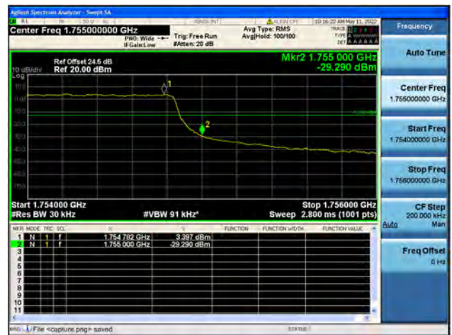
Band4 / 1.4MHz / High CH / QPSK / FULL RB
