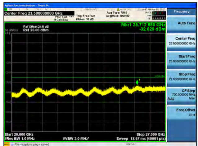
Band41-20G-27G / 10MHz / High CH / 64QAM
