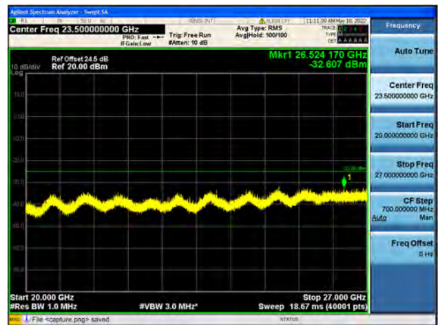
Band41-20G-27G / 5MHz / High CH / 64QAM
