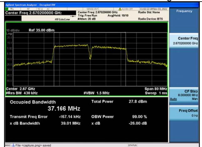
Band41C / 20MHz+20MHz / 64QAM/ High CH
