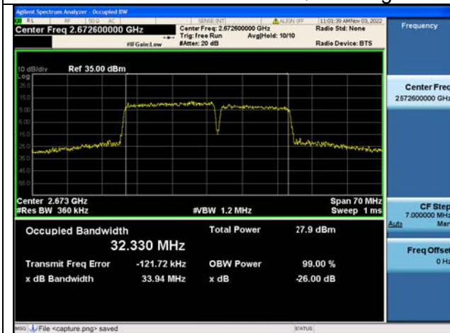
Band41C / 20MHz+15MHz / 64QAM/ High CH
