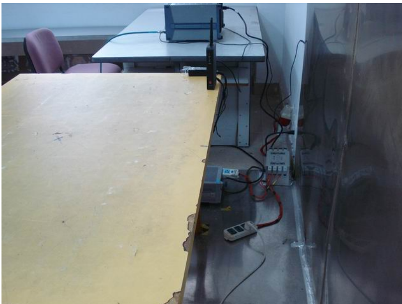
Conducted Emissions Test Setup – Side View
