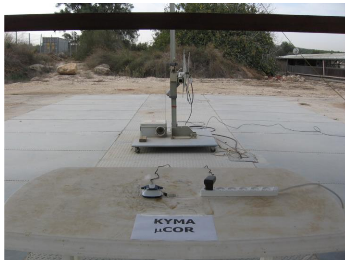
Figure 10. Radiated Emission Test in Charging Mode
