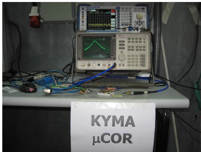
Figure 4. Conducted Emission from Antenna Port Test
