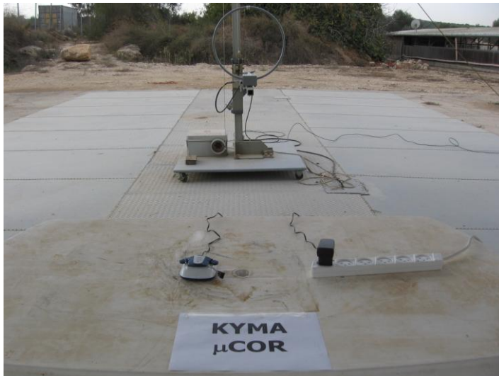
Figure 12. Radiated Emission Test in Charging Mode
