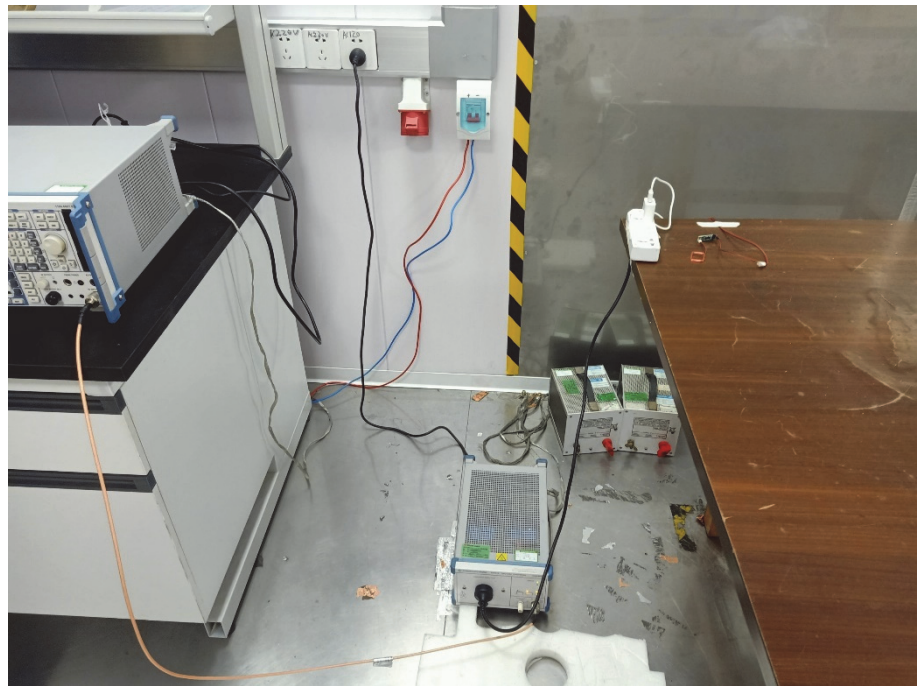
Conducted Emission Test Setup
