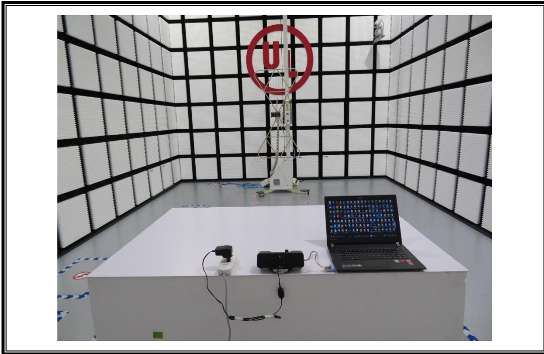
RADIATED RF MEASUREMENT SETUP (30MHz ~ 1 GHz)
