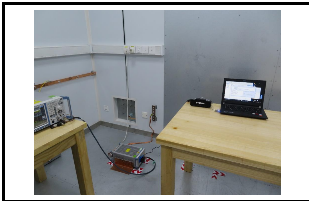
POWERLINE CONDUCTED EMISSIONS MEASUREMENT SETUP
