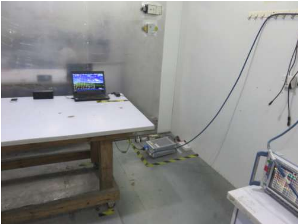
FCC RADIATED EMISSION TEST SETUP
