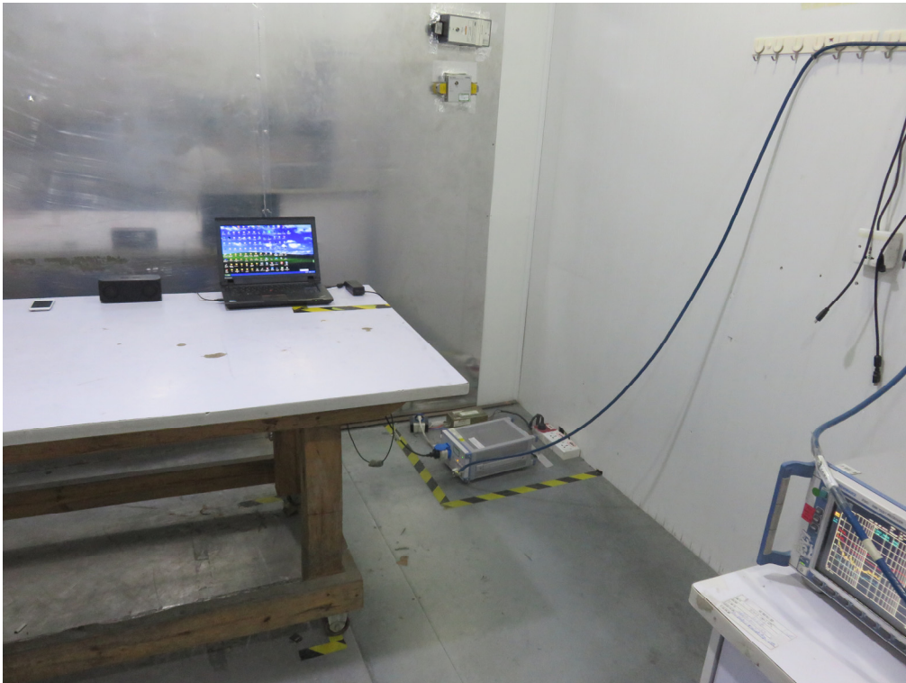
FCC RADIATED EMISSION TEST SETUP
