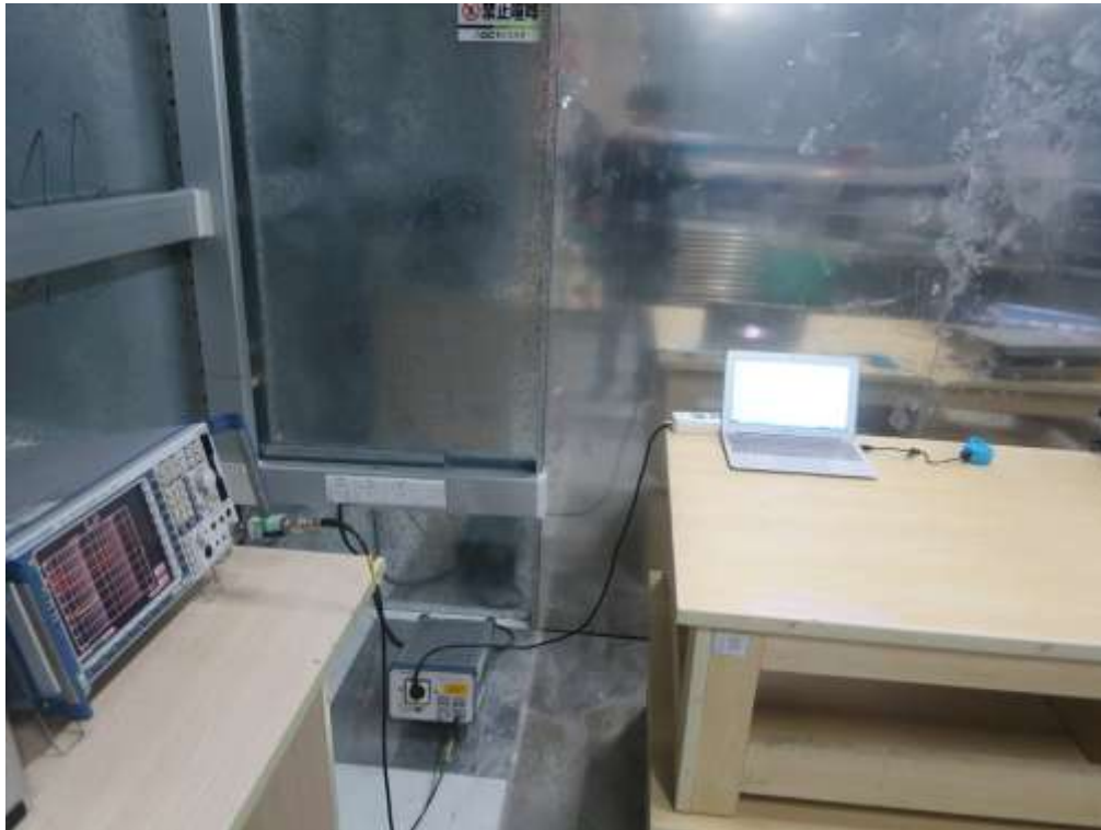
FCC RADIATED EMISSION TEST SETUP
