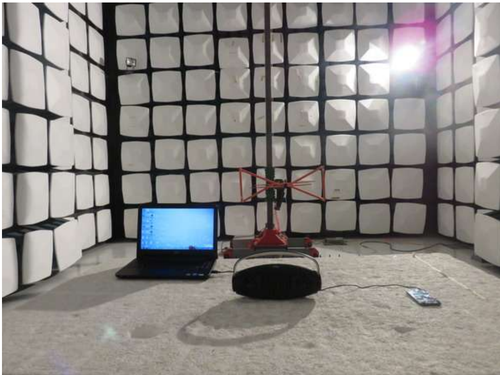
FCC RADIATED EMISSION TEST SETUP
