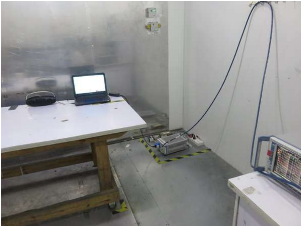
FCC RADIATED EMISSION TEST SETUP
