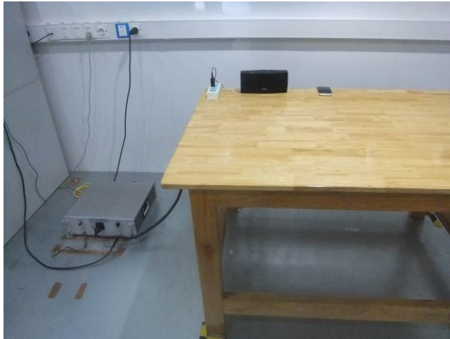
Conducted Emissions Test Setup Front View
