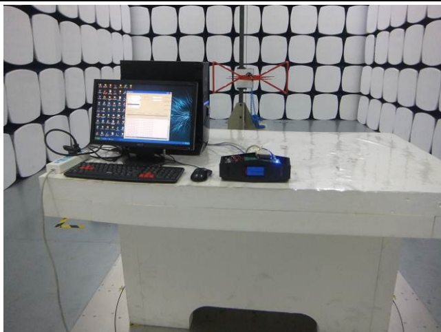
Radiated Spurious Emissions Test Setup Below 1GHz
