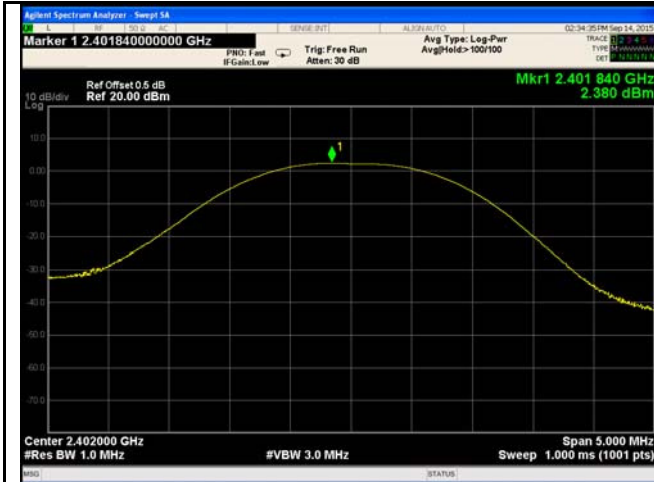
GFSK Output power - Low CH 2402
